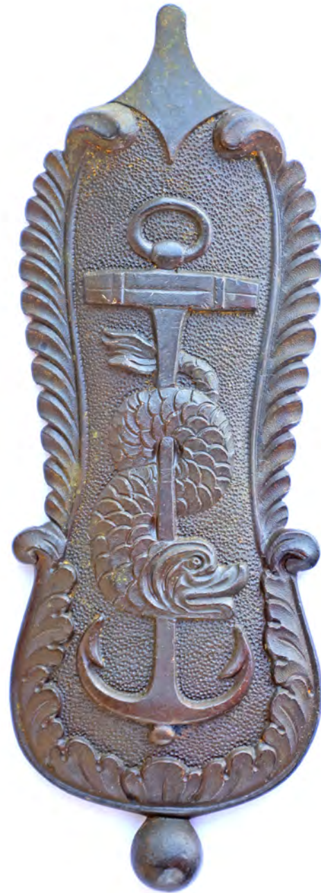
Figure 15. Pattern used to manufacture the drag for Congressional Swords.
