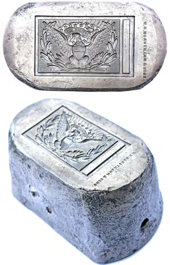
Figure 13. Die used to produce the M1851 regulation eagle buckles for William H Horstmann & Sons.
