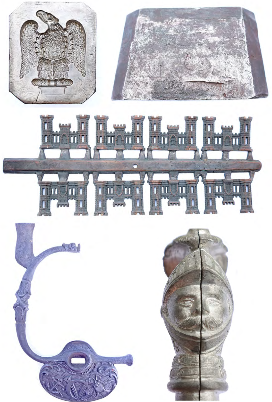
Figure 7. Examples of Stamping Die (top) and various Casting Patterns (bottom).
