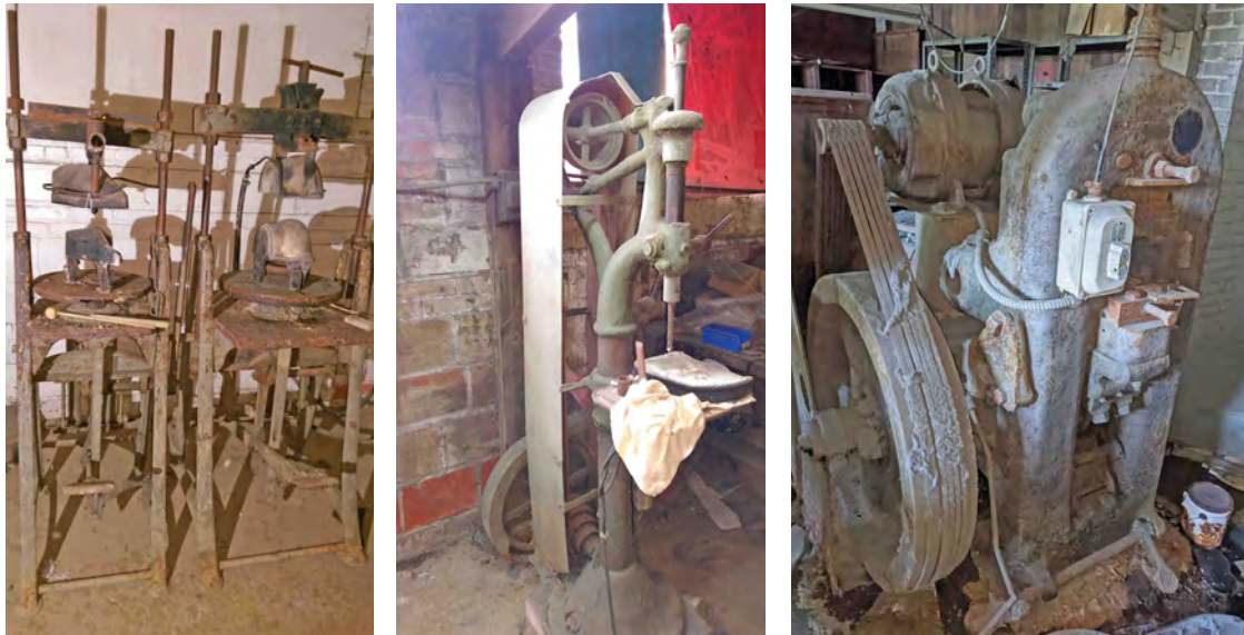
Figure 4. Hat forming machine, drill press and Ferracute coining press.
