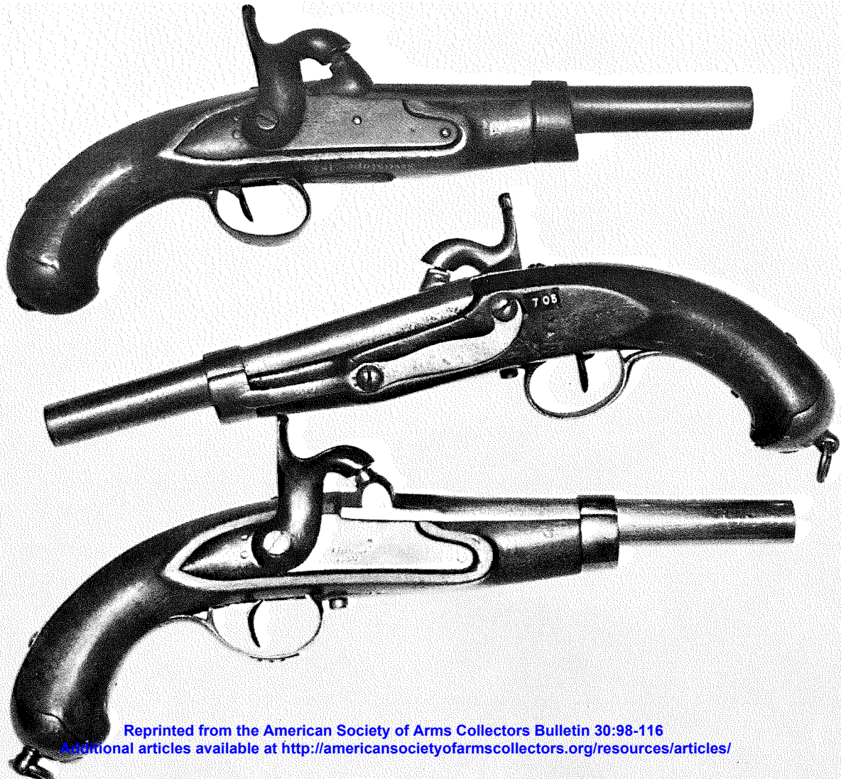
Figure 26. Piedmont M 1829 converted. Lower is original percussion.
