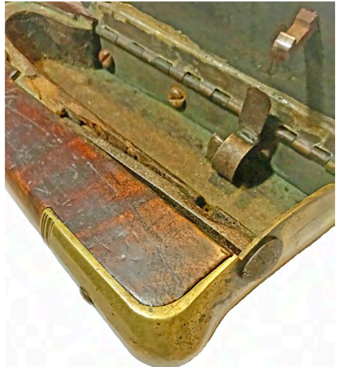
Figure 15. The coil spring which opens the lid of the box is of the same design as springs used to operate door locks.
