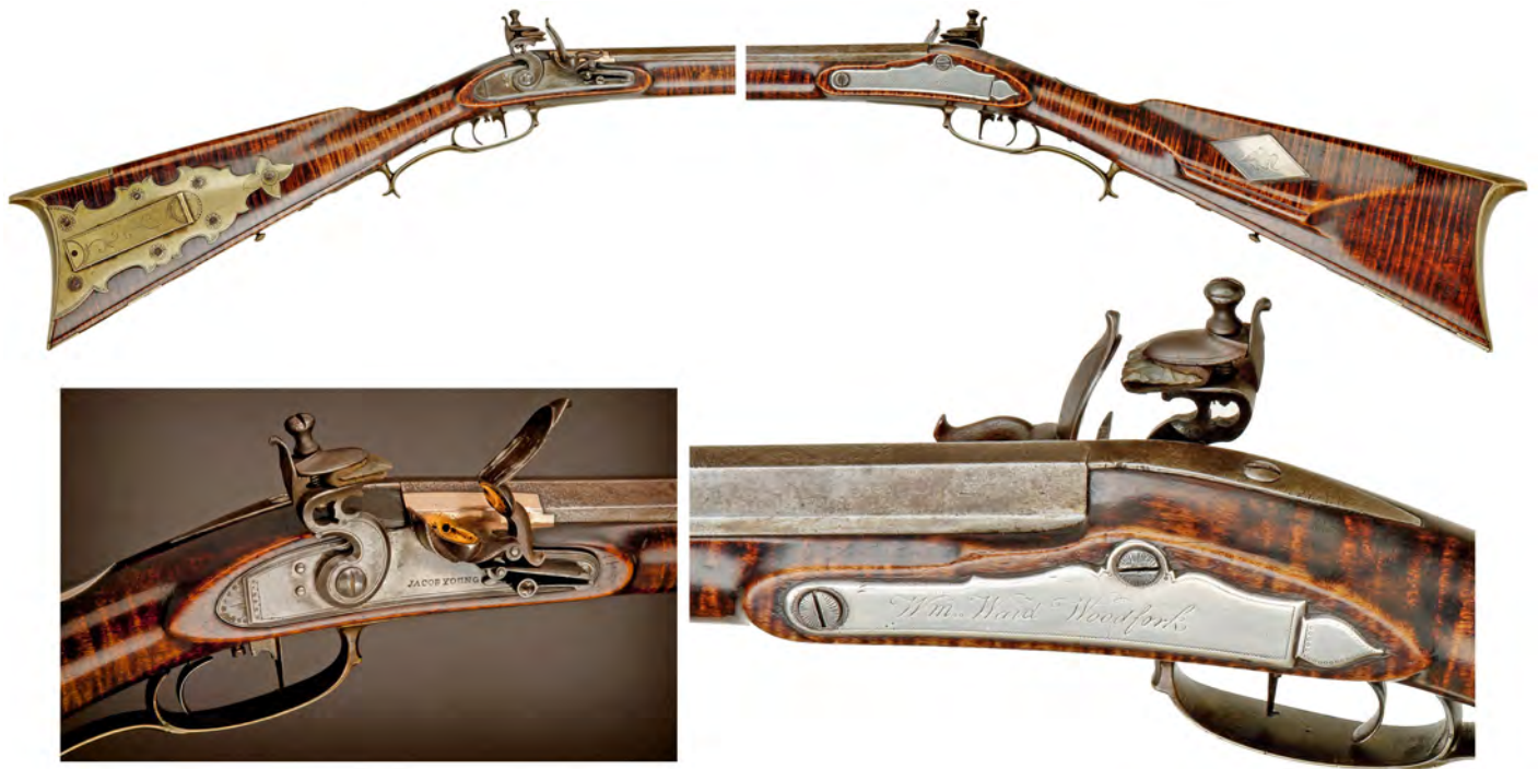
Figure 2. Jacob Young made this rifle for Wm. Waid Woodfork and elegantly engraved his name on the silver sideplate. Its unique patchbox was fashioned from a single piece of cast brass and fitted with a captured lid. The rifle is built around a handmade flintlock signed by Jacob Young - notice the gold lined flash pan and flash guard inlaid into the barrel. The cheekpiece holds the largest of a dozen coin silver inlays: a large, elongated diamond decorated with a Federal eagle.
