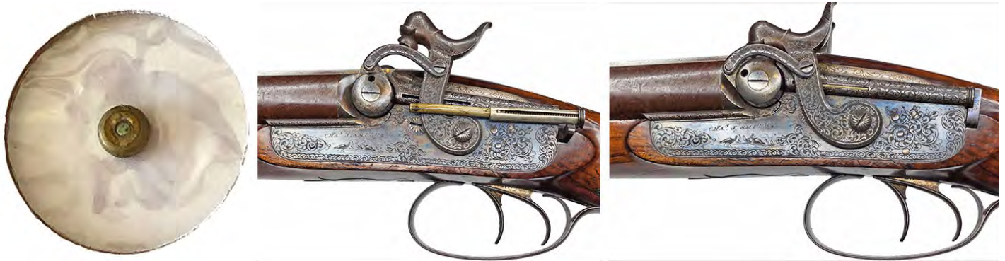
Figure 17. The Charles James Smith pellet primer (left, photo by Jas van Driel). The C.J. Smith double gun (center, photo by Fred Bienvenu). The magazine taken apart; the action ready to receive the pellet primer. The magazine together (right). The action rotated and the primer detonated.
