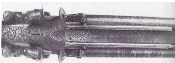
Figure 15. The tube magazine version of Joseph Egg's system, placed next to the central rib between the barrels (see reference 14, page 70).
