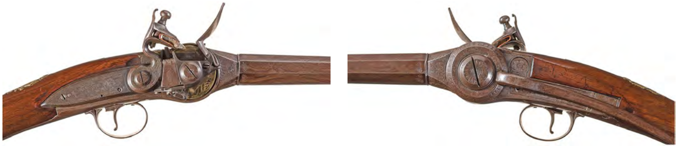
Figure 4. Lorenzoni system gun by William 1 Wilson, London, the 1770s. The closed priming powder magazine in front of the cock, and one of the axis screws for the large brass cylindrical action (left). The door for the ball and gunpowder magazines is behind the long action-rotating lever (right). Photos courtesy of Rock Island Auction.
