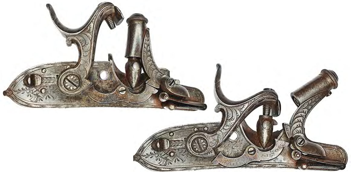
Figure 11. The Westley Richards patent lock. The hammer cocked, the priming powder magazine on the pan. The linking arm between hammer and magazine is screwed onto the front of the lock plate. As the hammer falls, the magazine is pushed up and away, leaving the primed pan open. Photos by Fred Bienvenu.
