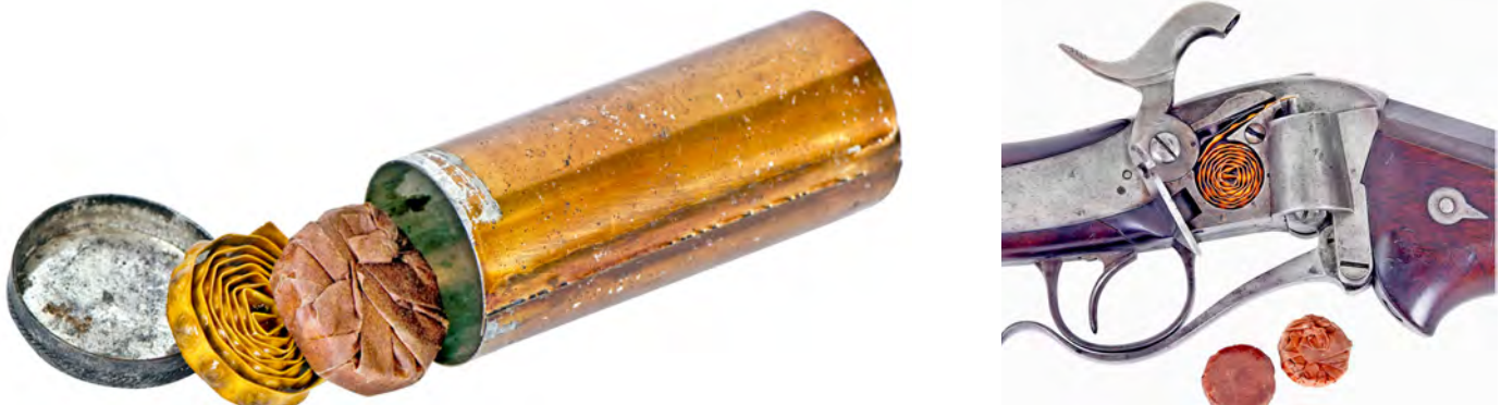
Figure 18. Maynard tape primer rolls, unwrapped and wrapped, and their container. The tape primer roll in its magazine, with the end fulminate bubble over the nipple. The magazine door of a model 1850 Sharps is open. Photo by Ron Paxton.
