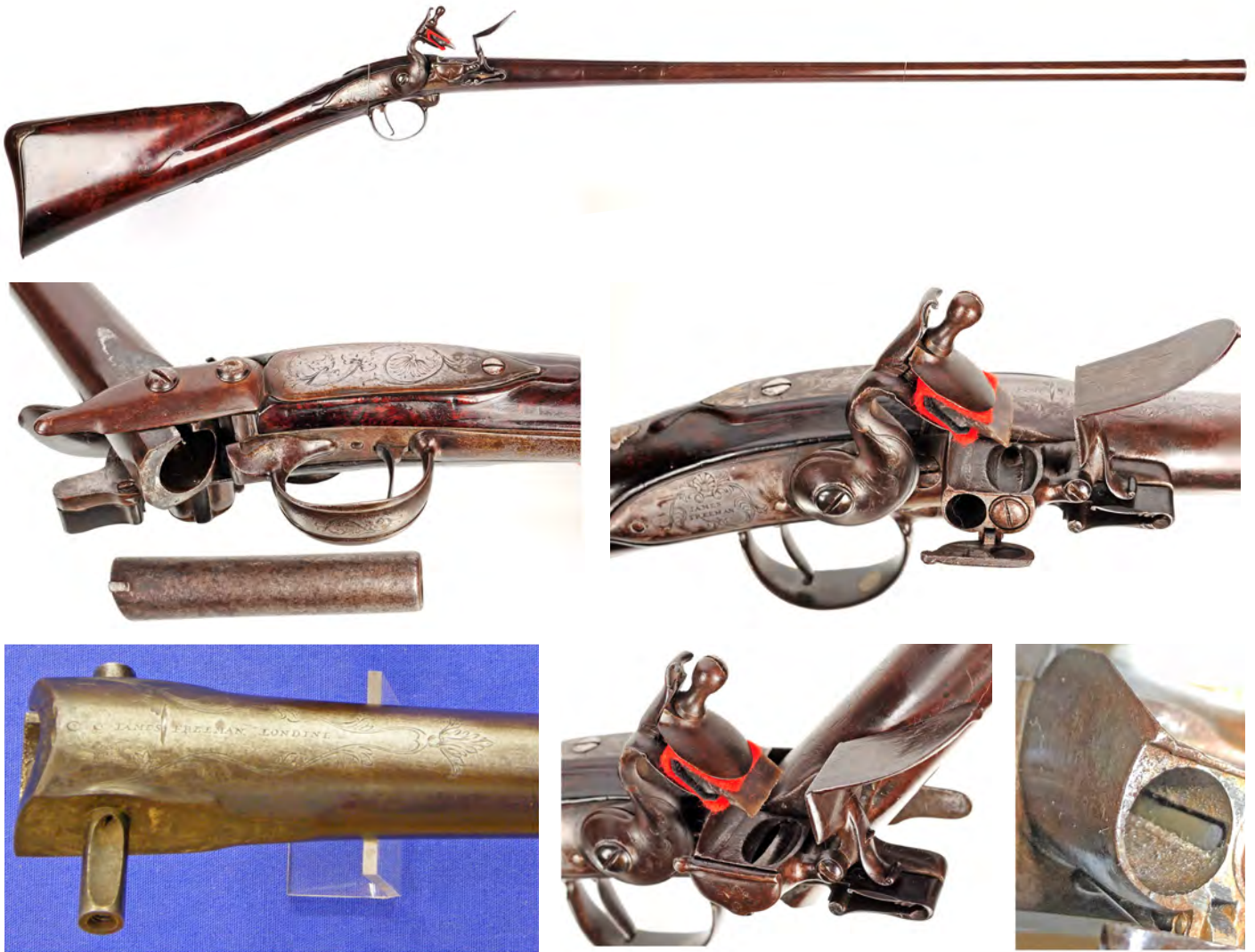
Figure 3. The Freeman gun (top). The gun's barrel released and lifted upward, and the cartridge removed (upper left, photo by Dan Retting). The protrusion at the left edge of the cartridge fits the slot in the breech for indexing. The powder magazine with its gate open (upper right). The floor of the pan is attached to the barrel, not the lock. (blue background, photo courtesy of Ton Bolk). As the barrel is raised, the floor of the pan drops down in front of the magazine (photo by Dan Retting). The opening in the forward wall of the magazine through which priming powder flows when the magazine is tilted downward (bottom, photo by Matthew Schneiderman).
