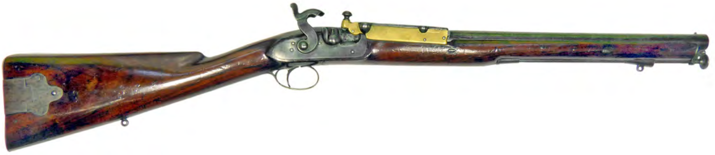
Figure 16. Westley Richard's patent brass cap magazine. At the far left, the "thumbpiece" that's pressed down to place the cap on the nipple. Photo by Brian Godwin, courtesy of the Bob Freeman Collection.
