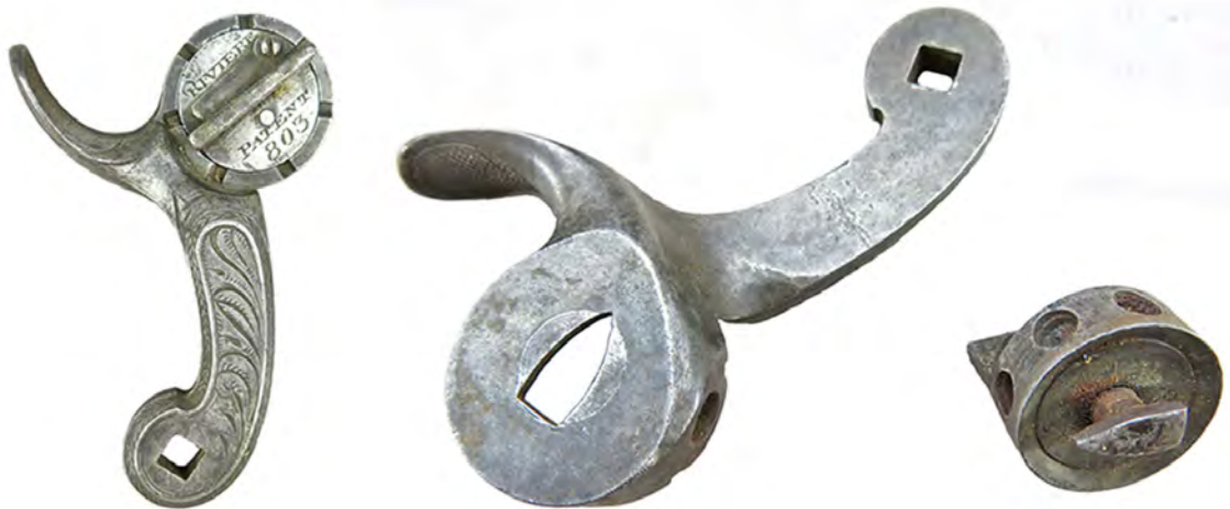
Figure 12. The Isaac Riviere hammer magazine. A raised handle for turning or removing the wheel and notches around the edge for indexing (left). The magazine wheel removed, showing the spaces for the sticky pills (right). At the lower border of the hammer head, the opening that allows the nipple to detonate the pill. Photos courtesy of Thomas Del Mar auctions.
