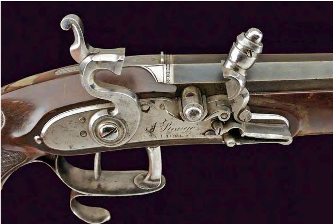
Figure 10. A very early fulminate-powder-detonated pistol by Ronge, Liege. What looks like a magazine is a big firing pin and its housing. It's moved onto the pan (pointing toward 10 o'clock) and then flipped back up, both by hand. Photo courtesy of Czerny's Auctions.
