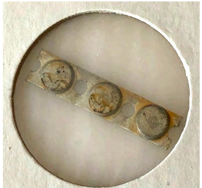
Figure 20. A piece from an Edward Savoral 1876 metal tape primer roll. Photo by Matthew Schneiderman.
