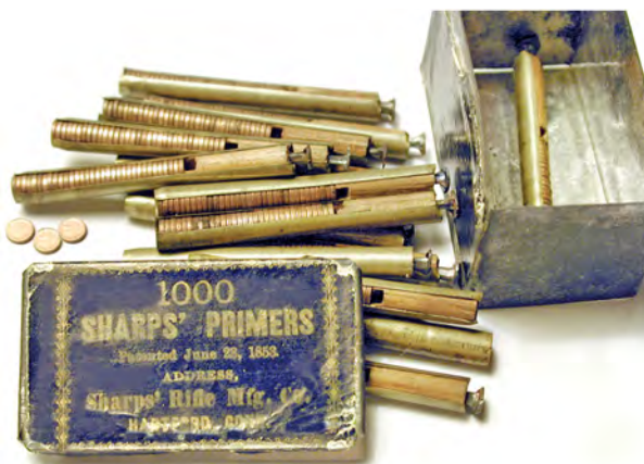
Figure 21. Sharps copper disc primers in their "chargers". The wooden piece is for pushing the stack of primers into the magazine. The metal at the top makes it easier to push down (photo by Ron Paxton). A drawing from the Sharps patent #9308. To the left is the magazine with its spring and a stack of primers in place.
