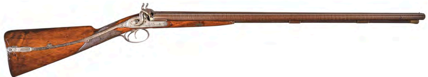
Figure 23. The William Needham double gun, with the long cap magazine sweeping down from the rear of the lock to the butt. Photo courtesy of Rock Island Auction.
