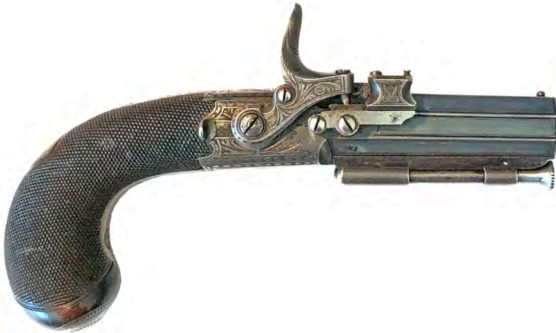
Figure 9. A third model Forsyth sliding-primer pocket pistol. Photo by Matthew Schneiderman.
