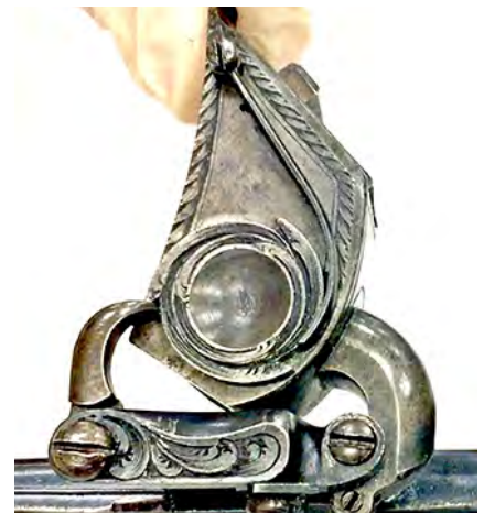
Figure 6. Collier #89. The lever arm and the cylinder axis screw (top left, photo by Frank Graves). The magazine frizzen of the Constable flintlock pepperbox, showing its gear system (top right, photo by Ben Nicholson, courtesy of Jonathan Tavares and the Art Institute of Chicago). A drawing of the first-model Collier magazine frizzen, side view, from the Collier patent (lower left). From the top: loading cover; space for priming powder; internal cylinder with three troughs; pan. A first-model Collier magazine frizzen, side view (bottom right, photo by Ben Nicholson). This one has three priming-powder troughs on its internal cylinder. When the frizzen is pushed down, the fixed spur catches one of the three raised teeth on the side and rotates the cylinder 120 degrees, dumping powder from one of the troughs.
