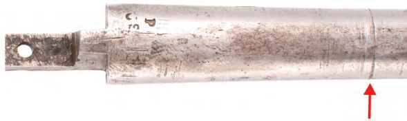
Figure 30. Bottom side of an iron banded example with numbered 47 on the breech and barrel, suggesting it was originally made to be a pin fastened barrel (in general, iron banded examples are not numbered). Note the lathe marks and the deeper score on the bottom of the barrel only (red arrow) that corresponds to placement of the retaining pin with pin fastened barrels. It is believed this was used to position placement of the loop on the bottom of the barrel through which the retaining pin passed.
