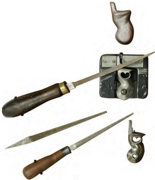
Figure 2. Filing jig for hammer used in an effort to provide some uniformity of parts.
