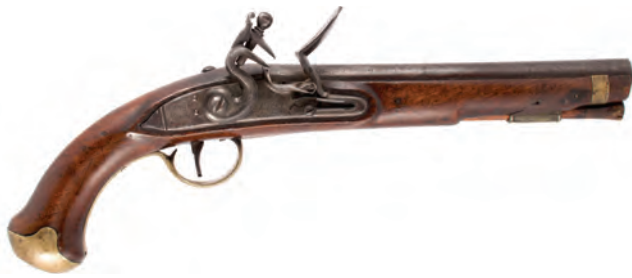
Figure 10. 1797 assembled horseman's pistol. Note the brass band at the end of the fore stock to prevent splitting.
