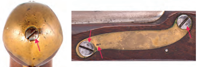
Figure 24. Assembly marks on the butt cap screw head, heads of the lock plate retaining screws and side plate.
