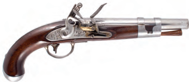
Figure 40. Example of a flat lock 1813 pistol, note the iron accessories with the flat lock of the 1811 pistol. The barrel was also in the configuration of an 1811 pistol as it lacked the facets at the breech.
