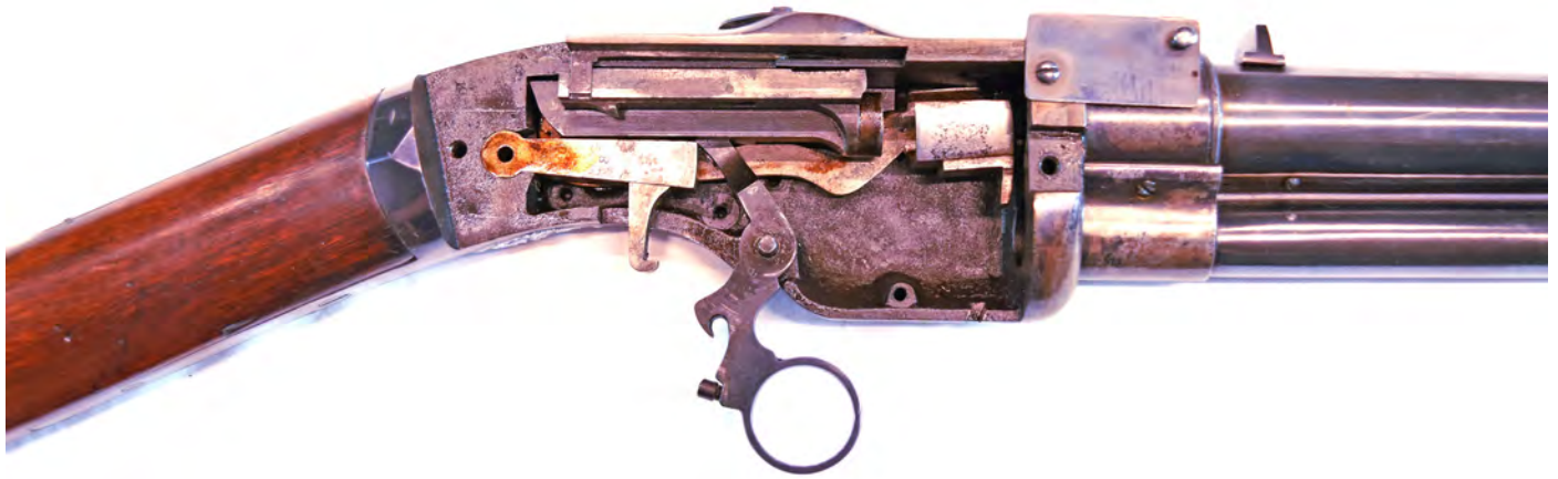
Figure 9. Smith-Jennings Interior: Action view of a 2 nd Model Smith-Jennings rifle, serial No. 8. Visible from left to right are: the locking wedge or block, the bolt (note the thin arm that rides with the bolt and interfaces with the priming magazine), the ring lever that acts on the bolt and locking wedge and the cartridge lifter. In this photo, the bolt is pictured partially to the rear. Pulling the ring to the rear will move the bolt into battery and lift the locking wedge into place. The lifter also serves as a guide to keep the bolt aligned with the chamber when in its raised position. The small cylindrical piece on top of the ring acts on a sear (not pictured) that is part of the lock that has been removed to take this photo. The lock work itself would have been familiar to any flintlock or percussion gunsmith. Compared to the Jennings, the Smith-Jennings shows pieces much closer to the later toggle-link lever-action.
