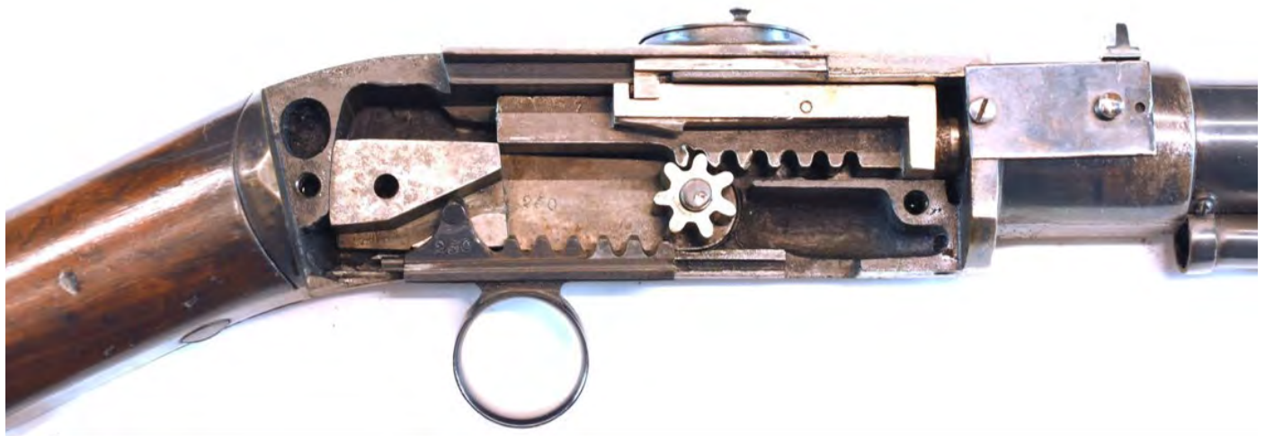
Figure 8. Jennings Breechloader interior – Action view of a Jennings breech-loading rifle, serial № 250. Visible from left to right are: the locking block (note the camming track), ring-trigger, pinion, and bolt (note the arm that rides with the bolt to interface with the priming magazine). The trigger and bolt have integrated racks that engage the pinion to work the action. The trigger is most of the way to the rear and the bolt is completely forward in this photo. Further movement to the rear will lift the locking block, and, as the trigger moves all the way back, the fourth tooth from the left is wider than the first three and will trip a sear in the lock to fire the gun. All loading is done through the rectangular gate, seen here in the open position towards the muzzle.
