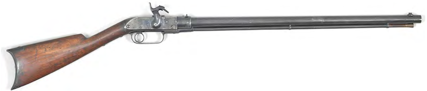
Figure 7. Jennings Breech-Loader, the second iteration of Jennings' rifle design as a single shot breech-loader vs the initial repeater that he patented.
