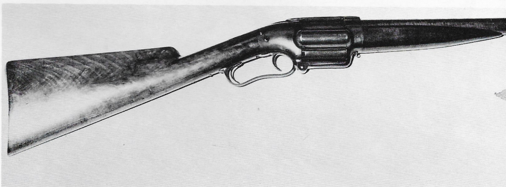
Figure 16 Roper Patent #53881 of April 10, 1866 had an enclosed chamber for carrier with slots or segments that revolved the steel shells around to be inserted full length into the barrel on firing. This rare Roper model is the cloverleaf cylinder where on firing the steel chamber is inserted only 1/4 inch into the barrel to seal it. The caliber 44 steel chamber is percussion and barrel liner may be removed so that the gun becomes a 12 gauge shotgun. This type of combination is a rarity and usually only found in air guns.
