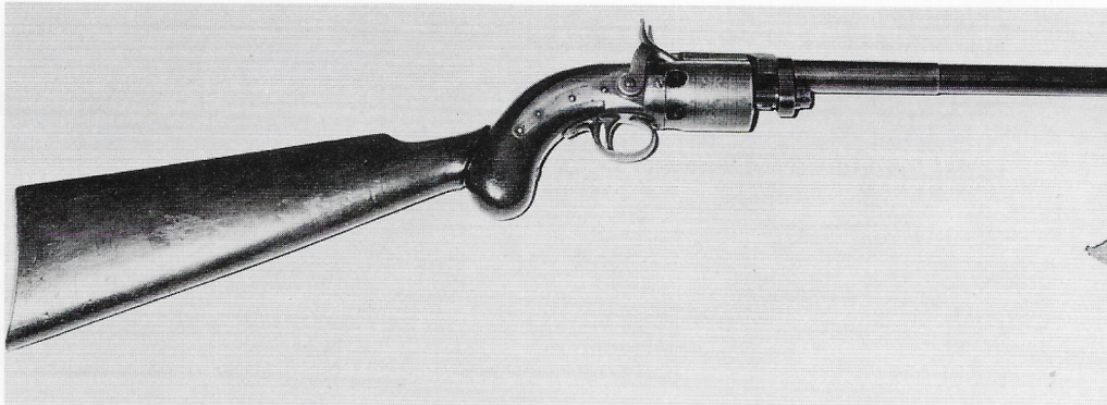
Figure 8 Wesson and Leavitt long arm, Caliber 40, six shot percussion, Serial #254. Hammer revolves and actuates cylinder by bevel gears. Colt successfully sued and stopped Wesson and Leavitt production.
