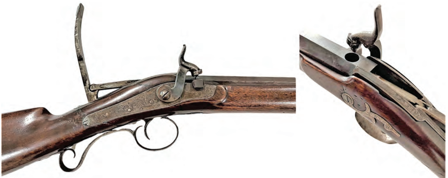
Figure 9. Chicopee Falls Co Jenks percussion sporting rifle c. 1840. Lock details with loading lever raised (left) and details of breechloading action and loading aperture (Authors collection)
