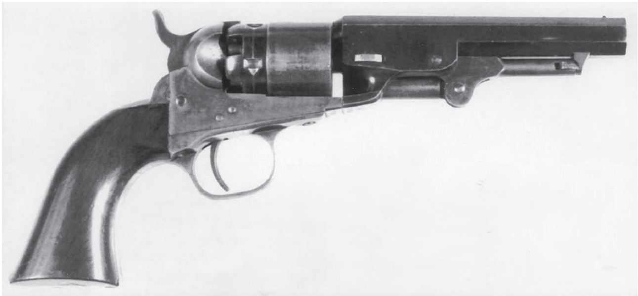
Figure 2. "Pocket Model of Navy Caliber" .36 caliber percussion pistol. Note octagon barrel, hinged ramrod, and round, roll engraved cylinder. As noted in Figure 1 , other parts are common with the "1862 Police." Robert B. Berryman photograph.
