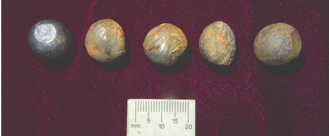
Figure 64. Unfired .626-inch ball, fired balls l to r fired at 905 f/s, 960 f/s, 960 f/s, and 1090 f/s. All balls recovered at 100 yards in sand and soil backstop. Note third ball from the left passed through a pine 4x4 target frame upright and the fourth ball from left also struck the edge of the pine target frame before embedding in the backstop.
