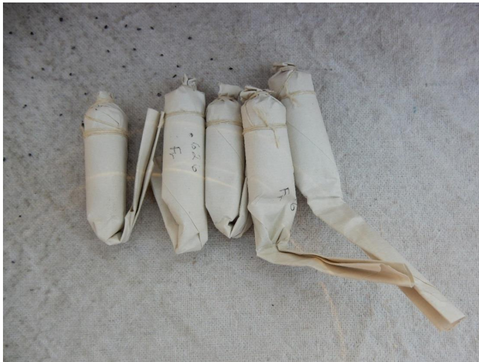
Figure 9. Completed cartridges with notes on the laid paper body denoting ball size and intended firearm.
