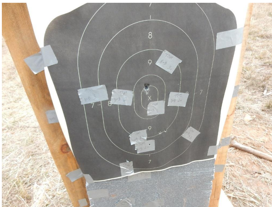
Figure 15. A buck and ball load hit on the paper target at 25 yards fired from the French Model 1763/66 musket. The ball struck the center mass with the three-buckshot striking, two at the lower 9 ring and one lower and left in the 8 ring.
