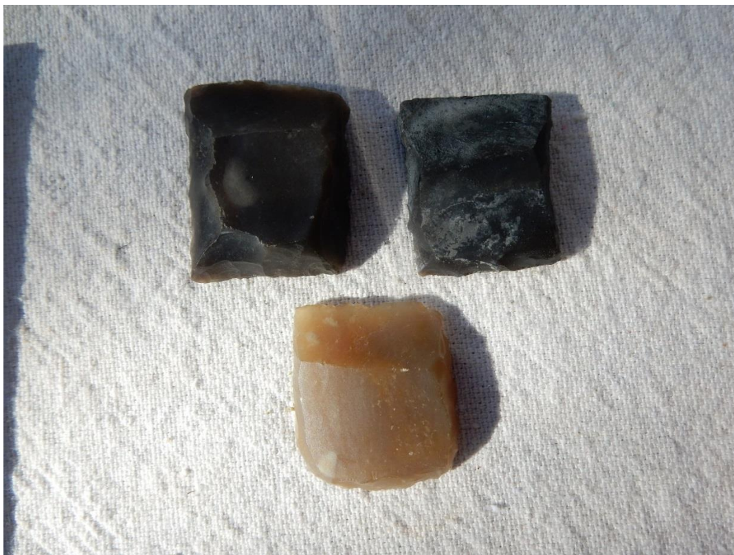
Figure 14. British and French blade-style gunflints used in the experimental firing. The top left is a British unused flint, and the top right flint is expended. The bottom flint is a French-style unused flint.
