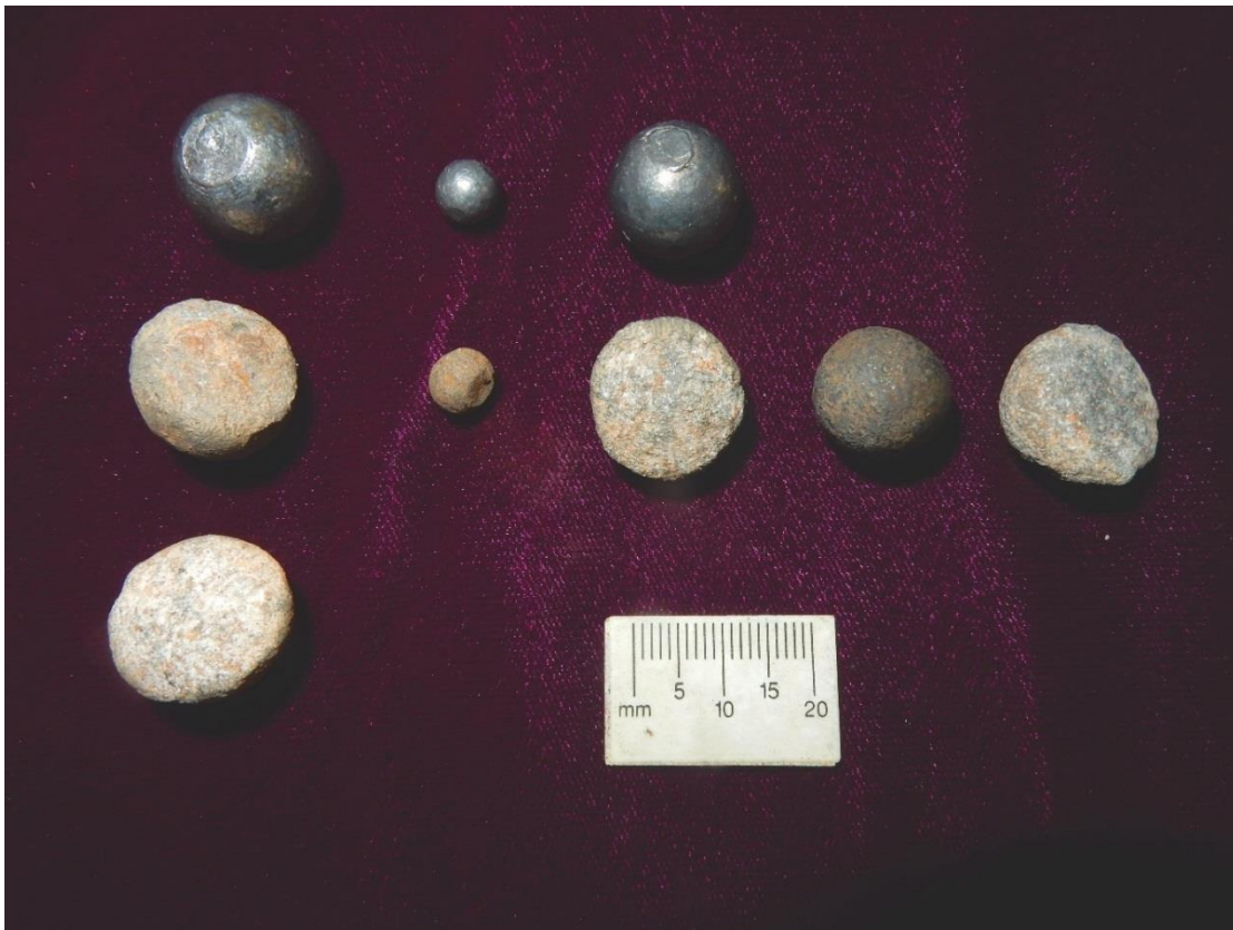
Figure 65. Left column, unfired .626-inch ball, fired .626-inch balls at 1110 f/s and 1175 f/s, both found in sand and soil backstop. Second column, unfired .282-inch buckshot and fired .282-inch buckshot at 1110 f/s found in sand and soil backstop. Third column, unfired .580-inch ball and fired .580-inch ball at 1135 f/s found in sand and soil backstop. Fourth column, .580-inch ball fired at 1155 f/s, and Fifth column, .580-inch ball fired at 1170 f/s and found in soil and sand backstop. All balls recovered at 100 yards.
