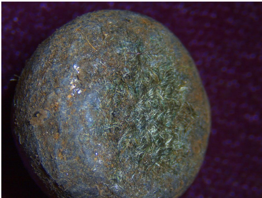
Figure 85. A 20x magnification of a ball fired from the French Model 1763/66 musket with fabric still adhering to its surface after passing through the simulated uniform cloth and gelatin blocks.
