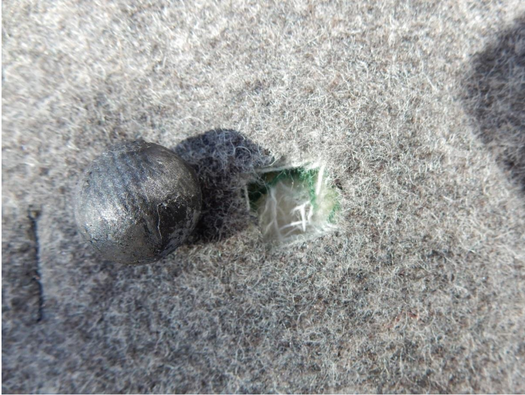
Figure 54. A fabric impressed .69-inch ball fired from the British Pattern 1756 Long Land musket with 75 grains of powder at 25 yards. The fabric impressions resulted from passing through the simulated uniform clothing.
