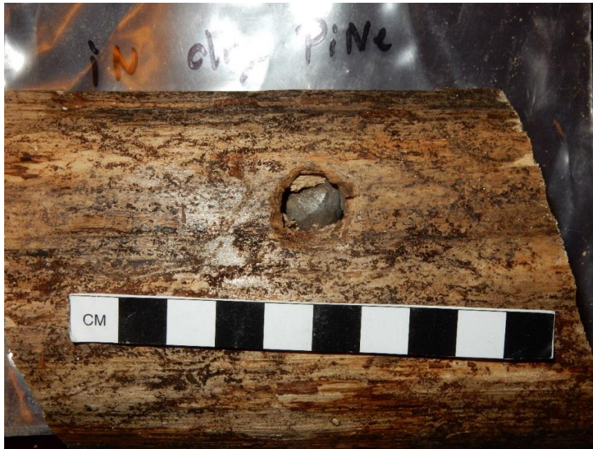
Figure 87. A .626-inch ball embedded \frac{3}{4} inch in a dry loblolly pine post. Note the deformation to the ball is moderate and would fall on the Bullet Deformation Scale as a 2.
