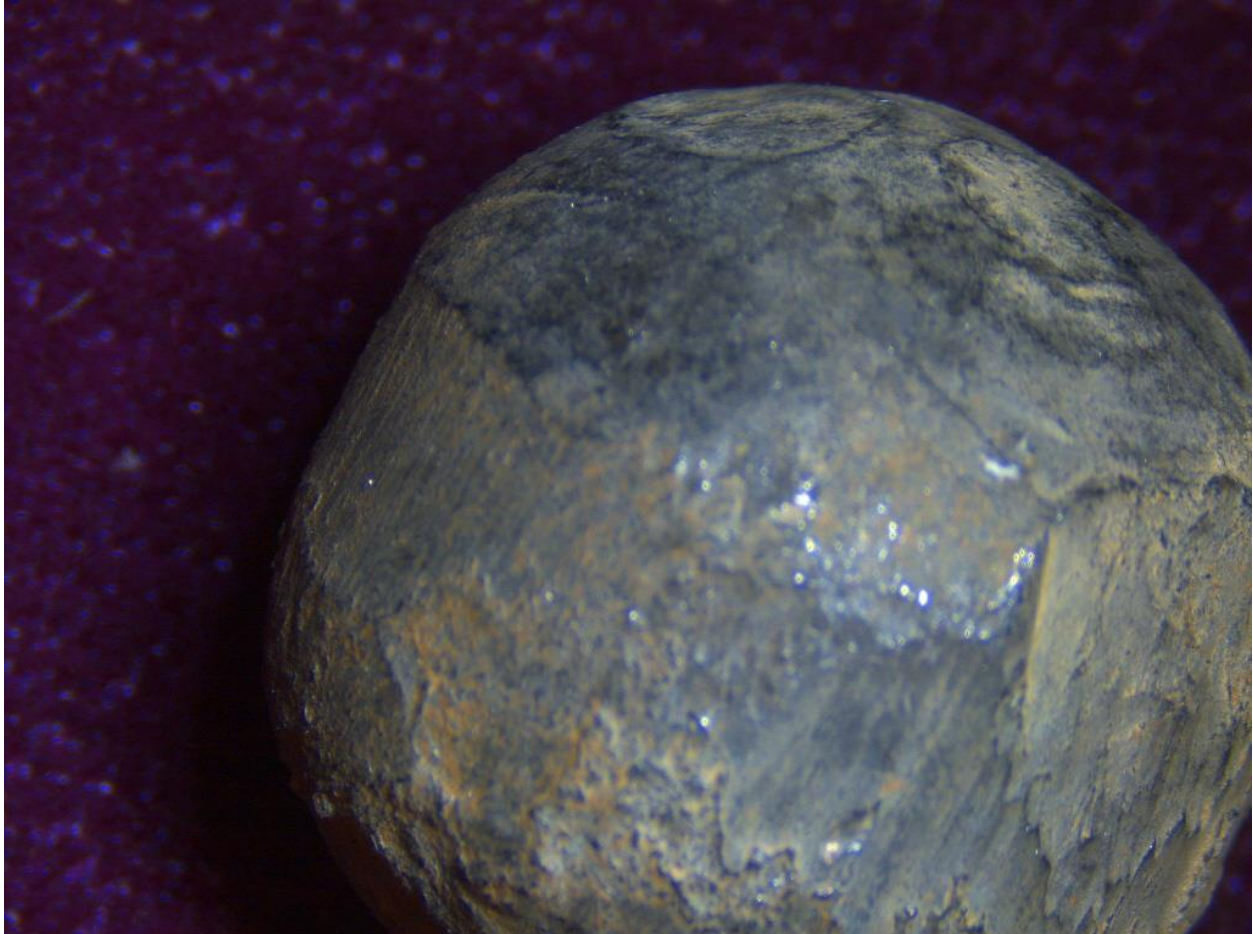
Figure 81. A 40x magnification of the bore band seen on balls fired in smoothbore guns. Note the micro striations run parallel to the line of the bore. This ball also has buckshot dimpling on the upper right surface.
