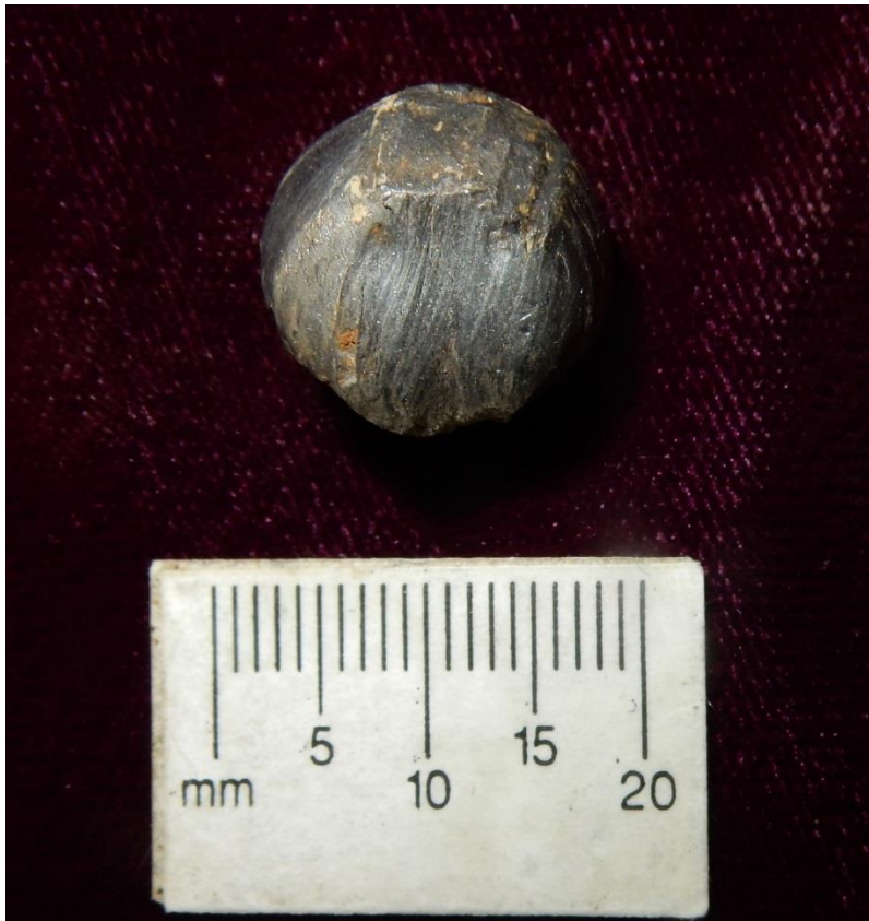
Figure 74. Fired ball with moderate impact scarring and deformation that is consistent with a Bullet Deformation Index of 2 indicating a likely velocity of 800-1100 f/s.
