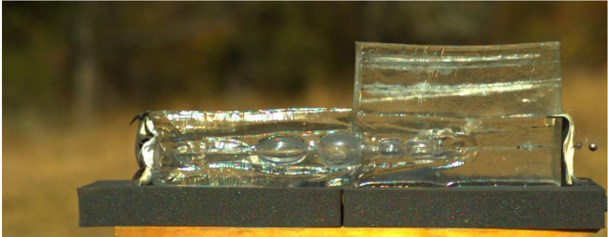
Figure 52. A .69-inch ball fired from a British Pattern 1756 Long Land musket exiting 32 inches of gelatin. Note the initial wound cavity, bits of cloth in the wound cavity on the right and a larger piece of cloth exiting the block behind the ball.
