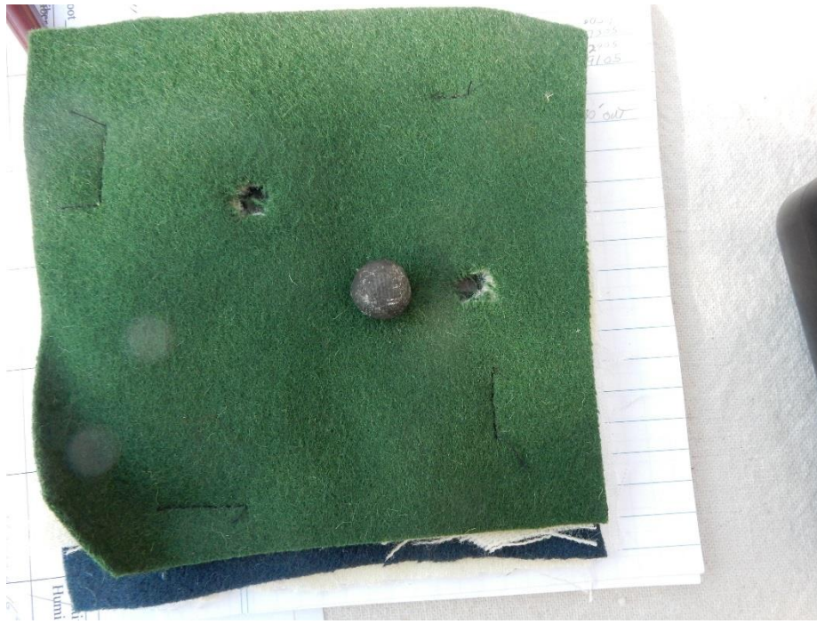
Figure 51. One of the cloth squares, 6x6 inch used to simulate a colonial era uniform clothing thickness. Two shots have passed through the cloth, and a recovered .626-inch ball is shown next to the hole it created. Note: Entry holes in cloth or tissue are often smaller than the bullet that created it due to the elasticity of the media.
