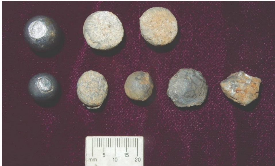
Figure 66. Top row, Unfired .626-inch ball, fired .626-inch ball at 1205 f/s and found in sand and soil backstop, fired .626-inch ball at 1215 f/s which nicked the target frame post and was found in the sand and soil backstop. Bottom row, Unfired .520-inch ball, fired .520-inch ball at 1215 f/s that hit oak palisade paling and ricocheted back into sand and soil backstop, fired .520-inch ball at 1250 f/s which hit a pine palisade paling and ricocheted back into sand and soil backstop, .520-inch ball at 1240 f/s that struck an oak palisade paling and fell to the ground below the fence, and .520-inch ball fired at 1285 f/s that went through a 4x4 pine target frame upright and was recovered in the sand and soil backstop. All balls found at 100 yards.
