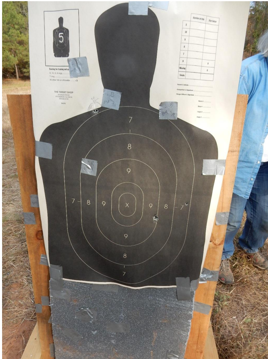
Figure 12. Man-sized torso paper target and target frame used as an aiming device during the firing. Hits were patched with duct tape and the shot noted. The uncovered holes in the target show a buckshot and ball hit from a buck and ball load.
