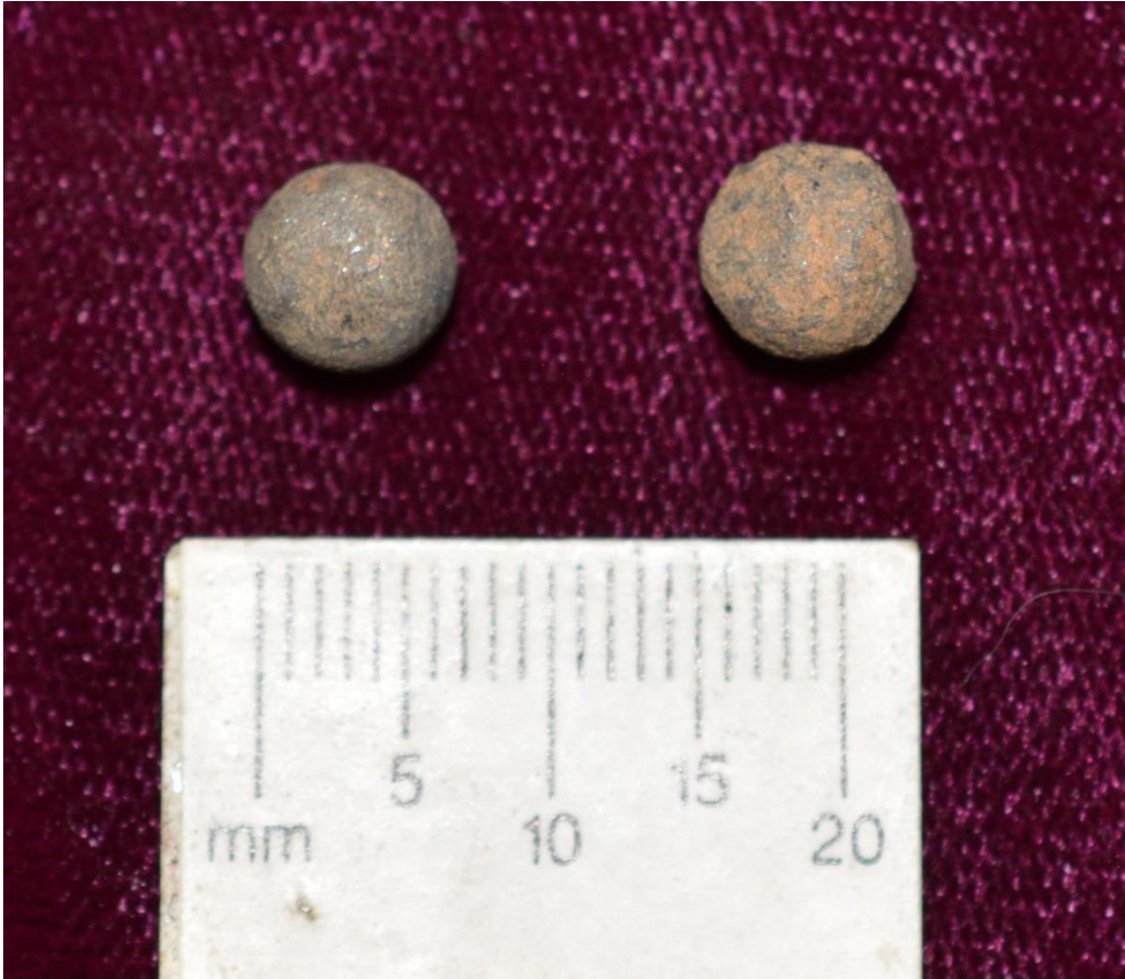
Figure 80. The slight to moderate faceting seen on the two buckshot are typical of buckshot that were in proximity to one another when loaded and fired. The soft lead is compressed in loading and firing causing the buckshot to press against and deform one another. The flat area on the left side of the right buckshot is a ramrod impression.
