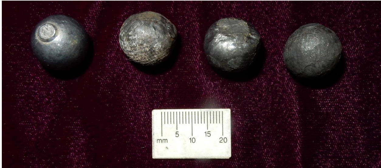
Figure 61. Unfired .69-inch ball, .69-inch ball fired at 600 f/s that struck ground surface at 100 yards, .69-inch ball fired at 630 f/s that struck a wood table, foam, and ballistic gel at 25 yards and was collected laying on the foam at the back of 32 inches of ballistic gel, and a .69-inch ball fired at 630 f/s that was captured in the ballistic gel at 25 yards after passing through 28 inches of gel. Note fabric impression on second and fourth balls.
