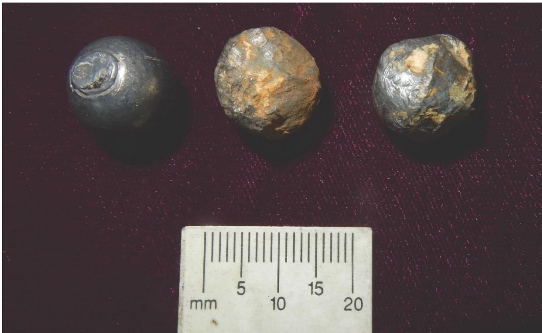
Figure 67. Unfired .520-inch ball and two fired .520-inch balls, center fired at 1345 f/s and hit pine target frame and right fired at 1350 f/s and hit pine target frame. Both found in sand and soil backstop at 100 yards. Note banding on last ball from being upset in firing from the musket.
