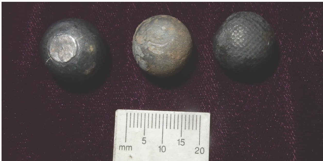
Figure 62. Unfired .626-inch ball, .626-inch ball fired at 775 f/s recovered from a soil and sand backstop at 100 yards and a .626-inch ball fired at 785 f/s and captured in ballistic gel at 25 yards after passing through 30 inches of gel. Note ramrod mark on second ball and fabric impressions on third ball.
