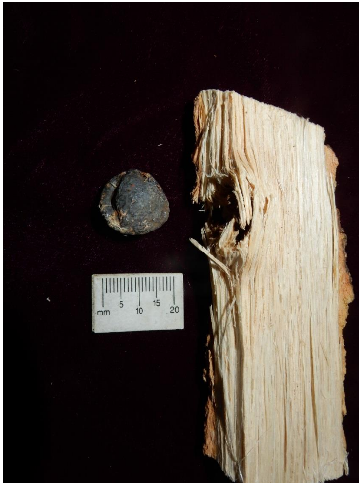
Figure 89. The .580-inch ball removed from the dry green oak. The ball is significantly deformed having hit at a higher velocity into a dense wood media. The bullet deformation is a 3 on the Bullet Deformation Scale.
