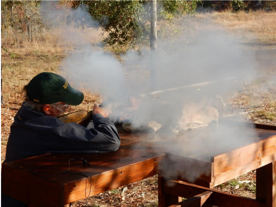
Figure 16. Charles Haecker firing the Model 1740 Potsdam musket. The musket misfired with only a flash in the pan.
