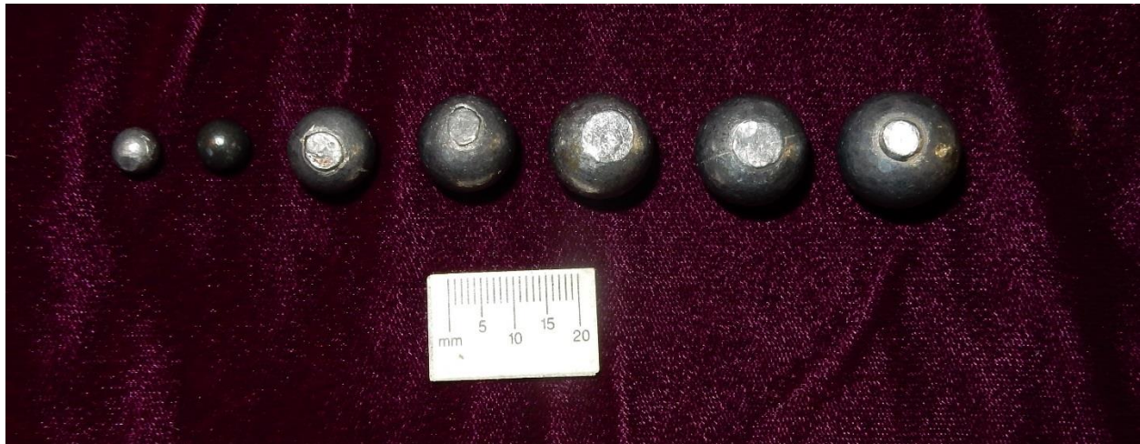
Figure 60. Unfired buckshot and bullet examples as used in the live fire experiments. l to r – .282-inch buckshot, .315-inch buckshot, .520-inch ball, .580-inch ball, .626-inch ball, .662-inch ball, and .69-inch ball.
