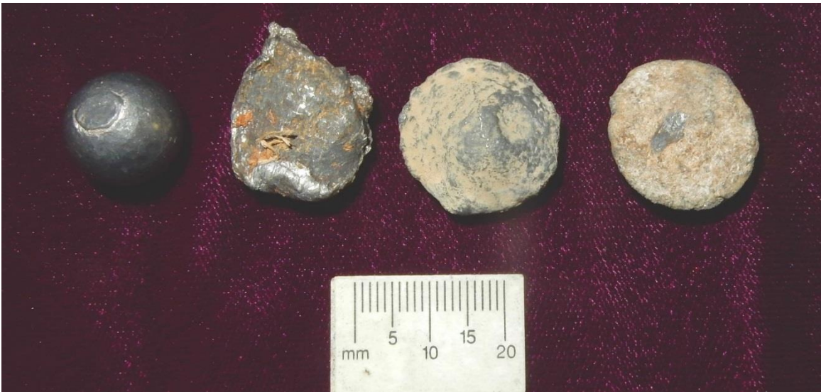
Figure 68. Unfired .580-inch ball and fired balls, second – fired at 1415 f/s and struck oak palisade paling and found in sand and soil backstop below fence, third – fired at 1435 f/s and found in sand and soil backstop, fourth – fired at 1480 f/s and found in sand and soil backstop. All balls recovered at 100 yards.
