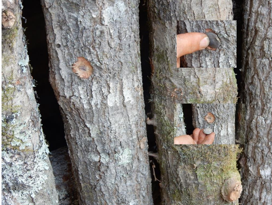
Figure 77. A .580-inch ball fired from the fowling piece hit on a live oak palisade paling with inset images showing the complete flattening or mushrooming effect of a high velocity hit on a hard media. The muzzle velocity was 1240 f/s. The ball scores a 3 on the Bullet Deformation Index.
