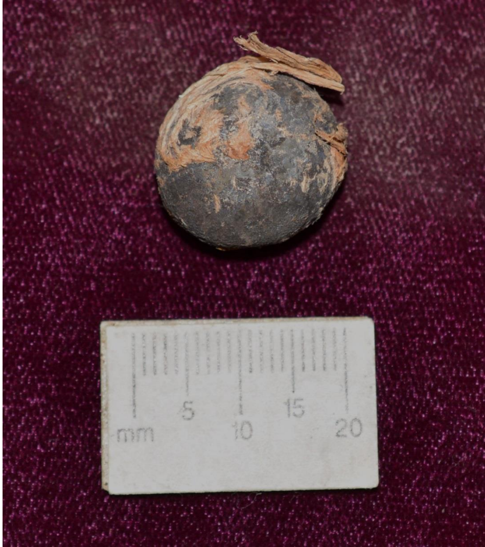
Figure 73. Fired ball that struck wood showing little to no impact deformation. This would score as a 1 on the Bullet Deformation Index indicating a likely velocity of less than 800 f/s.
