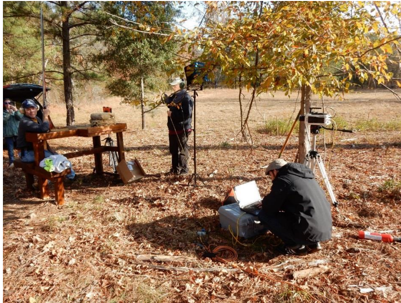
Figure 10. High-speed camera setup in progress with personnel measuring muzzle height above ground surface and preparing to calibrate the camera.
