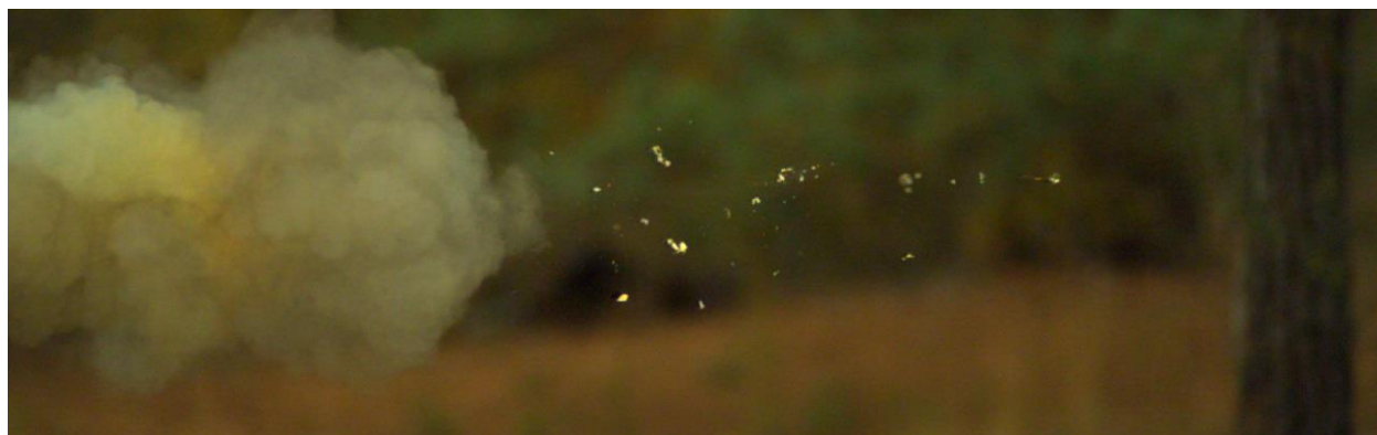
Figure 17. French Model 1763/66 musket being fired. Note the laid cartridge paper debris and the buck and ball in the center right of the debris field.
