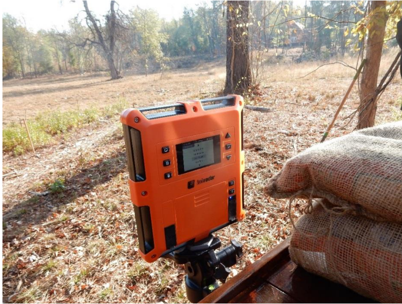
Figure 11. LabRadar® Doppler radar unit. Due to the extensive downrange gas flare and smoke from firing the unit was not capable of acquiring downrange velocity data and was withdrawn from service.
