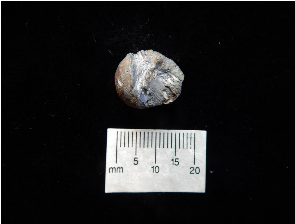
Figure 12. Impact scarring from striking the wood target frame. The damage is extensive, and some wood grain is visible on the scars, as well as wood fragments embedded in the ball.
