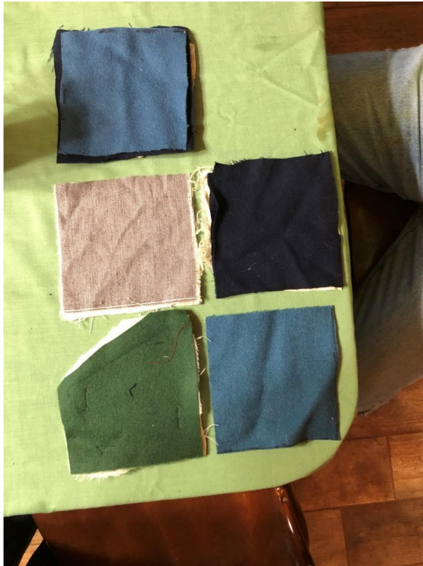
Figure 21. Simulated uniform cloth squares placed on the front of the ballistic gelatin. Top, Union overcoat, blouse, and shirt fabric; middle row, Confederate blouse and shirt fabric and Union blouse and shirt fabric; bottom row, colonial uniform coat, waistcoat, and shirt fabric, and Union trouser fabric.
