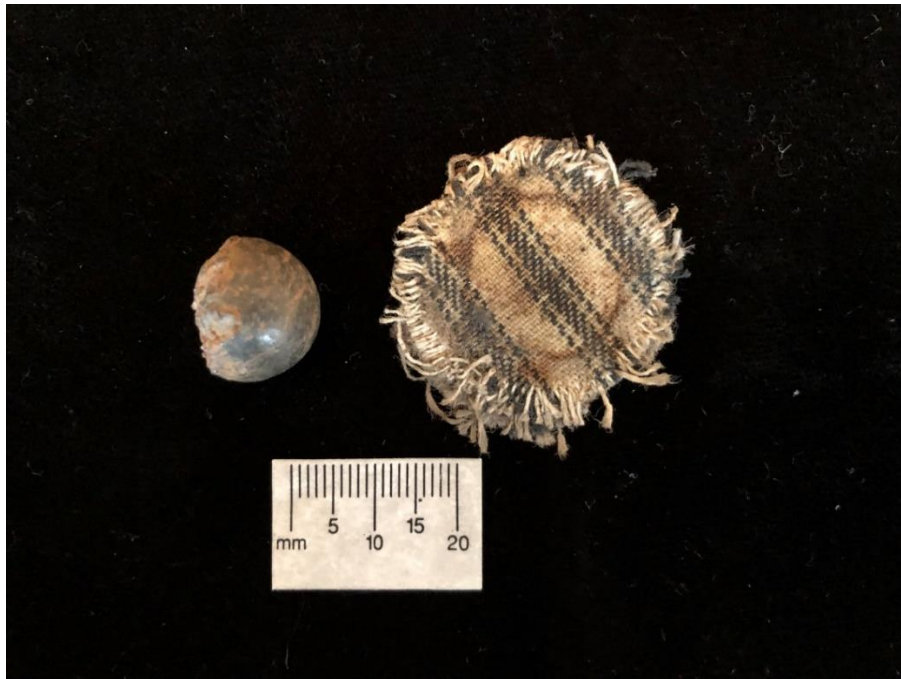
Figure 15. Rifle ball 3 and the recovered bed ticking patch. The ball was deformed on striking the target. No rifling or fabric impressions are evident on the ball. No ball fired with a patch was found to have any fabric impressions.
