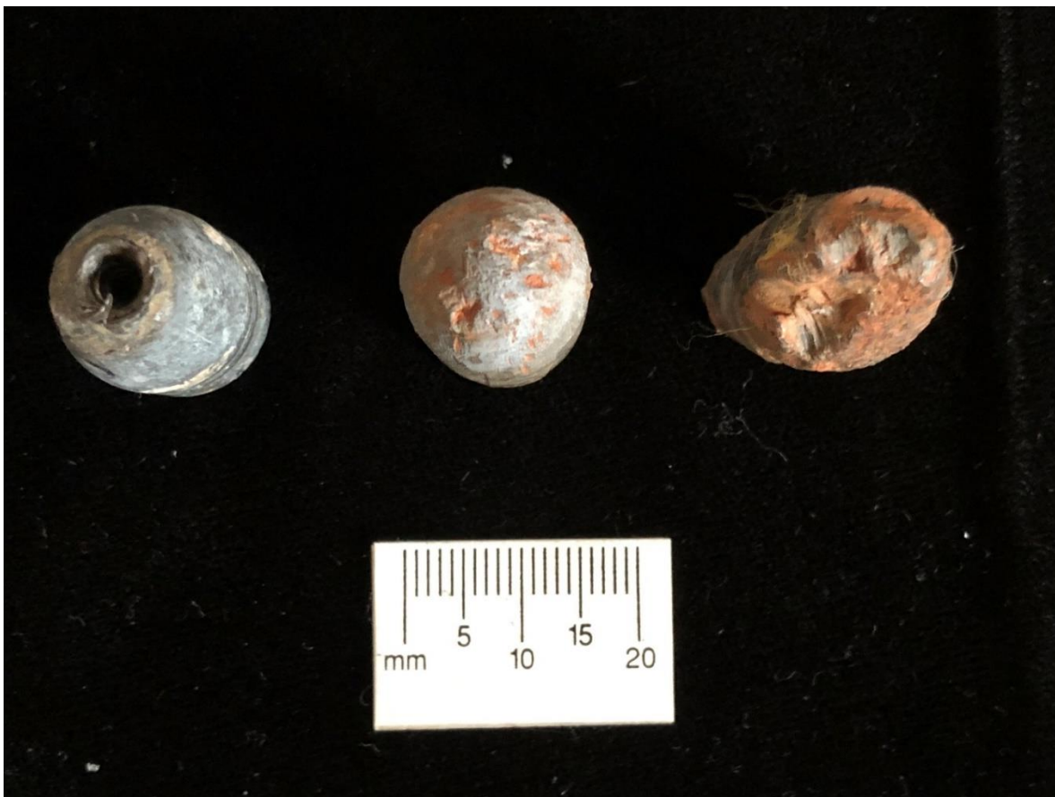
Figure 18. Nose view of the pulled and fired Minié balls used in the experiment. The bullet on the left exhibits the standard characteristic of being pulled. The center and right bullets are typical of fired bullets with nose damage from a stable bullet impact, and significant impact damage to the nose and side from being in yaw when it impacted.
