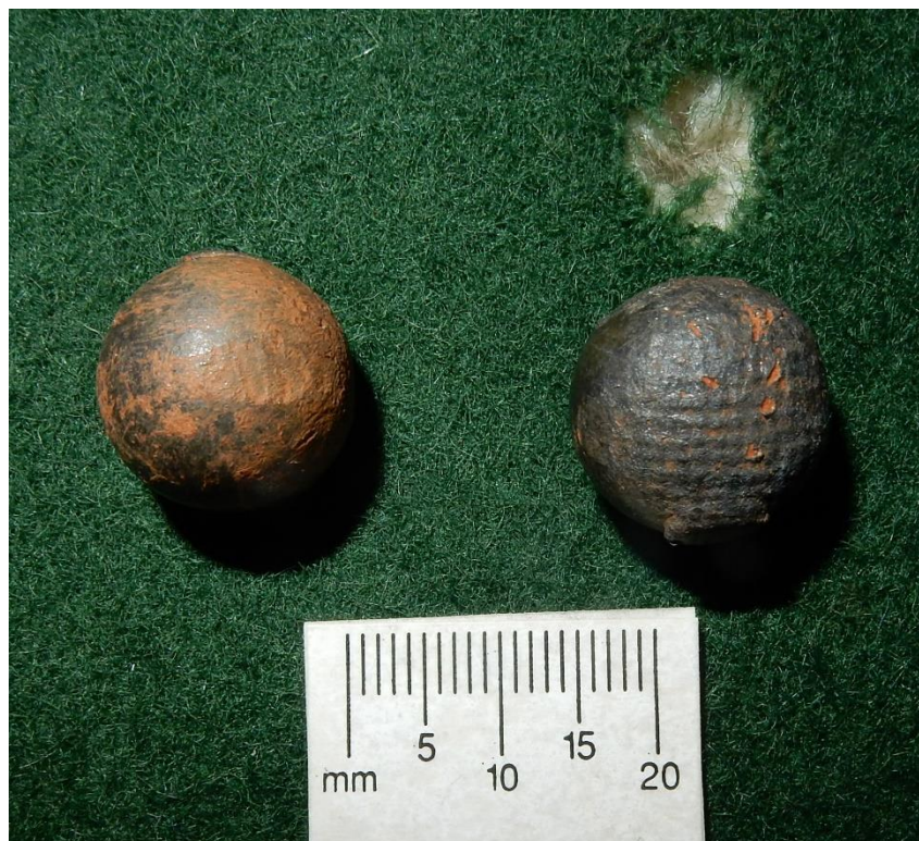
Figure 16. The colonial rifle ball 61-3 on the left exhibits compression banding and rifling impression. Rifle ball 61-1, right, exhibits fabric impressions from passing through the simulated colonial uniform cloth. No impressions of patching fabric were observed.
