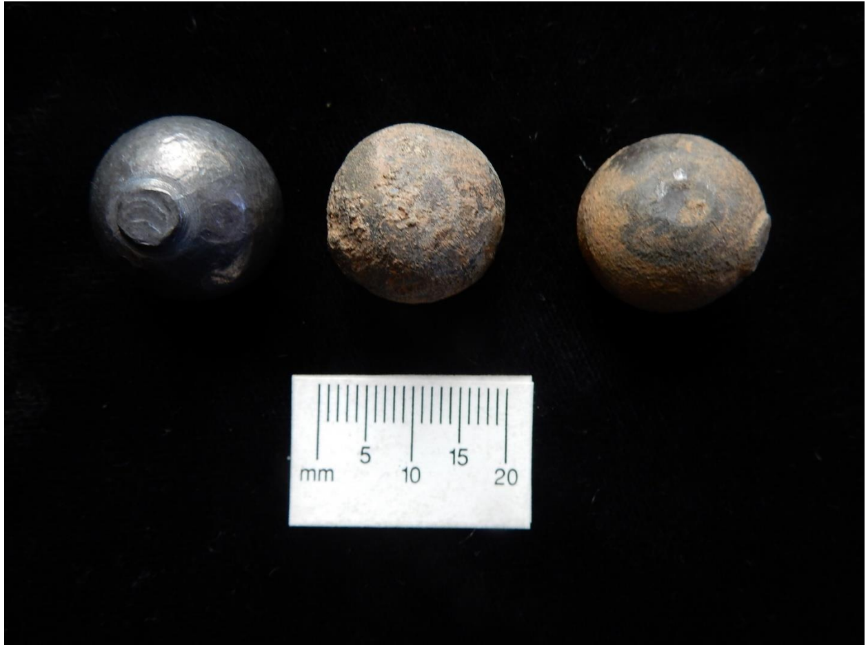
Figure 25. Ramrod marks on spherical balls. Casting sprues are also evident on the first and third balls.
