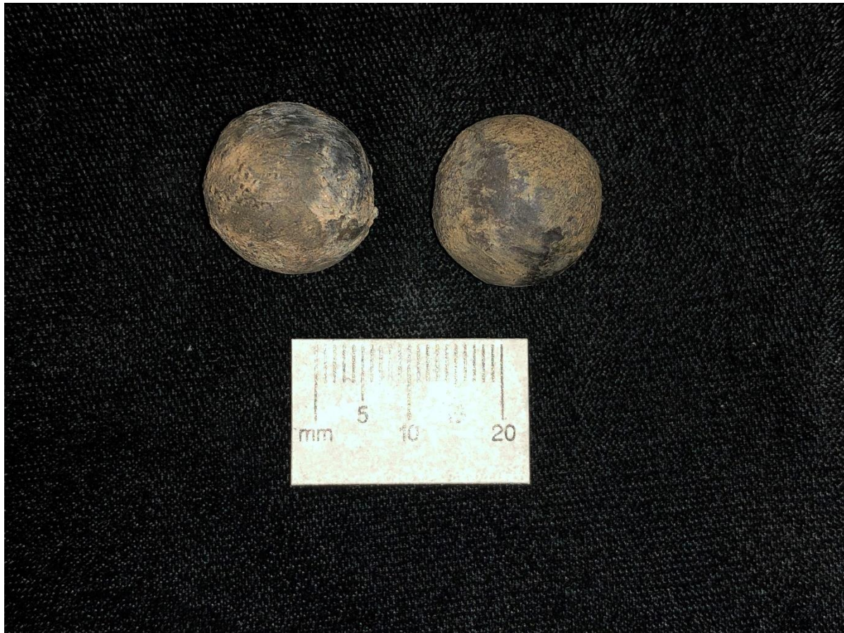
Figure 14. Double ball load, 17a and 17b showing slight deformation from contact in the barrel on firing.
