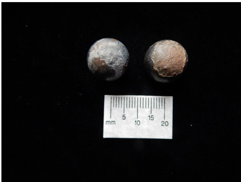
Figure 13. Examples of black powder stippling observed on fired balls.
