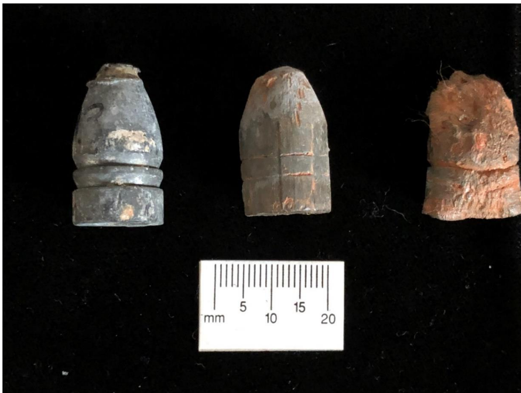
Figure 17. Pulled and fired Minié balls used in the experiment. The bullet on the left seated improperly and was pulled from the rifled musket with a ball screw. The center and right bullets are typical of fired bullets with rifling impressions evident and significant impact damage to the side from being in yaw when it impacted.
