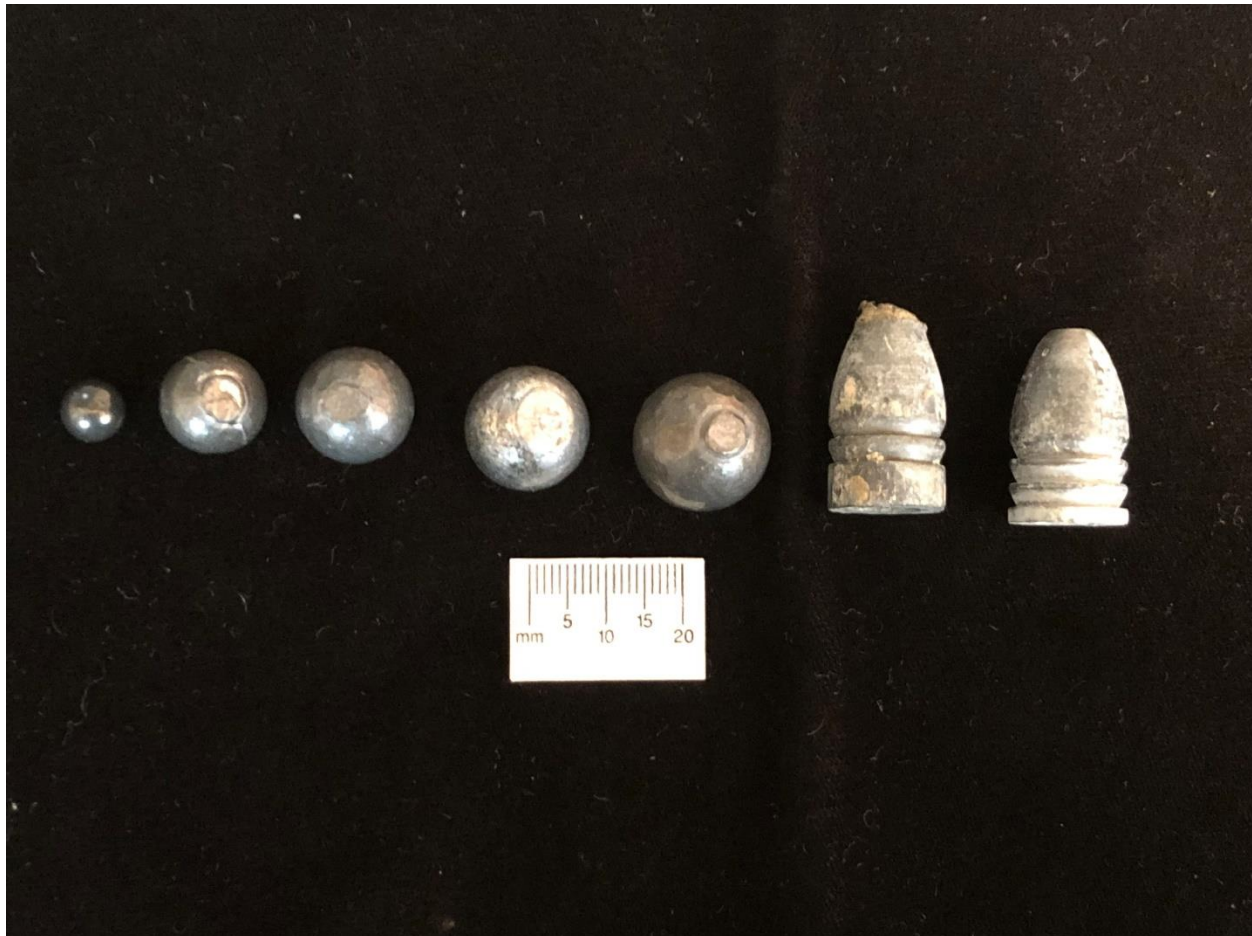
Figure 8. Unfired examples of the bullets used in the experiment. L. to R., .282-inch buckshot, .530-inch ball, .580-inch ball, .60-inch ball, .69-inch ball, .58-inch Minié ball with wide skirt base, and .58-inch Minié ball with narrow skirt base.
