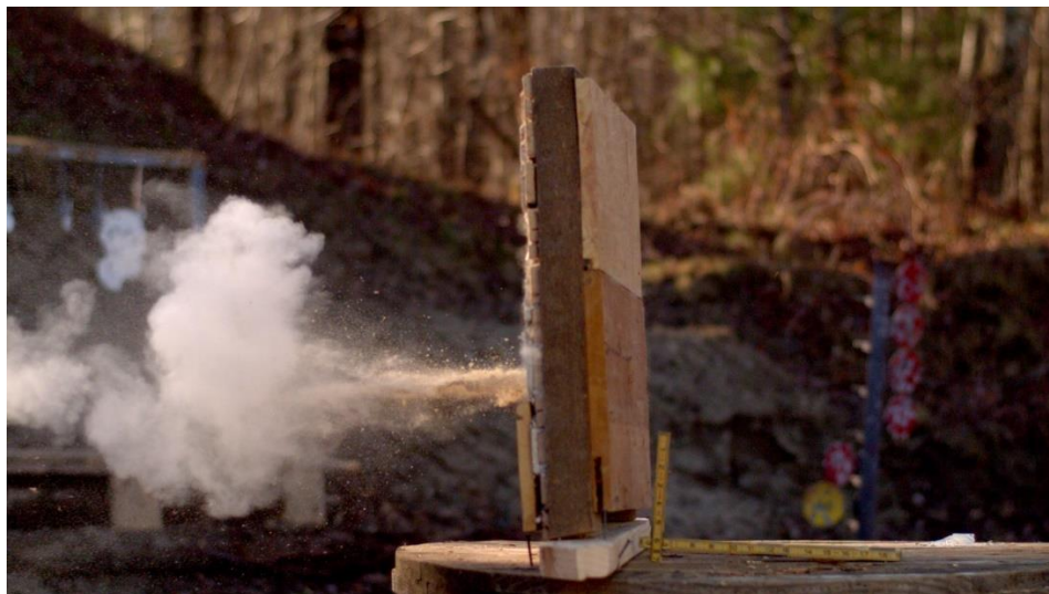
Figure 25. Still frame from the high-speed video showing the plaster dust and lath splinters resulting from the ball passing through Wall Section 3.
