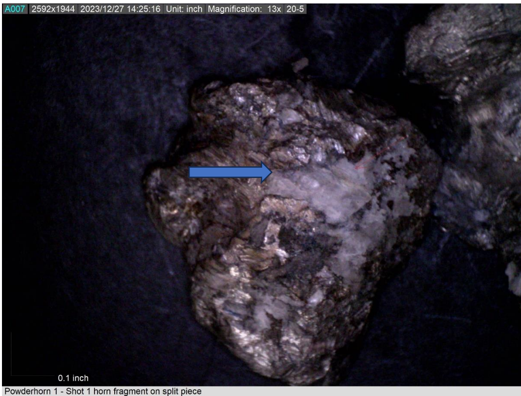
Figure 40. Photomicrograph of a piece of horn embedded in the split ball body.
