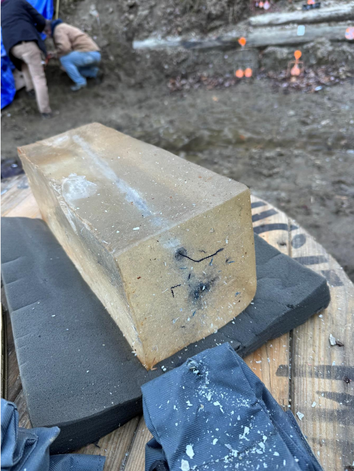
Figure 45. The wound track of the powder horn 2 shot with a piece of wool yarn still dangling from the entrance hole.
