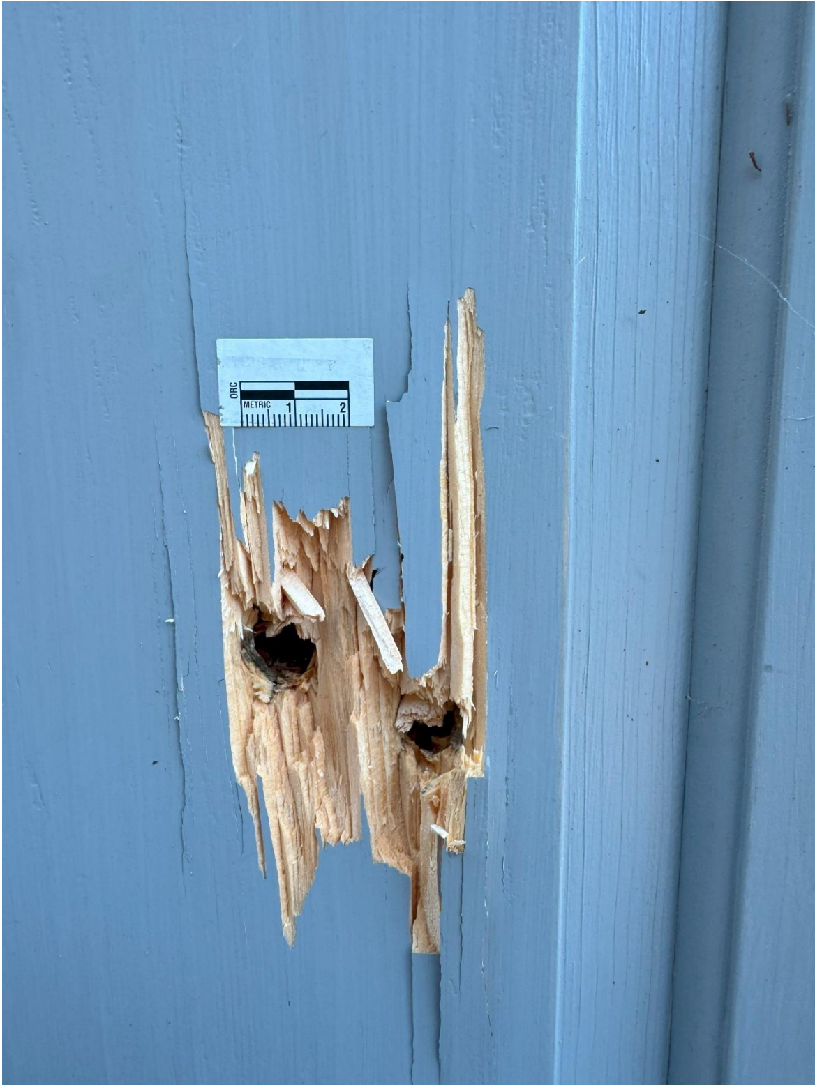
Figure 12. Wall 1 paneling exit holes for shots 1 and 2. Note the splintering and loss of wood around the holes as well as how closely spaced the bullet holes are.
