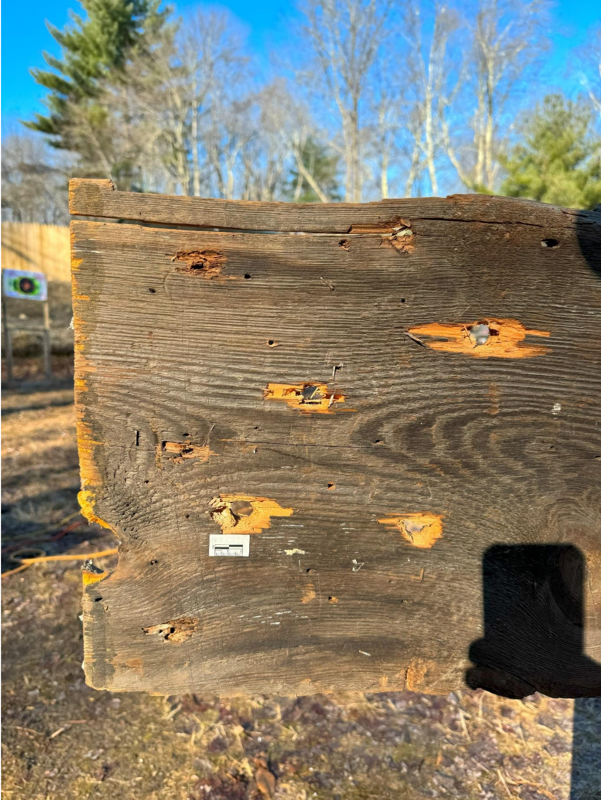
Figure 58. Exit holes in the panel caused by the .715-inch balls fired from the 1650 English lock musket.
