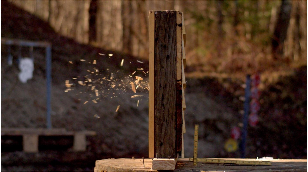
Figure 10. Still frame from the high-speed video showing wood splintering as the ball exits Wall Section 1.
