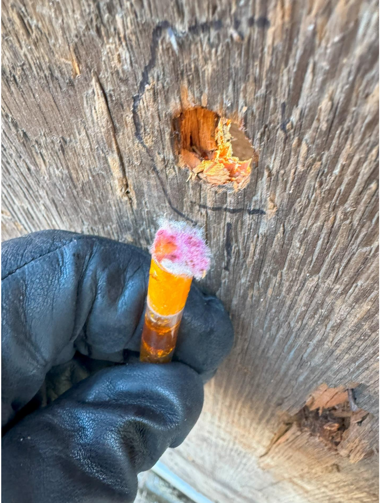
Figure 16. A positive presumptive lead test on the interior panel. This panel was never painted.
