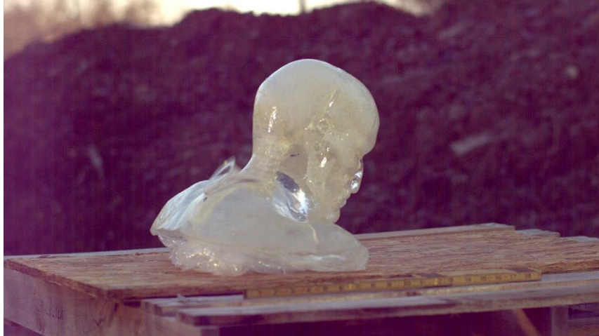
Figure 50. The ball created a splash effect as it enters the gelatin bust.
