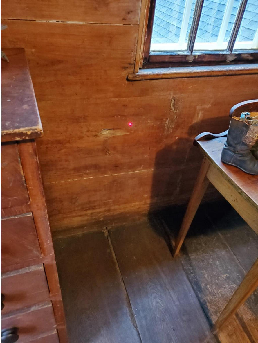
Figure 8. A bullet exit hole in the interior wall paneling of the Jason Russell house upstairs parlor. The laser dot is aligned on a trajectory rod in a bullet hole in the interior paneling across the room. There is little doubt that the wall panel hole and the interior wall paneling hole across the room originated with the same shot.
