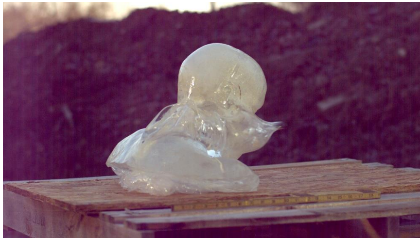
Figure 51. The ball exiting the ballistic gelatin bust. Note the massive cavitation effect on the neck and lower jaw area.
