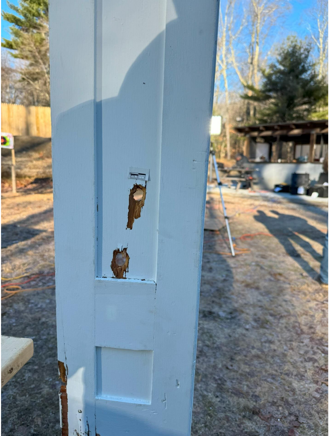
Figure 30. Exit holes showing the wood splintering after the ball passed through the shutter.
