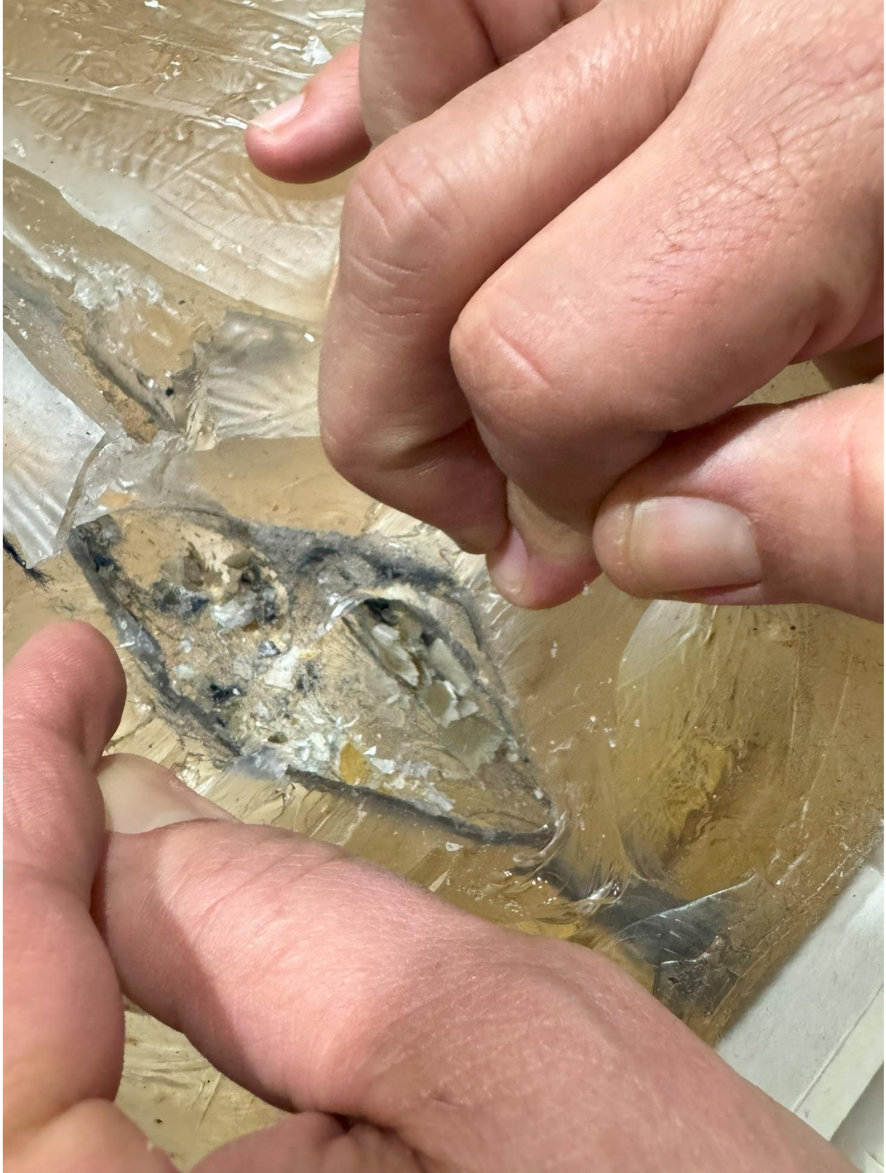
Figure 36. Horn shards and cloth fragments before removal from the ballistic gelatin wound track.
