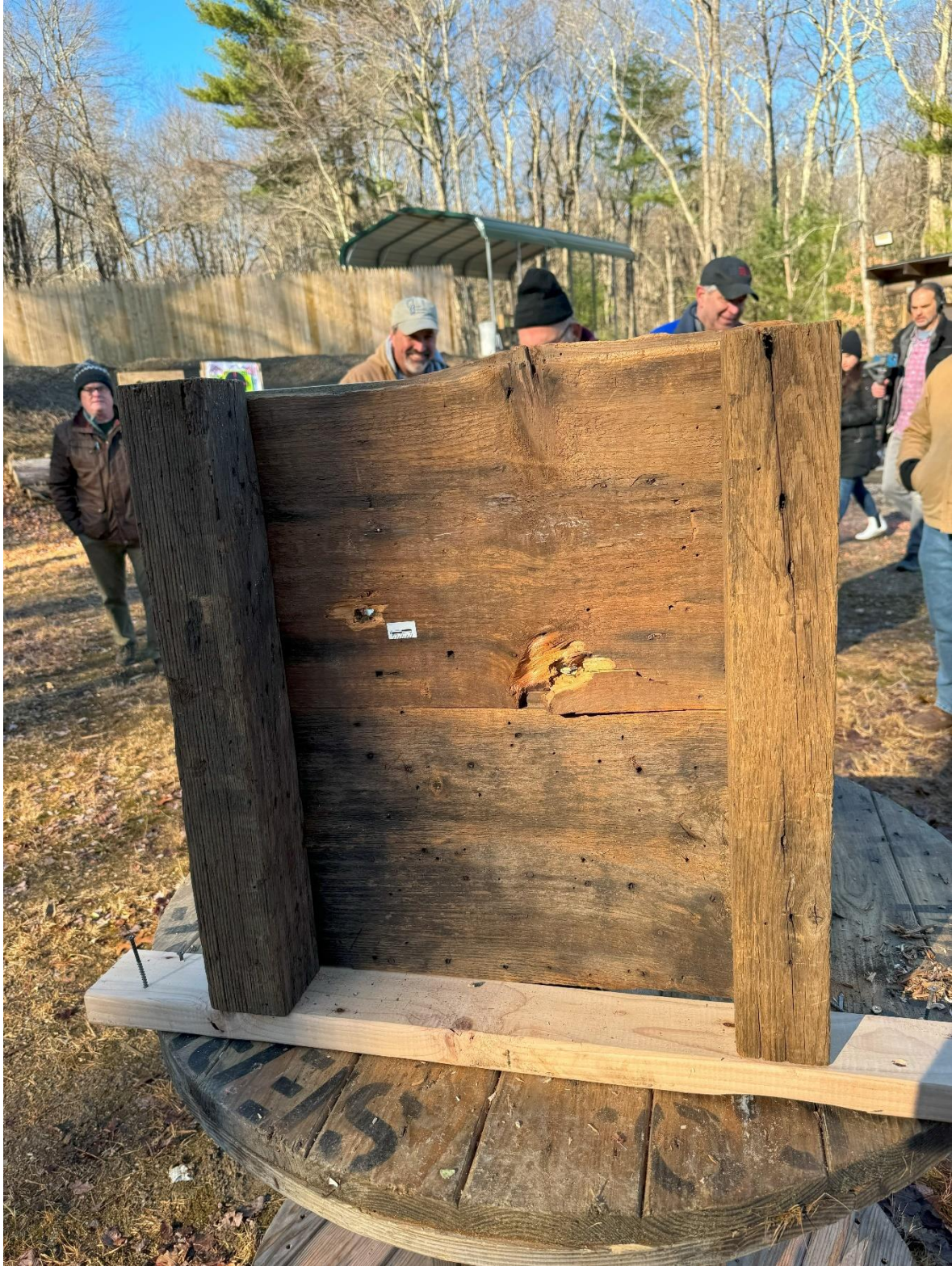
Figure 22. Wood splintering around the bullet holes in Wall 2. Note the extreme splintering around the lower hole near the feather edge joint which nearly duplicates that found on the interior of the Elisha Jones shed sheathing.
