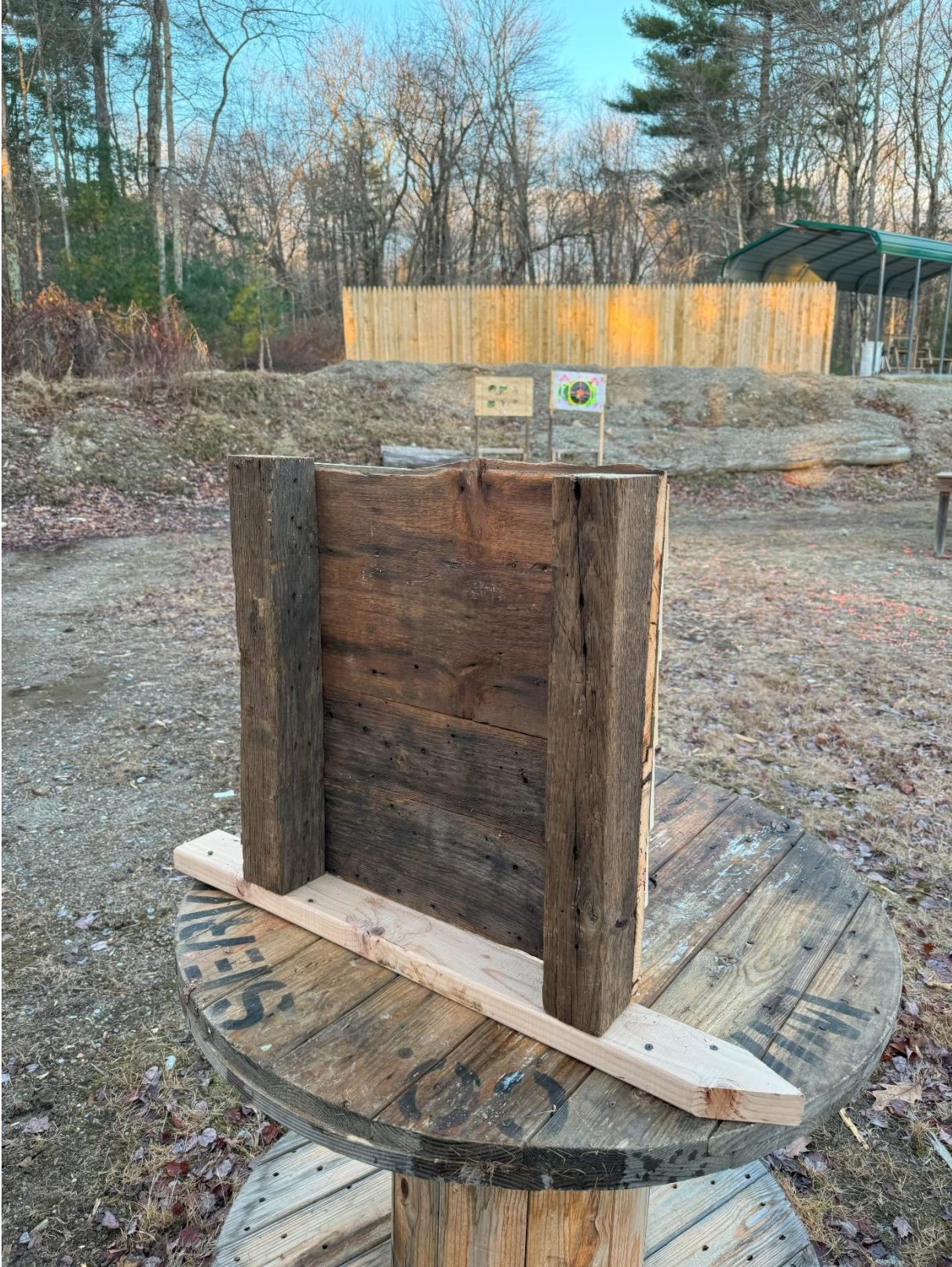
Figure 20. Clapboard and sheathing setup for Wall 2 to replicate the Jason Russell house attic and the Elisha Jones shed.
