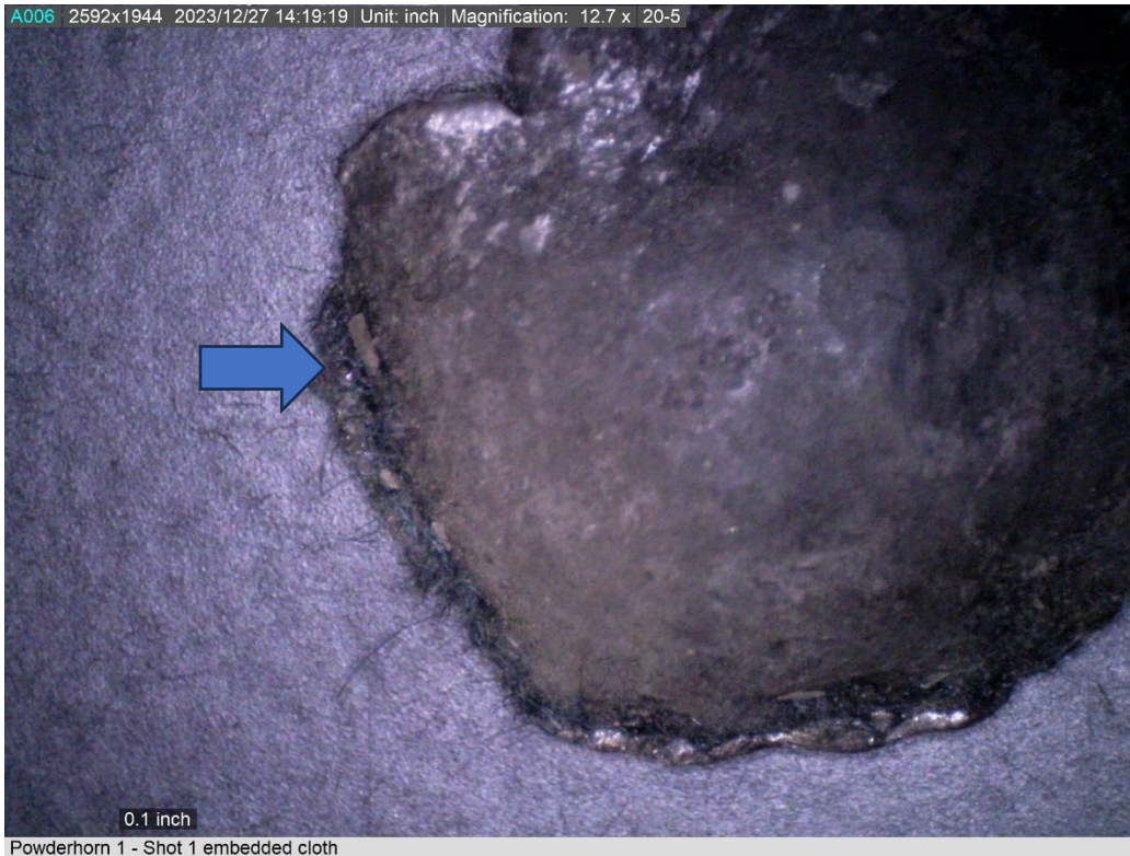
Figure 39. Photomicrograph of the edge of the split ball showing cloth fragments embedded in the lead.
