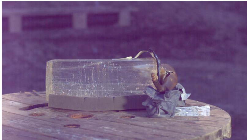
Figure 34. The ball shatters the horn, is split in two, and the two wound tracks can be seen being started as the ball passes into the ballistic gelatin block.
