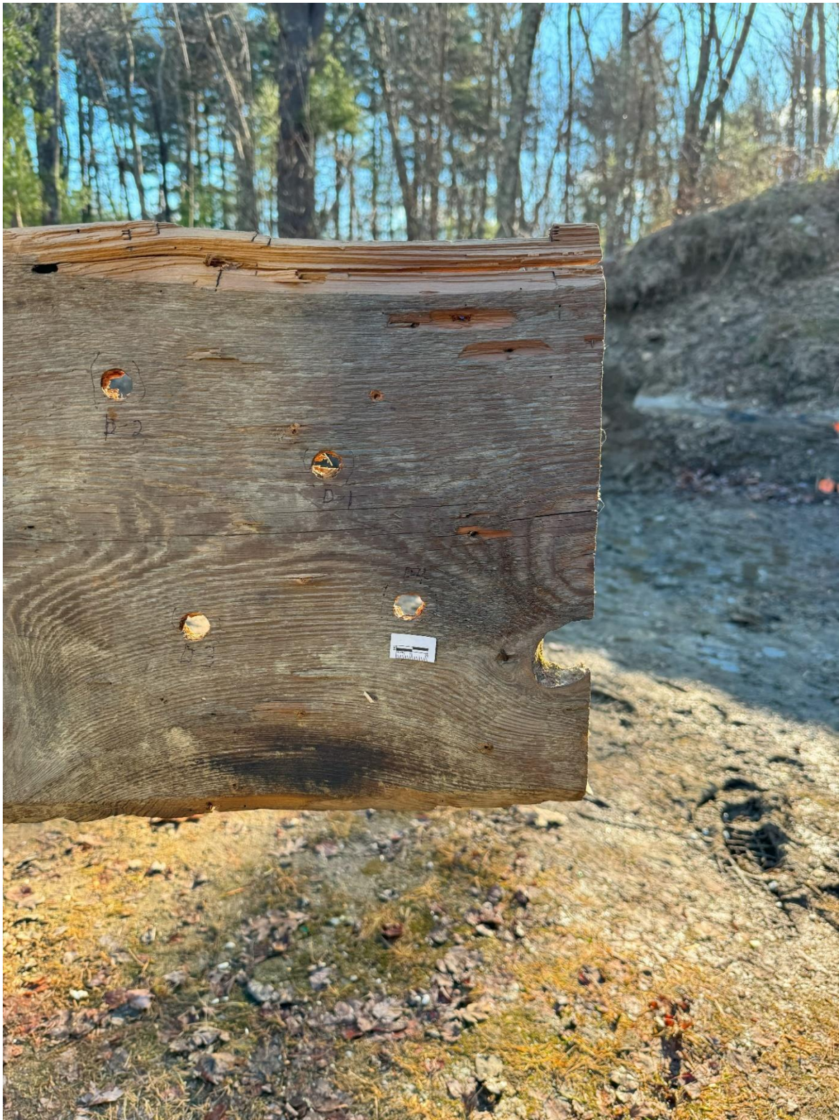
Figure 57. Entrance holes in the panel board caused by the .715-inch balls fired from the 1650 English lock musket.
