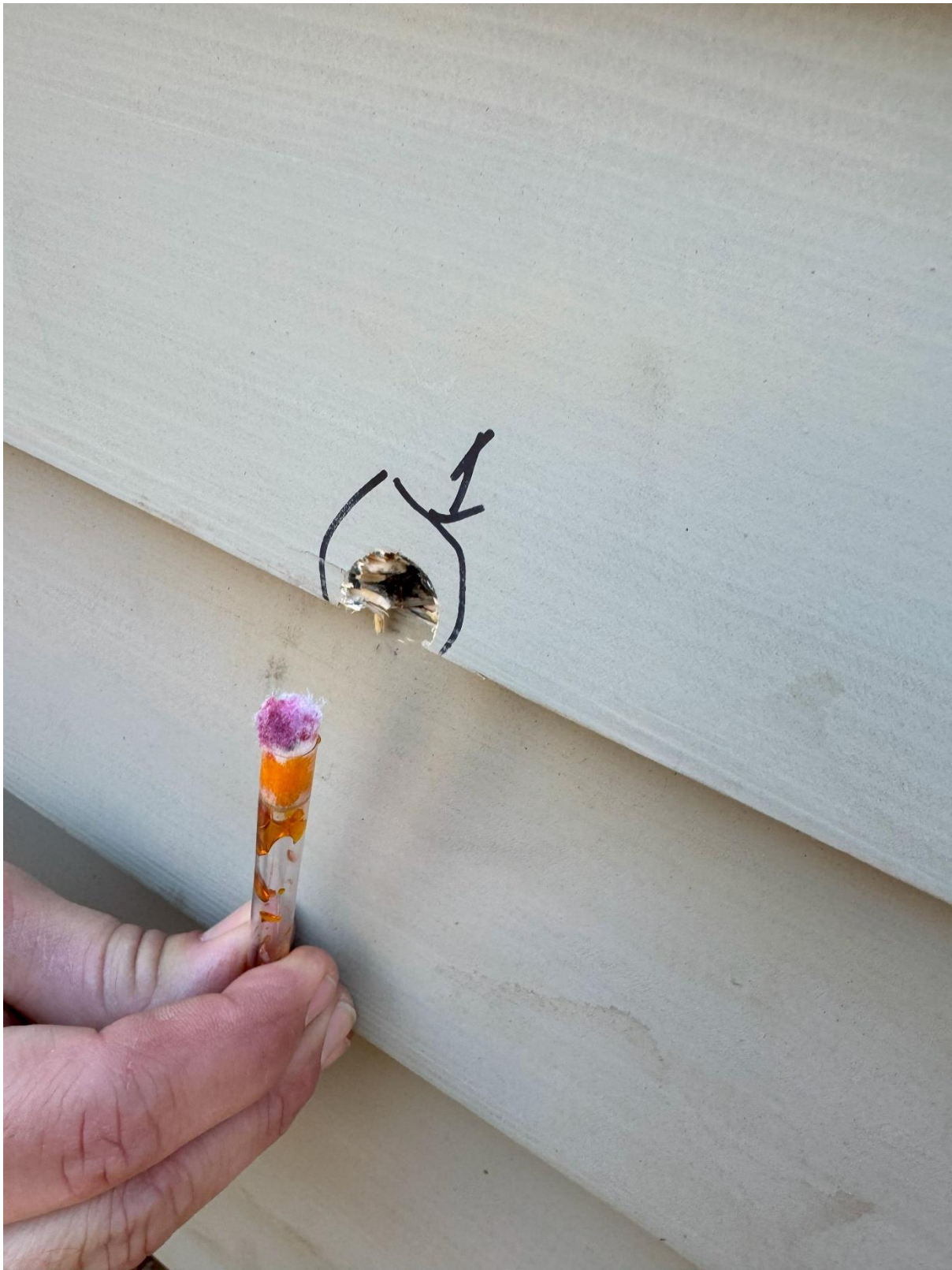
Figure 13. Positive presumptive lead test on the Wall 1, shot 1. The hole was swabbed on the interior. The paint is modern latex.
