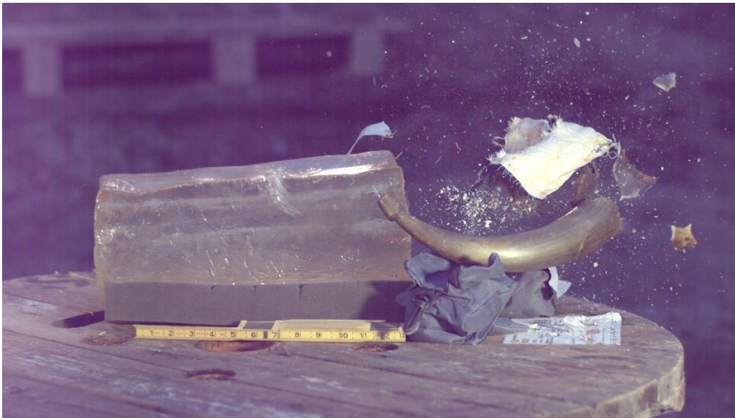
Figure 44. Powder horn 2 in the process of shattering after being hit by the ball. Note the cloth flying through the air, fragments of horn being dispersed, and the end plug being blown out of the horn.
