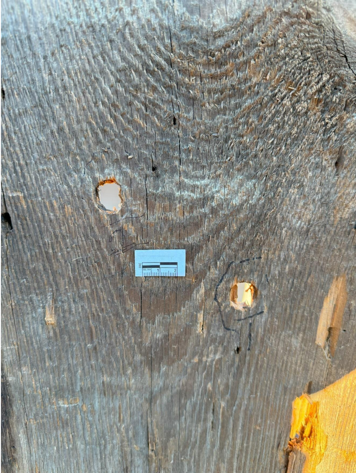
Figure 15. Interior wall panel for Wall 1 placed 15 feet (3 meters) from the wall and paneling showing entrance holes for shots 1 and 2. Note the wide spacing between the two shots compared to the comparable holes in Wall 1 clapboard. This is due to the effect of media causing the balls to deflect in their flight.
