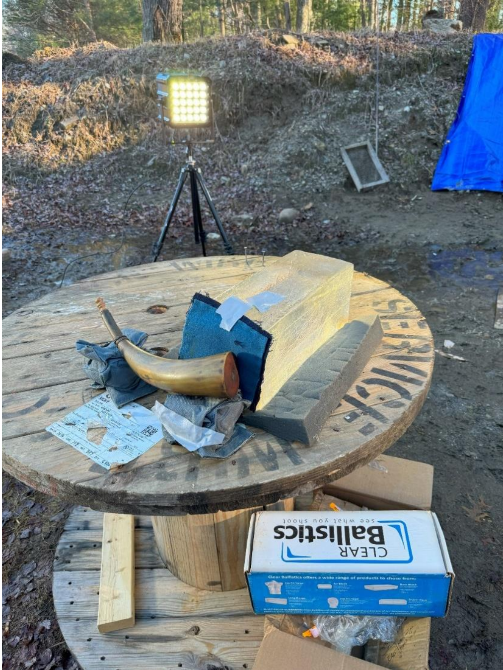
Figure 32. Powder horn 1 ready to shoot. Note the cloth and ballistic gelatin block.
