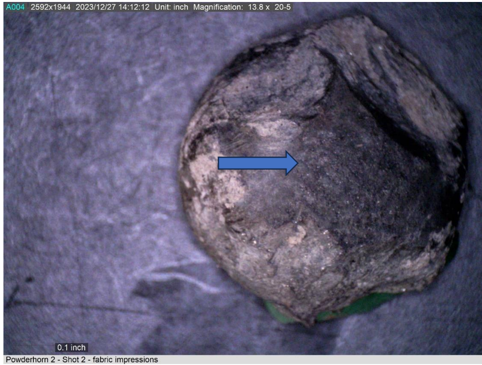
Figure 46. Photomicrograph of the split ball surface showing fabric weave impressions from passing through the cloth.
