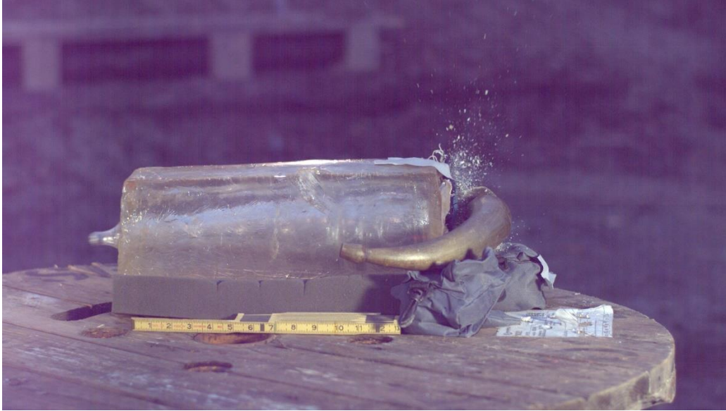
Figure 43. The ball exiting the ballistic gelatin block and powder horn 2 starting to shatter.
