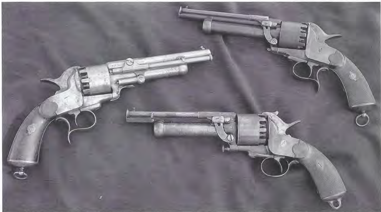
Figure 16. The more commonly recognized Le Mat revolvers: first model (left), transitional model (upper right) and second model (bottom right). These pieces were made under the Le Mat and Girard partnership, using later patents and differ significantly from the pieces made by “A. Le Mat & Co.” (Photo by Doug Adams.)
