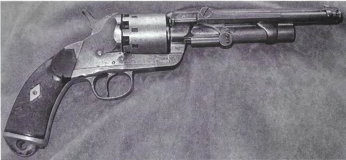
Figure 7. Krider engraved No. 2. This spectacular find represents the efforts of Le Mat and Beauregard in the field of small arms. This nine-shot, .41 caliber revolver and 18-gauge shotgun offered considerably more firepower than its Colt competitor. (Photos by Doug Adams, Courtesy of Cliff Young.)
