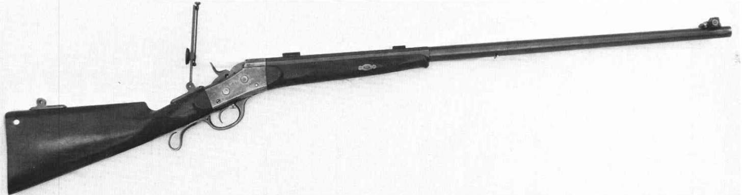
Gove-Remington under lever Creedmoor rifle with 34 inch .44/105 caliber half octagon barrel. This rifle is mounted with both tang and heel position vernier rear sights and a spirit level windgauge front sight. It was the prize at a match in Denver in 1876.
