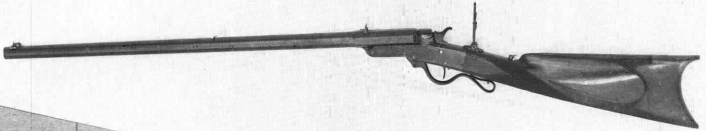
Gove-Maynard rifle marked with the last marking on the right side of the frame. The 26 inch barrel has been modified to a cartridge similar to the .40/50 bottleneck, the buttstock has been changed, and the tang sight and breech have been modified.
