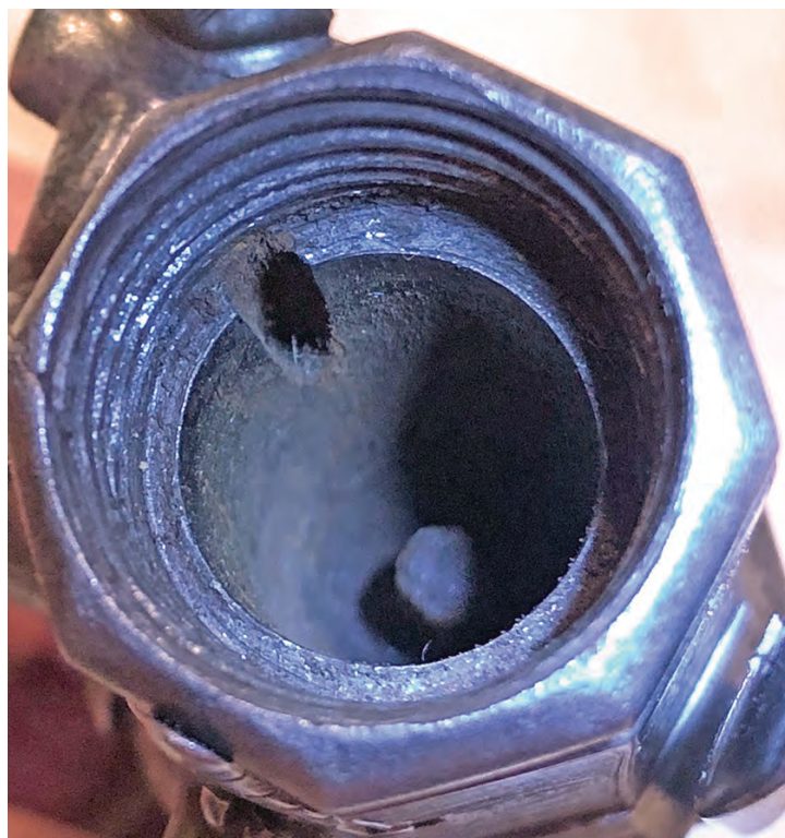
Figure 5. A view of the pillar breech. The breech is very deep, with the pillar far down—enough room for two shots. Although the pillar looks off-center in the right photo, it is central. In both photos, the end of the forward-shot ignition channel is at 11 o'clock in the left image, and at 4 o'clock in the right.
