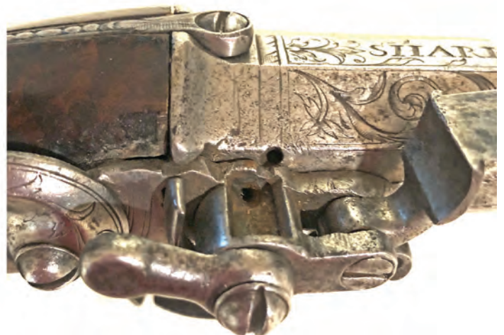
Figure 4. The pan and touch hole for the forward (first) shot (left). The control lever points forward. The pan and touch hole for the rear (second) shot (right). The control lever, rotated 180 degrees, points backward. The ignition flash will also enter the forward touch hole, but without any effect.
