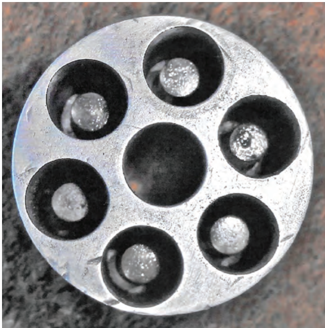
Figure 7. The Devisme cylinder, containing the Thouvenin pillars (left) and with the pillars removed (right). Note the nipples and the ignition channels are part of the pillars. Photos courtesy of Bolk Antiques.
