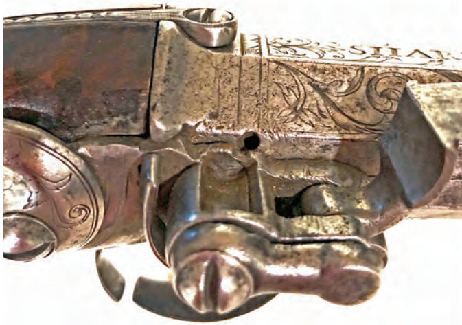
Figure 4. The pan and touch hole for the forward (first) shot (left). The control lever points forward. The pan and touch hole for the rear (second) shot (right). The control lever, rotated 180 degrees, points backward. The ignition flash will also enter the forward touch hole, but without any effect.
