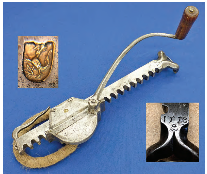
Figure 5. As an alternative to the windlass, the Cranequin could be used to span heavy siege bows. As shown above it was a clever combination of gears and rack and pinion, creating a great mechanical advantage that could span the heaviest crossbows. A superb example of a Cranequin, dated 1558. (bottom, authors Collection).
