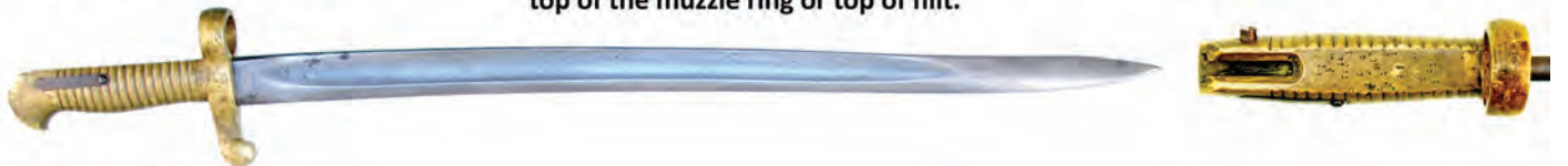
Figure 24. Ames-produced bayonets with 20" length blades fit the barrel of the M1841 barrel. These bayonets were made for a stud-only or a stud and guide method of attachment. The socket bayonet is a reused M1835 socket bayonet.
