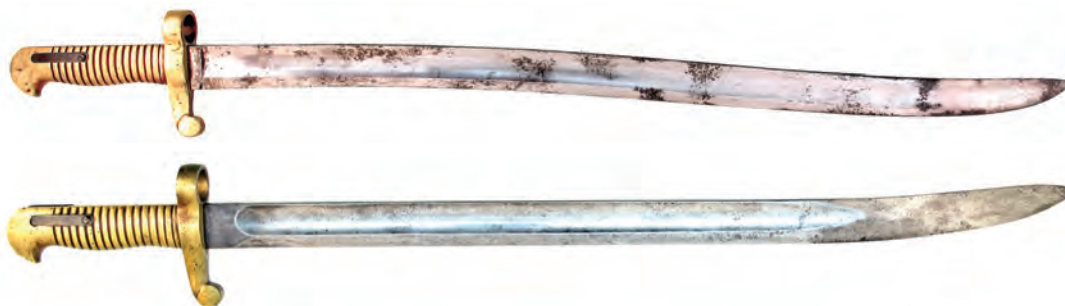
Figure 26. Whitney Bayonet Models-2 & -3 fit on the Whitney Type 2 rifle. Most important, the bayonet mating number on the muzzle ring aligned with the barrel mating number on the left side near the front sight.
