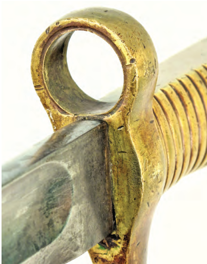
Figure 22. Whitney used an iron shim to reduce the bore diameter of the muzzle ring to fit on a Whitney Enfield barrel (Author's collection).
