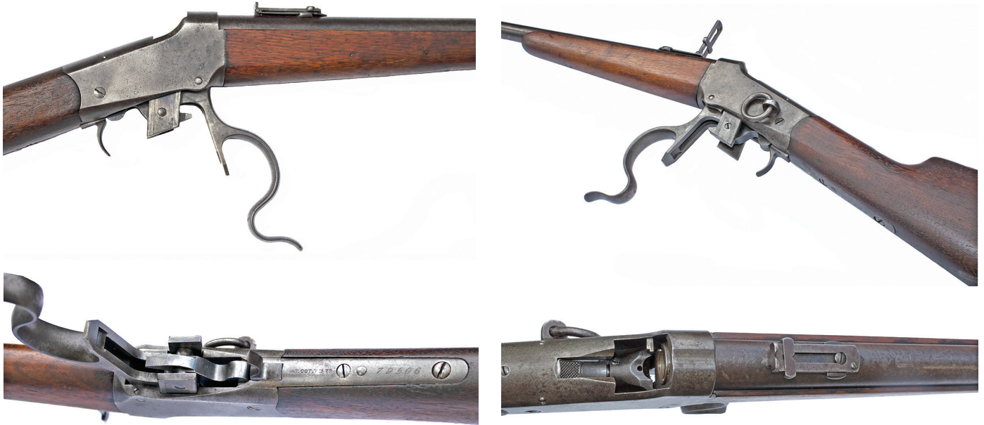
Figure 4. Winchester Single Shot carbine serial number 79506 with action open, right side (upper left) and left side (upper right). Bottom view of carbine with action open and serial number markings (bottom left) and top view of carbine with action open showing extractor and internal mechanics (bottom right).
