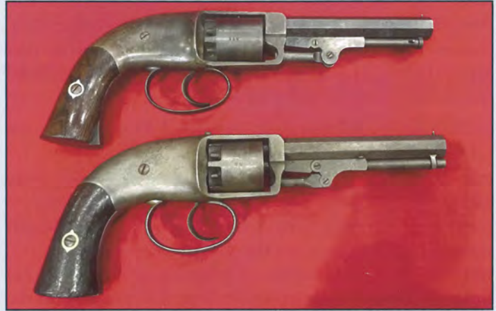
Figure 2: The nearly identical small frame Pettengill revolvers. The .34 caliber Navy model is above (#371), and the .31 caliber Pocket model is below (#95). Note the greater width of the Navy frame at the yoke, as well as the slightly longer cylinder and cylinder cavity. GOODSON COLLECTION.
