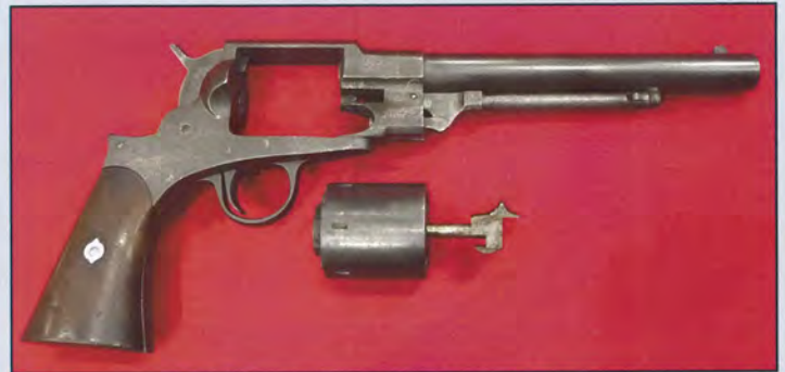
Figure 1: Freeman .44 percussion revolver (#663). Note Freeman-patented cylinder axis pin and locking catch. GOODSON COLLECTION.
