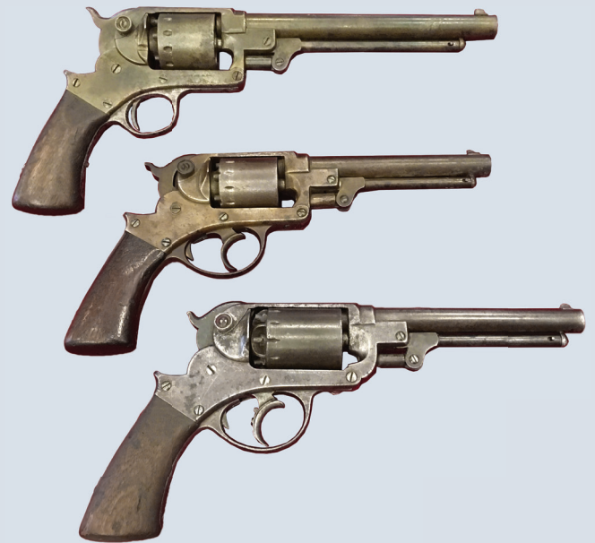
Fig. 1 - The Three Starr Brothers; the .36 double action (bottom), .44 double action (center) and .44 single action (top). Note that except for the change from double to single action around 1863, and the longer barrel length of the single action, the basic configuration of these three models remained largely consistent throughout Starr's production of over 59,000 revolvers.
