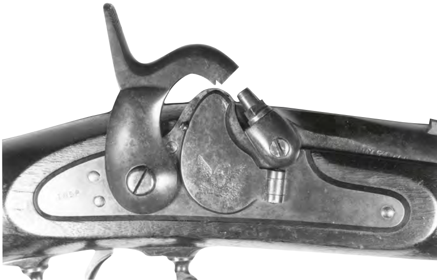
Figure 1. Case-hardened lockplate, hammer, and Maynard Tape Primer cover with stamped eagle and "1858" date, but without "U.S." and "Harper's Ferry" Stamping.
