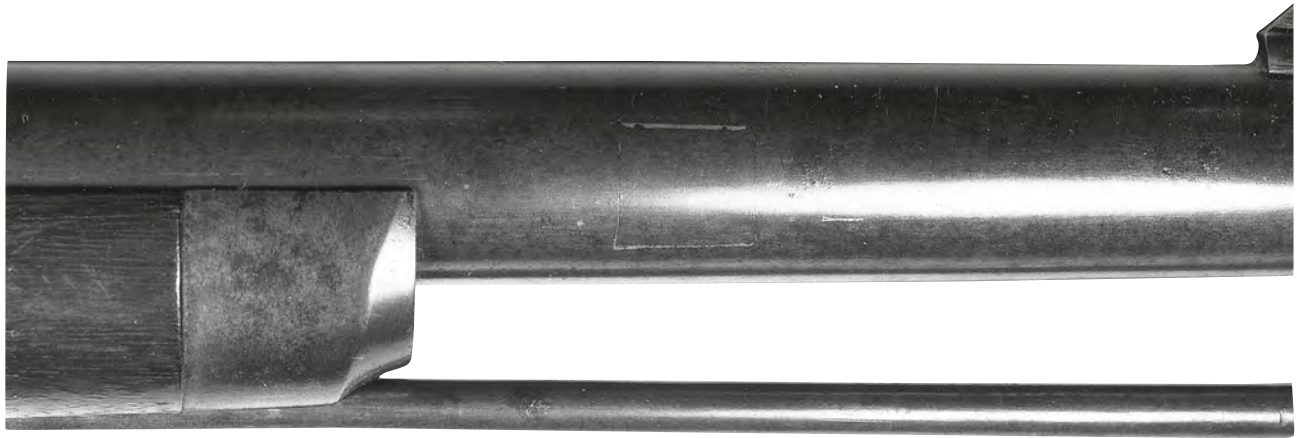
Figure 11. Blued noscap and filled-in mortise.
