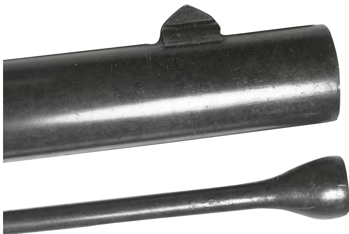
Figure 10. Front sight, end of tulip ramrod, and filled-in mortise-cut which was originally meant for a saber bayonet stud. The filled-in area was polished and browned at the armory.
