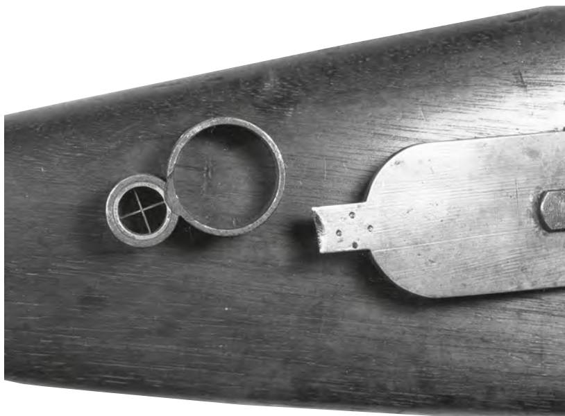
Figure 8A. Double-ring crosshair front sight, lying on stock.
