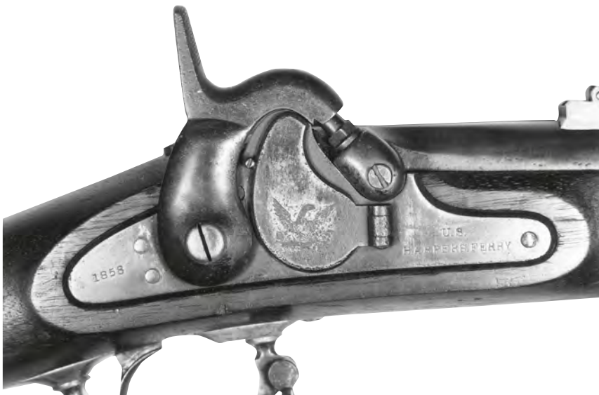
Figure 1A. Lockplate, hammer, and Maynard Tape Primer cover, with stamped eagle. Lockplate stamped "1858 U.S. Harper's Ferry."
