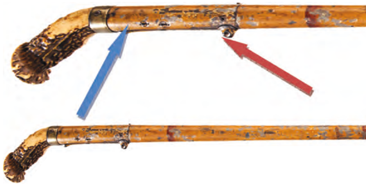
Figure 9. Two views of a cane gun marked "FAIRBANKSPATENT BOSTON." The collar and tip of the gun are made of brass. The simple undercock percussion lock is similar to cane guns made in this country and in England starting in the mid-1820s. The hammer (red arrow) has a hole for a line or ring to facilitate cocking the gun. The trigger (blue arrow) is in its closed and concealed position. The tag grip and faux bamboo painted barrel were popular designs with many makers of cane guns. (Photos courtesy of Matt Parise, Rock Island Auctions.)
