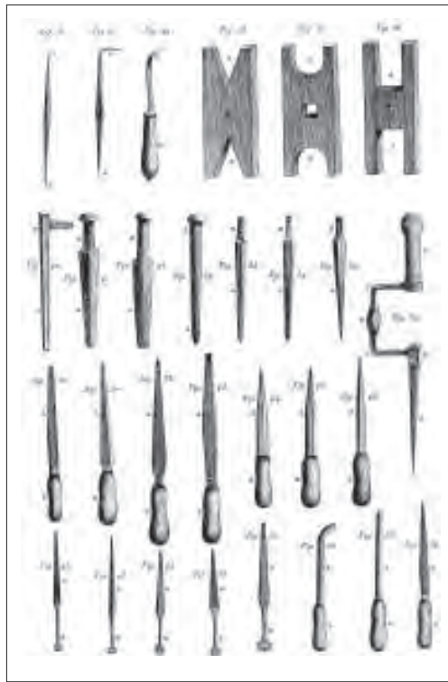
Fig. 13.32 Chisels, files, a brace with drill or reamer and support brackets ? ( chaffe-pommeaux ) from Plate. IX from Diderot on the tools of the Fourbisseur , usually considered a decorator of metals but is accompanied by swords and sword guards.
