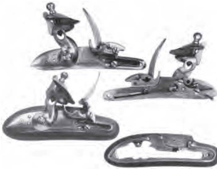
A379abc Fig. 13.36 The 'Musket Lock Jigg' or 'jigger,' produced by Ezekiel Baker for the East India 'Fusil & Carbine Pattern Lock Approved July 1818' It is stamped with 'EB,' the supplier's initials and 'J.L.' These are probably the initials of Joseph Longmore, who in 1817 was a gunlock filer at the Royal Manufactory in Lewisham. David F. Harding collection.
