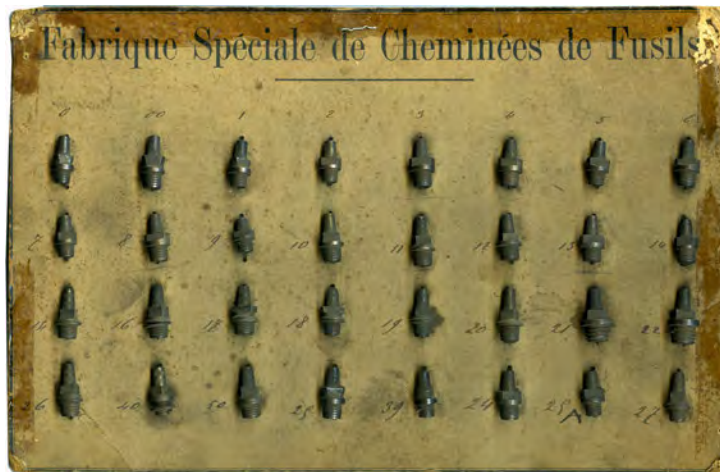
A1.2. A late sample board, probably dating from the last half of the 19th century. The nipples differ in cone length, square shape, vent design and screw thread.
