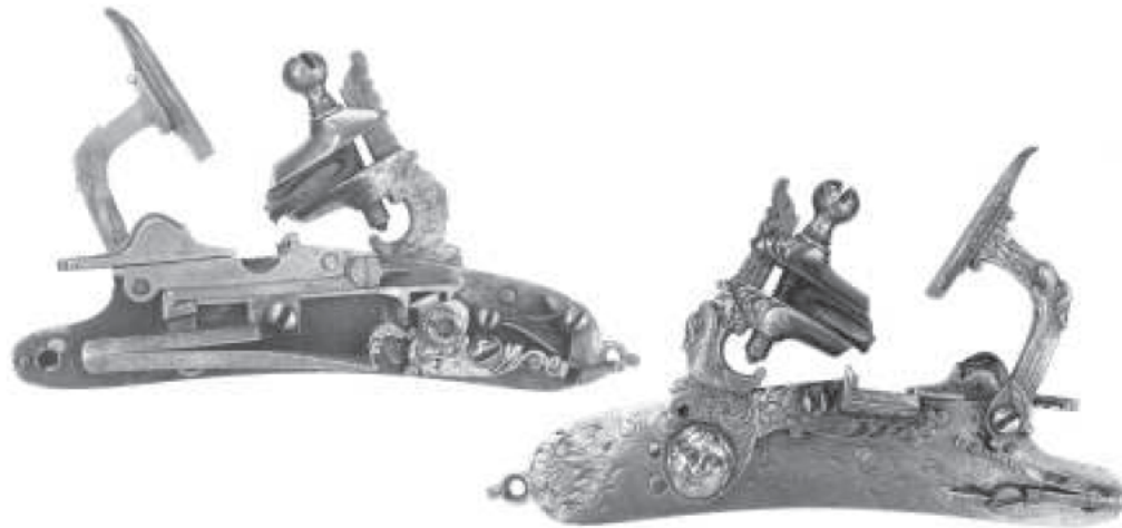
M050 Fig. M050 Fig. Fig. 4.35 An Italian snaphance engraved CZ and dated 1768 on the inside of the plate, under the mainspring. Cassiano Zannotti of Lugo, Emilia and later, Bologna, was born 1706, son of Pietro. He died in 1786. The movement of the pan-cover on the Italian snaphance was accomplished by the same push-bar used on the English snaphance, but rather than being pivoted on the tumbler, it was activated by contact with a lip on the tumbler acting on a catch on the bar. On the majority of locks, the cock was arrested in its fall by a shoulder landing on the bolster of the lock plate but on this one, a buffer is attached under the pan by screws.
