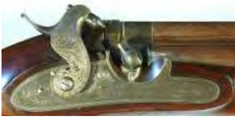
A387Fig.11. The pill lock on a six-barrel “volley gun” by John Thompson of London who was active in 1826. Ross Egles collection.
