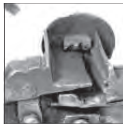
Fig. 10.8-10. A decorative characteristic usually found on Moroccan-made snaphance locks is found on the guide for the pan-cover. The top illustration includes a groove which helps to hold the cover in place when it is closed.
