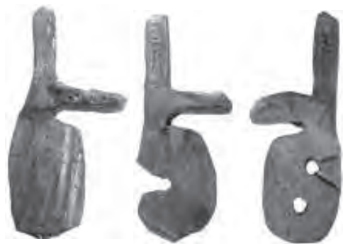
A782 Fig. 13.21 Preliminary forging beginning from a .625 inch (16mm) bar. Left : the bar split for the lower jaw and the body widened with the hand sledge. Center : the stage for swaging or further forging. Time required: less than ten minutes by Lloyd Johnston, Woodville, Ontario.
