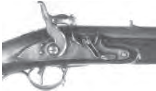
A348Fig.11. William Moore’s percussion tube-lock held a round tube in place by a U-shaped spring-clamp. No patent for this design has been found although it was widely used. This lock was submitted for the Ordnance percussion trials of 1834-1835. FN Royal Armouries Museum – Leeds.
