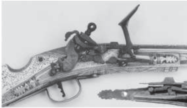
A262 Fig. 4.19 Snaphance lock from a Scottish gun with an engraved brass stock, dated 1624 by James Low of Dundee, and the interior of a similar mechanism illustrating the relationship with the English snaphance. Royal Museum of Scotland collection, Edinburgh No. LH419.
