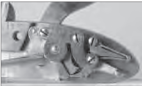
Fig. A1.1. Illustrations of the detent, from the top: the cock at rest showing the detent hidden under the unusual bridle and the mainspring hooked on the swivel of a Samuel and Charles Smith flintlock from a rifle (S/N 4065); the cock at half bent with the sear resting in front of the 'hump on the detent and pushing it to the rear; the cock at full cock position with the detent pushed forward to a position where the sear will be forced to slip over the 'hump' to clear the half-cock bent as the cock falls. [M.133]
