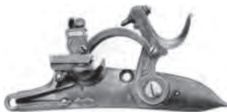
A157 Fig. George John Lacy and Sampson Davis, patent No. 6,046 dated December 6, 1830 claiming "the mainspring outside the lock and making a head fixed upon it act as a striker." It is marked "Davis" on the outside and S. Davis on the inside of the lock. It also bears an inspector-like mark; '6' over a 'crown' over 'SD' over 'Patent.' Robert E. Brooker collection
