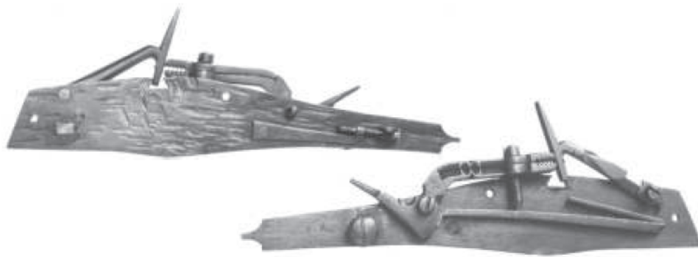
A003 Fig. 4.10. This, the earliest surviving snaphance, is one of 35 muskets made in the government arsenal at Arboga in 1556 which were mounted with Nuremberg barrels. The pan, which is missing, would have had a cover pivoted towards the front requiring it to be removed manually for firing. It would be described as a laglås (lay lock) with an external mainspring. Livrustkammaren, No. LRK16317
