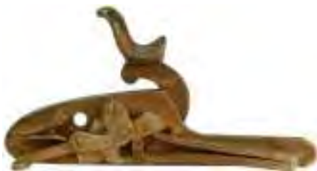
Fig. 12.19 A rebounding lock of inferior finish inside, stamped "Richard." It incorporates Stanton's lengthend mainspring designed to bear against the tumbler to produce the action required to force the hammer to return to the half-cock position. [M263]
