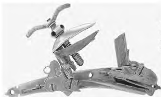
M034 Fig. The Kabyle lock, an Algerian miquelet with brass overlays and engraved dog catch. Dated 1273 A.H. (A.D. 1856) on the lower edge of the lockplate.
