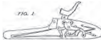
A423 Fig. Everett L. Lake, U.S. Patent No. 289,423, Dec. 4, 1883; Lock for Fire-Arms
