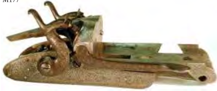
M177 Fig. 12.6 The breech of B.L. double gun with a side lever which, when pressed, lifts the hammers to half cock to allow the firing pins to retract. This design would have appeared after the center fire cartridge became popular about 1862 and before it was superseded by the rebounding lock first patented in 1866. It is marked Beacham's Patent and engraved Perry & Yeld . [M177]
