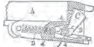
A424 Fig. 12.37. Charles A. King, U.S. Patent No. 412,340, Oct. 8, 1889; Rebounding mechanism.
