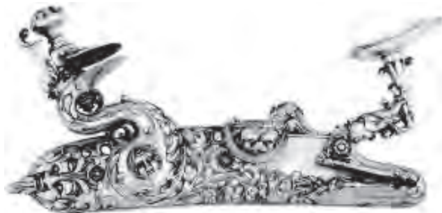
A559 Fig. 4.34 Snaphaunce lock signed and dated 1683 on the inside, by master gunsmith Matteo Cecchi, also known as Acquafresca of Bargi near Bologna, from one of a pair of nearly overly sumptuous silver-and-gold-mounted, ebony-stocked pistols all of Acquafresca's making preserved in the Bayerisches Nationalmuseum collection, Munich.
