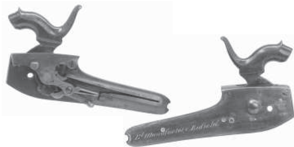
A765 Fig. English percussion lock of George Lovell's first back-action design introduced in 1838. Harold R. Jonah collection
