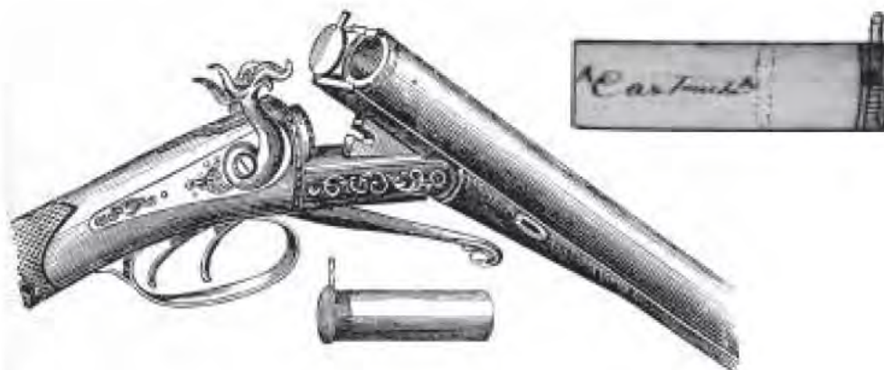
A408 Fig. 12.2 The Lefaucheux breech-loading gun patented in 1833 as illustrated by W. W. Greener in The Gun and its Development in 1888.
