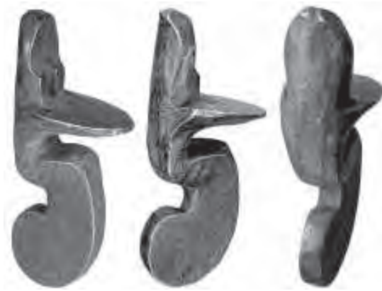
A783abc Fig. 13.12 To quote Charles E. Greener, “A cock of dainty form and proportions would take shape from the forging as if by magic.” This cock was found under one of the work benches at the time the Greener plant on St. Mary’s Row, Birmingham, was closed to provide the space required for a traffic pattern in the mid 1960s. This shape of cock first appeared in the 1780s and continued to be popular until the flintlock period ended. It may have been forged by someone who later became a Greener employee.
