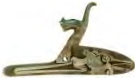
Fig. 12.17. A bar action rebounding locks scroll engraved and "Newark" on the bar of each. They bear the "Stanton Patent Joint Patents" stamp on the inside of the plate and the registration "No. C 12297" on the right and "No. C 12298" on the left. [M223]
