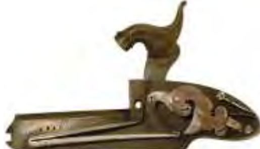
A015 Fig. W. & J. Rigby, Dublin, percussion cap lock with unusually long swivel. Michael McNall collection.
