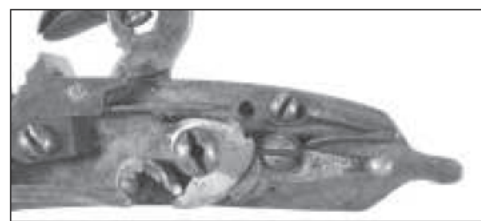
M172 Fig. 4.44 Engraved building A vertical acting sear with a wide ledge to accept the sear nose. Movement of the cock is arrested by the shoulder of the cock.
