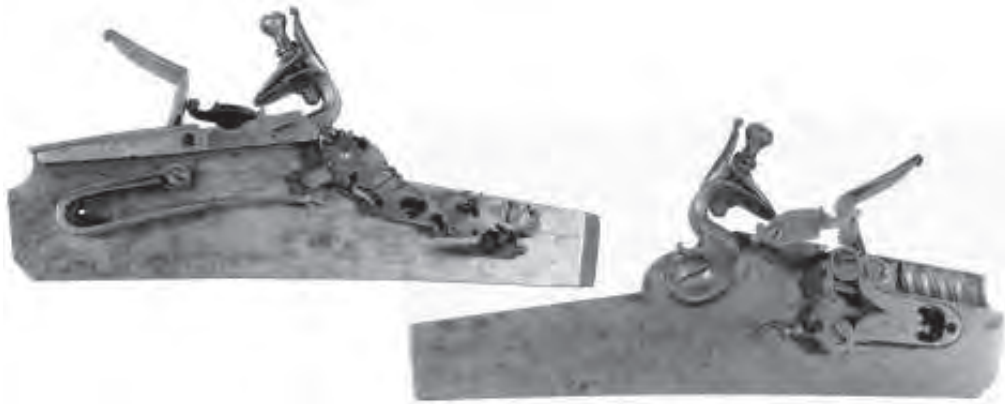
A566 Fig. An unsigned, late 18th century flint-lock. This might be classed as a flintlock as there is a tumbler but the sear rests on the front of a ledge at the top of the tumbler and the action of the trigger pushed the trigger bar forward, lifting the sear nose up. Paul Murray collection
