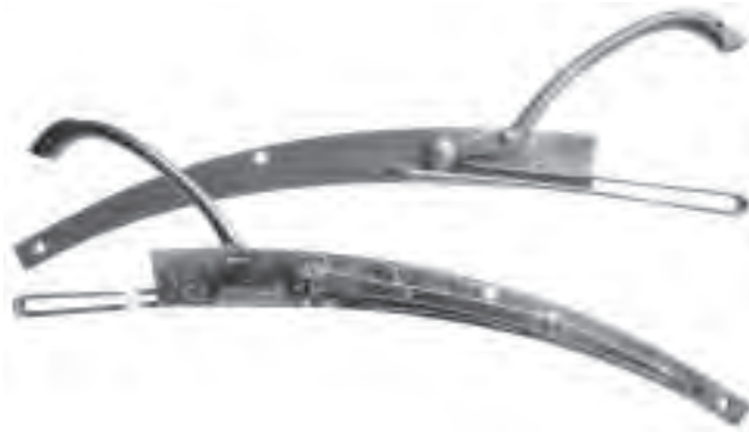
A378 Fig. 2.20 Japanese matchlock with coiled internal mainspring. All components are brass. The lock is held at the rear by a tapered brass pin, which passes through the lockplate and stock into a brass disc set into the opposite side of the stock. The front end of the lockplate is retained by the rear brass barrel band. Bath Royal Literary & Scientific Institution, Bath.
