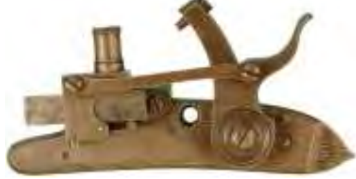
A374Fig.11. This percussion slider lock, probably the basis for Forsyth’s Third Model slider lock, is engraved “Rumford Patent” although no patent in England or on the Continent has been found for it.. [224]
