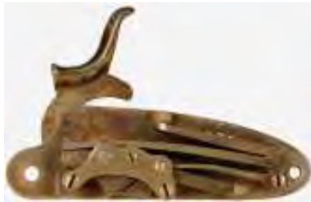
M129 Fig. 12.13 American style rebounding lock with the mechanism behind the hammer is under constant pressure. No patent for this lock has been found but it is from a W.H. Baker & Co. first model front trigger break model double or 3-barrel gun, c. 1875. [M129].
