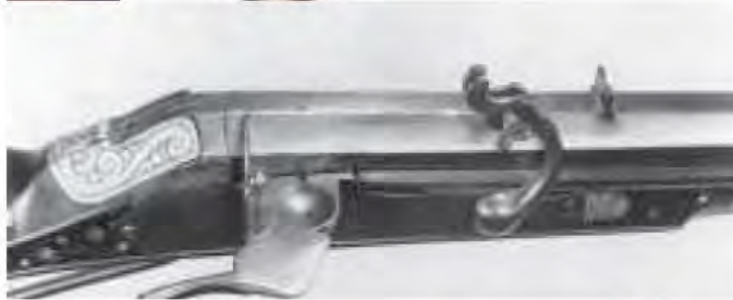
A213 Fig. 2.26. The pan ( bassin in French) and pan cover which forms part of the lock plate, of a late 16th-early 17th century German matchlock. Courtesy Jean René Clergeau.
