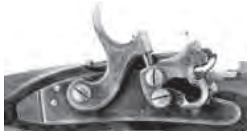
A310a,b. Fig. Joseph Contriner's percussion design with a primer magazine activated by the action of the hammer Plate XXII from Ubhandlung Feuer- und Seitengewehre by Beroaldo Bianchini, published at Vienna 1829. Photograph courtesy G. Charter Harrison.
