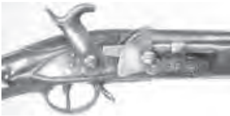
A342 Fig. 6. One of six Thomas Hayward muskets included in the 1834-1835 British trials. The tubular magazine held round percussion pellets. When the hammer was cocked, one pellet was picked up in a cavity in a turning drum and put into position to be struck as the hammer fell. It is constructed on the India Pattern lock. Royal Armouries Museum—Leeds. FN
