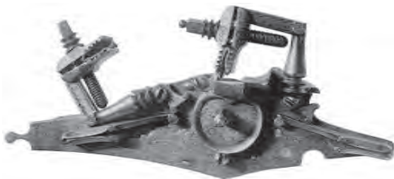
A148 Fig. A double dog lock, possibly Flemish, probably late 16th century. The external wheel is retained by a single screw on the lower edge. Herbert J. Jackson collection. Royal Ontario Museum, No. 925.27.45
