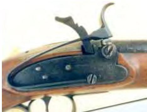
A157 Fig. George John Lacy and Sampson Davis, patent No. 6,046 dated December 6, 1830 claiming "the mainspring outside the lock and making a head fixed upon it act as a striker." It is marked "Davis" on the outside and S. Davis on the inside of the lock. It also bears an inspector-like mark; '6' over a 'crown' over 'SD' over 'Patent.' Robert E. Brooker collection
