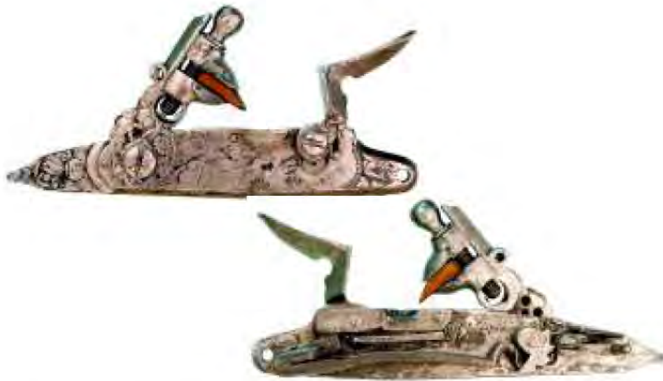
[154] Fig. 6.5 Flintlock of Puype's Type 4, c.1660. Engraved lockplate and cock with floral decoration, a standing dog(?) on the back of the cock, and the signature Mayer á Lyon , a maker who was active 1640-1660. The vertical acting sear is of the two-piece form, a variation of that described by Godwin ( CJAC , Vol. 34, No. 1). [M154]
