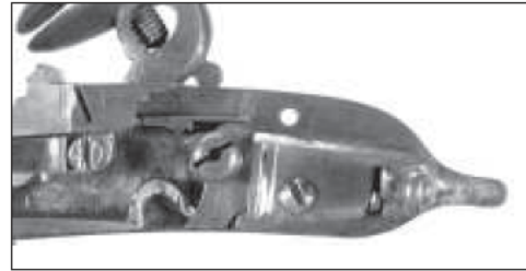
M077 Fig. 4.40 Brento The Tusco-Emellian Box Lock. A two-piece sear held in the engaged position by an additional internal spring. The movement of the cock is stopped by the shoulder of the cock.
