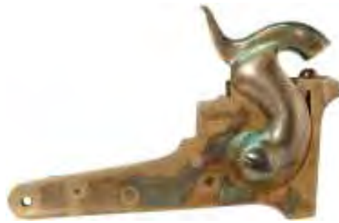
M117 Fig. Sharps' New Model 1859 with the Lawrence primer marked on the plate, C. SHARPS' PAT. / OCT. 5th 1852 and R.S. LAWRENCE PAT. / APRIL 12th 1859 near the primer mechanism,.
