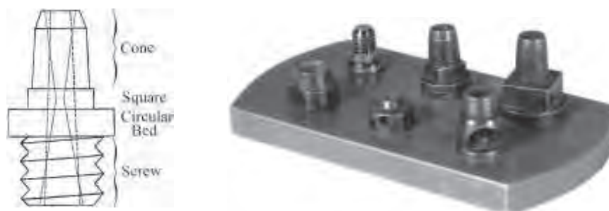
A594 Fig. 11.17 The British military nipple. The dotted line represents the shape of the original vent hole, c.1840; the solid line is that in use in the 1860s. The terminology is that of the Board of Ordnance (to 1855) and thereafter, of the War Department.
