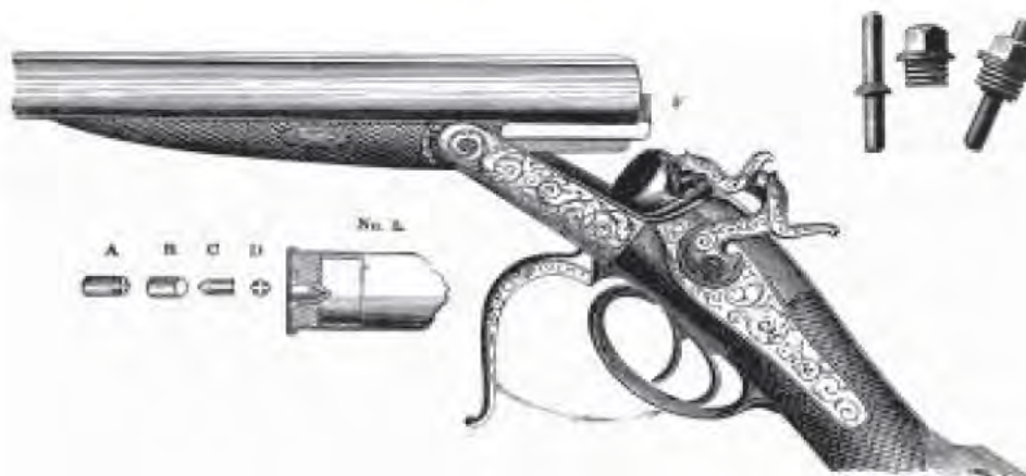
A409 Fig. 12.4 George H. Daw's patent breech-loader with a detail of the cartridge and his primer. The primer components are: A. Cap on anvil, showing the end that rests on the powder; B. percussion cap; C. The Anvil; D. End view of ditto."
