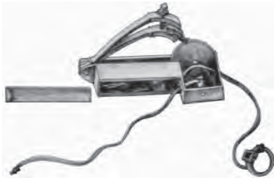
Fig. 3.1. One of the prototype wheel-mechanisms included in the Löffelholz manuscript. There was probably a square end to the axel on the other side of the wheel, and the socket on the ring of the cord would serve to turn both it, and the screw on the dog-head. Staatsbibliothek collection, Berlin
