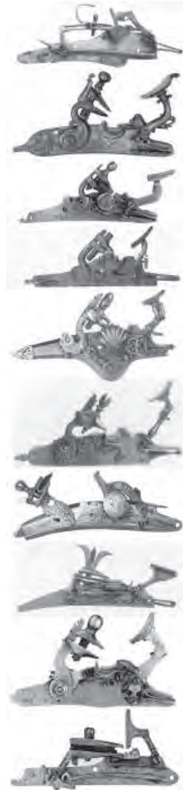
A261 Fig. 4.2 (Left, top to bottom): Snaphance locks by country of origin: Sweden, Sweden, Italy, England, Russia, Italy, Scotland, France; Italy, Russia. All are classed as snaphance but this illustration indicates the great variation of snaphance design. The only feature common to all is the steel fastened perpendicular to the arched steel arm and they are identified by other features; some common, some unique.
