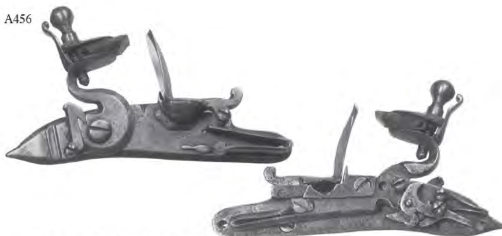
A456 925-27.18 An unsigned lock of slight bannana shape with back ketch or dog and no half cock position on the tumbler. An indistinct mark under the mainspring may be the 'hen' mark of a Suhl gunmaker. This is the prototype of Fig. 8.6. H.J. Jackson Collection, Royal Ontario Museum, Toronto.
