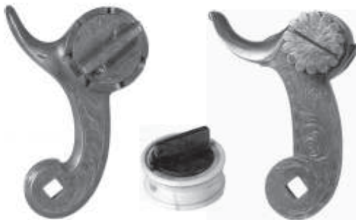
A604-5 Fig. 12.24 A hammer to carry seven pellets [P70] and a spare magazine in a bone case by Isaac Riviere of London, and a similar one by Thomas (?) Sykes of Sheffield to hold six pellets. Both are engraved with the maker's name and "Patent" but no patent has been found to cover them.
