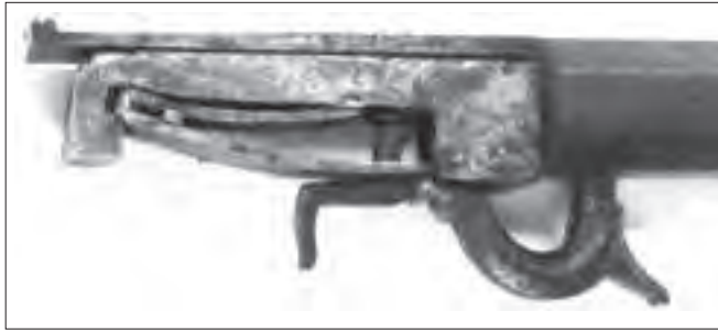
A588 Fig. 11.21 It is believed that the U.S. patent granted to Fordyce Ruggles in 1826 but lost in the Patent Office fire in December 1836, covered the underhammer ignition illustrated here. Nicholas L. Chandler collection
