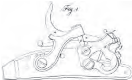
A310a,b. Fig. Joseph Contriner's percussion design with a primer magazine activated by the action of the hammer Plate XXII from Ubhandlung Feuer- und Seitengewehre by Beroaldo Bianchini, published at Vienna 1829. Photograph courtesy G. Charter Harrison.
