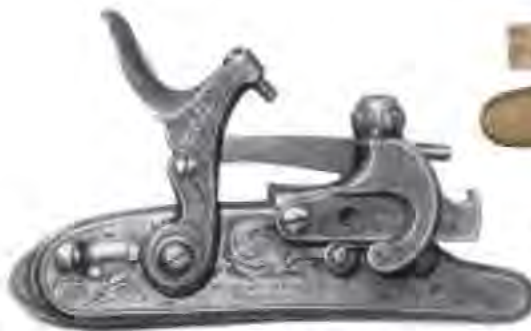
A068 Fig. 11.6 Forsyth's slider lock introduced prior to 1812. Musée d'Arms collection, Liège
