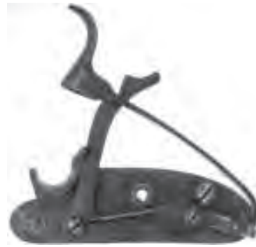
A157 Fig. George John Lacy and Sampson Davis, patent No. 6,046 dated December 6, 1830 claiming "the mainspring outside the lock and making a head fixed upon it act as a striker." It is marked "Davis" on the outside and S. Davis on the inside of the lock. It also bears an inspector-like mark; '6' over a 'crown' over 'SD' over 'Patent.' Robert E. Brooker collection
