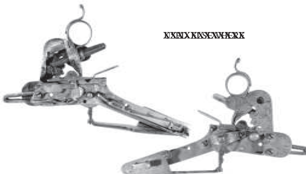
A569 Fig. An unsigned but lightly engraved lock of a Silesian Tscinke dating from the last half of the 17th century. The name is derived from Teschen, the village where this form of lock was produced. Paul Murray collection.
