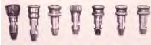
A019 Fig. 11.12 “Noses for Hall’s patches.” credit for improving Hall’s hammer is given to Thomas Cartmell of Doncaster by W.H. Wallaston, supplier of platinum to the gun trade. Keith R Dill collection.
