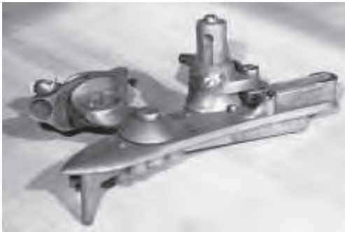
A309 Fig. An experimental military conversion with a sliding pan cover containing a percussion nipple, held in place by a thumb-screw, and a reversible combination top jaw and hammer, held by the flint screw, illustrated in Ubhandlung Feuer- und Seitengewehre by Beroaldo Bianchini, Vienna, 1829. Photograph courtesy Musée d'Arms, Liège.
