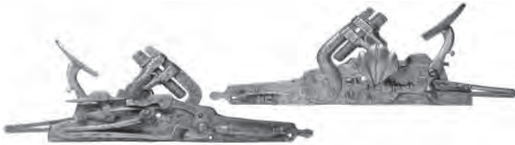
A454 Fig. 4.25 A Dutch snaphance of c.1620 with a straight lower edge and the typical hump back. The pan has a fluted shell shaped fence with engraved lines and the sliding pan cover has an enlarged ridge which provides a thumb rest to ease closing the pan. The swing-over safety. The design and mechanism is identical to the typical English snaphance. The frizzen may be a replacement. Herbert J. Jackson collection, Royal Ontario Museum, No. 925.27.19
