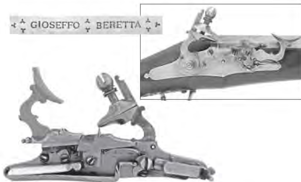
A554 Fig. 4.45 Brescia, 1660-80, mounted on a large (20 inch/51cm) holster pistol by Giovan Antonio Gavacciolo with a barrel by Giovan Antonio Beretta, a linear ancestor of today's Franco and Pietro Beretta. It has a conventional tumbler and sear with an early form of bridge. The chiselled motifs are unusual and exactly match those of a snaphaunce fowling piece, presumably part three of a trio. Private collection, Italy.
