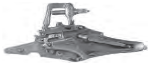
A209 Keld 1931 Italian Wheel Lock mechanism from a heavy gun ca. 1580 Keld Weigelt collection
