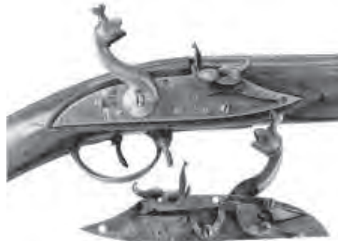
A225 Fig. One of a small group of snap matchlocks with an automatic frizzzen-like pan cover. Made by Muhammad Ali, one of the gunmakers working at Seringapatam for Tipu Sultan in 1797/78. The pan cover is fitted with a roller bearing which rides on a standard frizzzen spring. When the trigger is pulled, the serpentine is rotated downwards by the pressure of the trigger finger. The movement of the tumbler, through the linkage, also cantilevers the pan cover open. When the trigger is released the serpentine returns to the upright position under pressure of the sear spring. The pan cover may then be operated manually. Courtesy Robin Wigington
