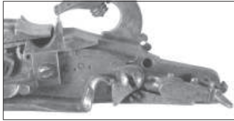
A558a-f M044 Fig. 4.39 C.O. A lateral acting sear working through the lockplate to engage a notch on the back of the cock. The movement of the cock is stopped by a buffer forming a part of the pan.
