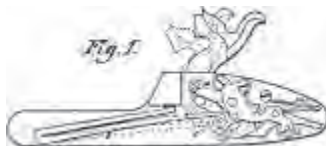
A421 Fig. John A. Nichols & Joseph W. Livingston, U.S. Patent No. 198,669, Dec. 25, 1877; Gun Locks.
