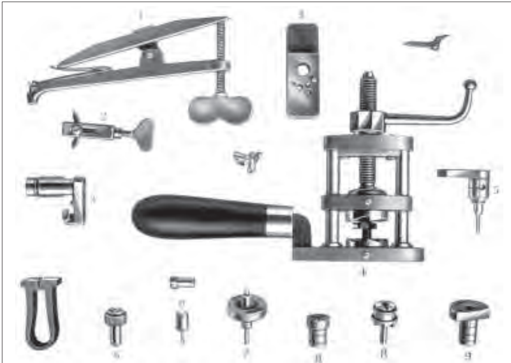
A044 Fig. 13.34 “Old gun lock filers’ tools.+ 1, 2. Spring Cramps; 3. Swivel Plates; 4. Stocks with Die; 5. Peg Grinder; 6. Wheeler; 7. Pivot Brush; 8 Levellers; 9. Oval. Illustrations from Gun-making Handicrafts by Charles O. Greener, 1925.
