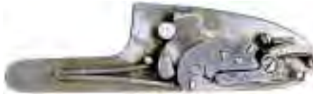
Fig. 12.22. A high quality seven pin bar action side lock with intercepting (double) sear, 'in the white' as made ready for sale to the gunmaker. The lump on the internal hammer (tumbler) is for the cocking rod to push on when the gun is opened, thus cocking the action. [M250]
