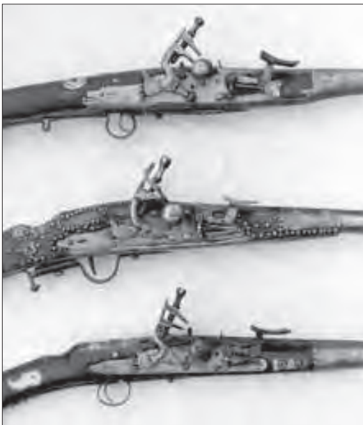
Fig. 10.6. The Barbary lock found on these 18th or 19th century Moroccan muskets is physically and mechanically identical to the English snaphance of the early 17th century. Very few Moroccan arms are dated and they were still in use in the 20th century. The Gordon T. Howard collection, The Stewart Museum, Montreal.
