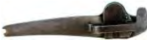
M118 Fig. William Jenks of Columbia, South Carolina obtained U.S. Patent No. 747 in 1838 for a side-hammer lock for a breech loading firearm. This, from a carbine of 1847 with a Maynard primer is stamped 'Remington' over 'Herkimer' over N.Y. on the plate and '587' on the hinge of the magazine cover. [M118. see also M163]
