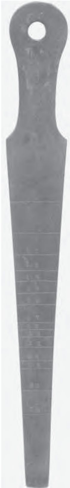
A692-3 An English, iron bore gauge. forged by an unknown smith with the initials 'RS.' It has the fractions in Imperial on one side and Bore sizes on the other.
