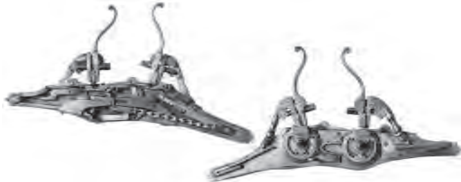
A134 Fig. A double wheel, lock which is probably from a gun designed for superimposed loading but there is a slight difference in the level of the two pans which might have served a double barrel, over/under gun. There are no marks but lockplate shape suggests south German of the late 16th century. Herbert J. Jackson collection . Royal Ontario Museum , No. 925.27.30
