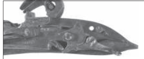
M110 Fig. 4.42 Bramanti A one-piece vertical sear operating in the manner of the flintlock to engage a broad step on the tumbler but no half-cock.
