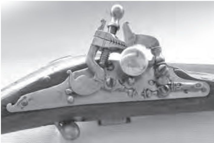
A291 Fig. 4.9 A small English snaphance pistol, c.1615. The barrel, lockplate, and pan are brass. The tail of the plate has the typical English monster hear form Palazzo Ducale collection, Venice.
