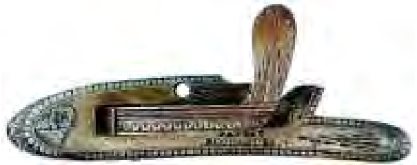
M220 Fig. Mule-ear pill or punch lock by Ephriam Gilbert covered under the Name & Date Patent April 3, 1829. Stamped (partially under hammer) E. Gilbert Patent Rochester. [NY] and inside the plate with the number 876. [M220]
