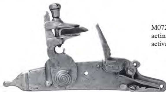
A456 925-27.18 An unsigned lock of slight bannana shape with back ketch or dog and no half cock position on the tumbler. An indistinct mark under the mainspring may be the 'hen' mark of a Suhl gunmaker. This is the prototype of Fig. 8.6. H.J. Jackson Collection, Royal Ontario Museum, Toronto.
