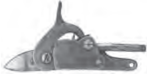
A341 Fig. 5. In 1832, the gunsmith Thomas Hayward of Winchester submitted a percussion magazine which Blackmore records “was considered by Lovell to be the best of the magazine locks.” It is believed that this is the prototype constructed on an India Pattern lock shown to Lovell at that time. [M174]
