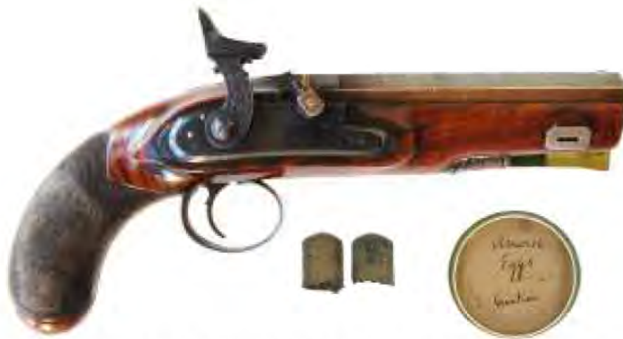
A340 Fig. 11.14 What may be the first, certainly one of the first, pistols fired by percussion cap is that illustrated here. It was made by Joseph Egg and is engraved Joseph Egg / By permission of Forsyth the Patentee on the lockplate. It is little different from locks of the period and internally is identical to the flintlock. Externally, the obvious changes included the replacement of the flint cock with an early form of hammer with a flat nose, and of the pan and frizzen by a drum and nipple to receive the percussion cap. South Somerset Museum, Yeovil, England.
