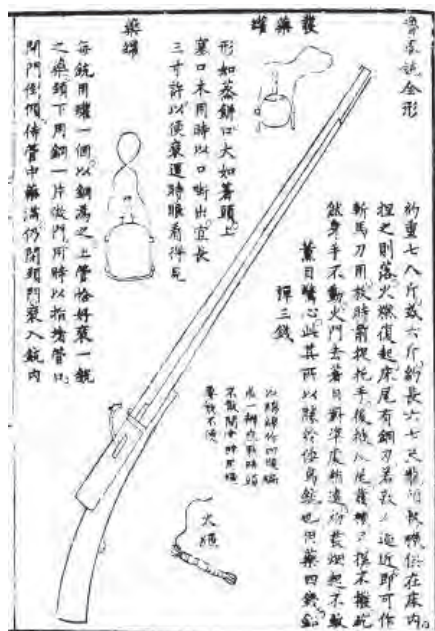
A705c Fig. 2.13. (left) The translation of the text accompanying the illustration provided by Chao Shih-Chên in his 1598 Handbook records that it is of Turkish origin which “on pressing the trigger, the cock falls, and after ignition it rises again....When firing one should only squeeze the trigger, not pull it, ...the touch-hole is slightly further away from the place where the eye takes aim (than in the case of the Japanese bird-beak gun), and hence the smoke and flame developed when the musket is fired affects the eye and startles the musketeer less. Needham, Fig. 174.
