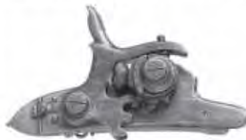
A147 Fig. TWO VARIATIONS OF ELZECKEL DAKER'S STRIKING PAN for combination flint and percussion ignition introduced in 1821. The left with pill, ex W. K. Neal collection [M216], the right with percussion cap. ex Herbert J. Jackson collection .
