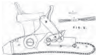
A595 Fig. 11.27 Joseph Manton’s Patent No. 4,285 dated July 22, 1818 was the first serious competition to Forsyth’s patent. It covered the primer and a clamping arrangement to hold a tube primer “placed in a grooved pan at right angles to the touch-hole,” perpendicular to the barrel with one end entering the vent. It continued to be popular among some sportsmen until into the 1880s.
