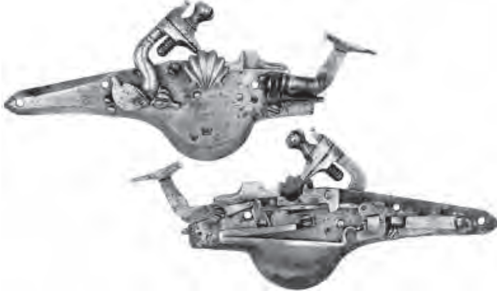
A499 Fig. 4.26 A Dutch snaphance of the second quarter of the 17th century from a pistol. The lockplate with wheel profile is flat with chamfered edges marked with the initials 'W S' surmounted by a crown; the cock is round with a flat base as found on English snaphance of the previous century. The fence is in the form of a fluted shell. Henk L. Viser collection, No. HV-79.
