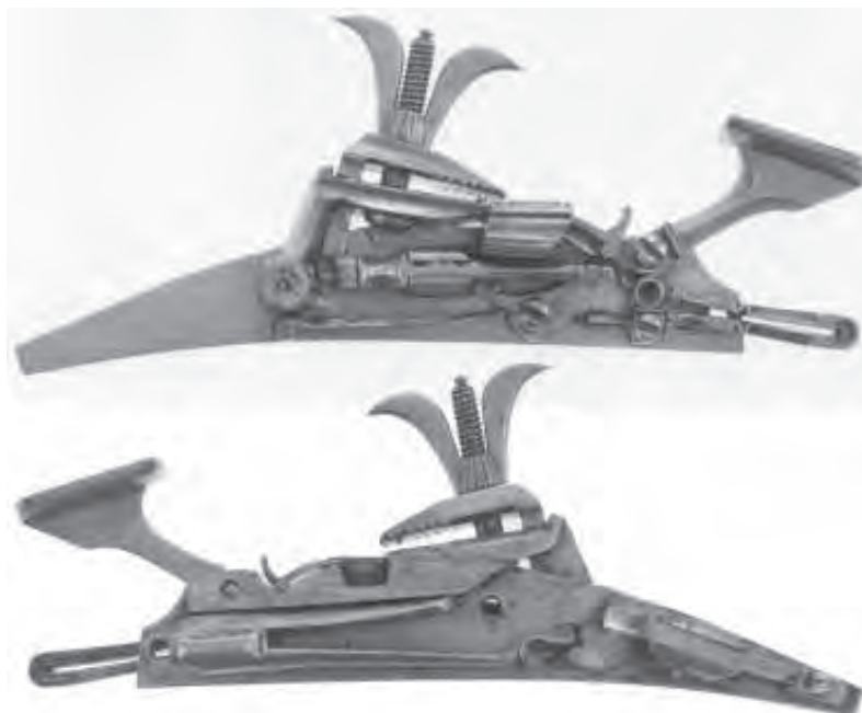
A038 Fig. 4.20 The Roberts snaphance lock mounted in pistol with a Nuremberg town-mark on the barrel. Royal Armouries Museum collection,
