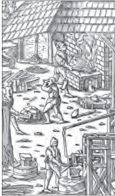
A761 Fig. 13.7 A water-powered hammer (lower right corner) being used to shape the beat the slag from wrought iron illustrated by Georgius Agricola in De Re Metallica , 1556.
