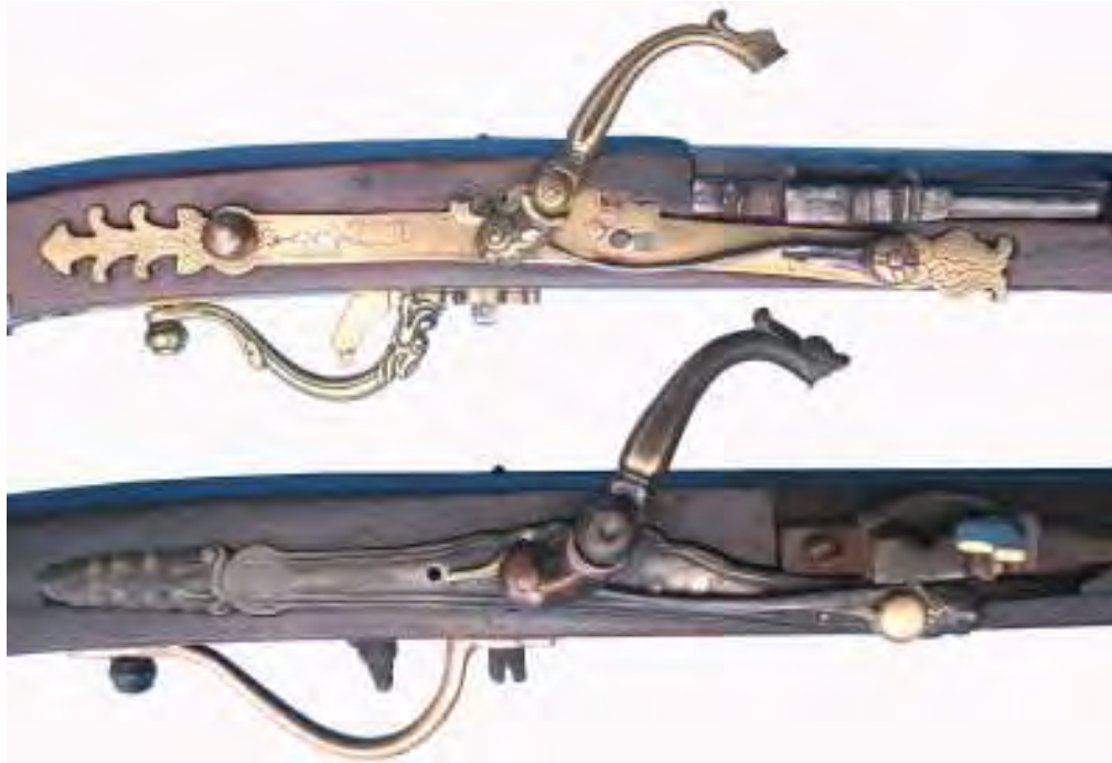
Fig. 2.22, 23. Two Vietnamese matchlocks with brass lockplate and serpentine. The external mainspring producing upwards pressure on the tail of the serpentine provided the action. Courtesy Oriental Arms, Haifa.
