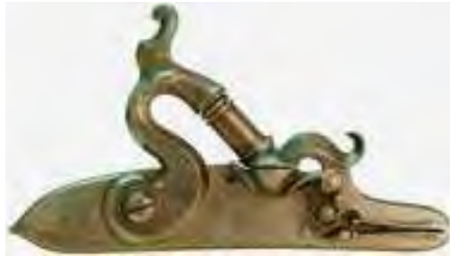
M158 vPercussion pill lock made to Jean Lepage's French patent of June 23, 1810. It is a single shot and does not have a primer magazine suggesting that it is only a slight variation of the ignitions covered in that patent. [M158, M207]
