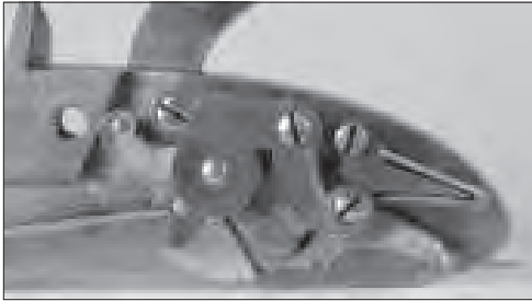
Fig. A1.2. Ezekiel Baker called this his 'solid shank' to give greater strength to the square of the tumbler and secured the cock with a 'washer-screw,' also known as a tumbler button, bunn nut or burr.
