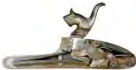
M243 Fig. 12.18. Rebounding lock, in the white, by Charles E. Sneider of Baltimore based on U.S. Patent No. 149,353 dated April 7, 1874. Stamped on exterior and interior, Sneider over Baltimore [M243]
