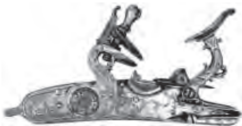
M172 Fig. 4.36 An unsigned, Tuscan snaphance engraved with vines on the cock, steel arm, and lockplate in front of the cock and behind the cock, with a bulding probably a residence.
