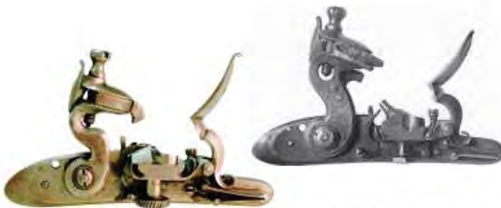
A147 Fig. TWO VARIATIONS OF ELZECKEL DAKER'S STRIKING PAN for combination flint and percussion ignition introduced in 1821. The left with pill, ex W. K. Neal collection [M216], the right with percussion cap. ex Herbert J. Jackson collection .
