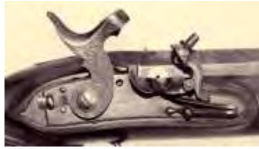
A403 Fig.11. Joseph Manton flintlock converted by replacing frizzen with a combination nipple/pan cover. This plan was used frequently by Manton. Paul Murray collection
