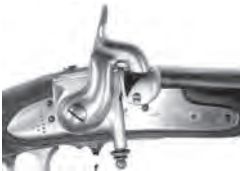
A112 Fig. American military experimental lock fitted with Butterfield's priming system. Stamped in front of the hammer Butterfield's Patent Dec 11 1856 Philada and Harpers Ferry and the date 1859, only the last digit of which is clear. U.S. Military Academy Museum.
