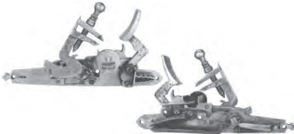
M101 Fig. A late 18th to at least the mid 19th century, snaphance with flat surface profile and fragments of a silver inlay. This lock is otherwise undecorated but of better workmanship than most.
