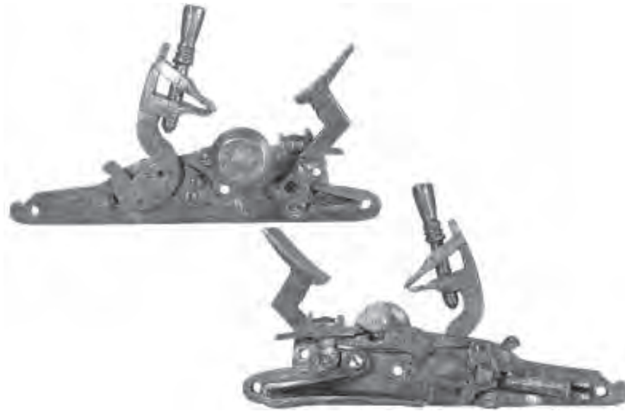
M273 Fig. 10.11. Barbery locks. This lock may have a Muslim provenance suggested by the unidentified marks and brass inlay on the flash guard, but everything else about it is English c.1610-30. Before the end of that century and into the next, many thousand Barbery locks were exported to north Africa. (Chapt. 4, Fig. 4.46).
