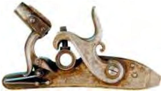
A336 Fig. 11.9 An early pill or powder lock by John Jones of Birmingham which would have been made prior to 1815. He produced a number of them and sold some but in 1815 he moved to Russia to take over as superintendent of the government arsenal at Tulla. Some of those that he did not sell have been installed in existing gun and engraved with a popular gunmaker's name [073]. FN
