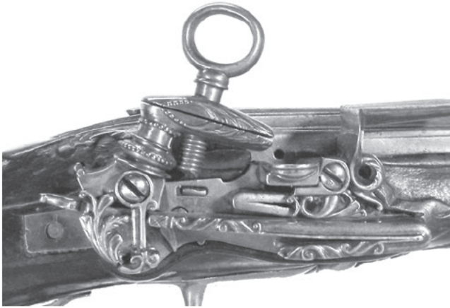
A572 Fig. A mid 18th century, unsigned Austrian miquelet of patilla configuration, with upward pressure on the tail of the cock, and the foot resting on the half cock stop. The square tail on the lockplate is typical, the filed decoration is superb. The barrel is stamped Lazarino Cominazzo , the famous Italian barrel making family. Paul Murray collection
