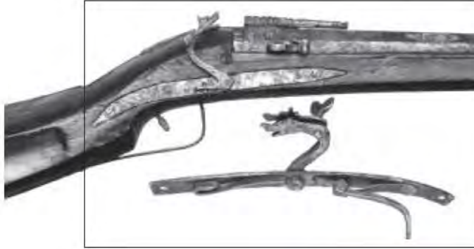
A089 English military snap-matchlock of Ventian manufacture, c.1550.
