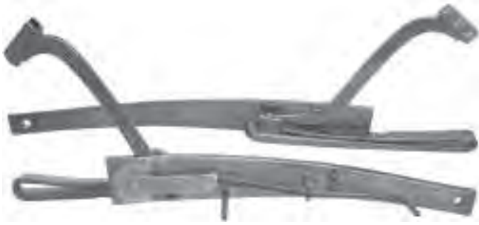
A377 Fig. 2.19. Japanese matchlock (Tanagashema) with a hammer hardened brass external mainspring and an iron sear. Brian C. Godwin collection.
