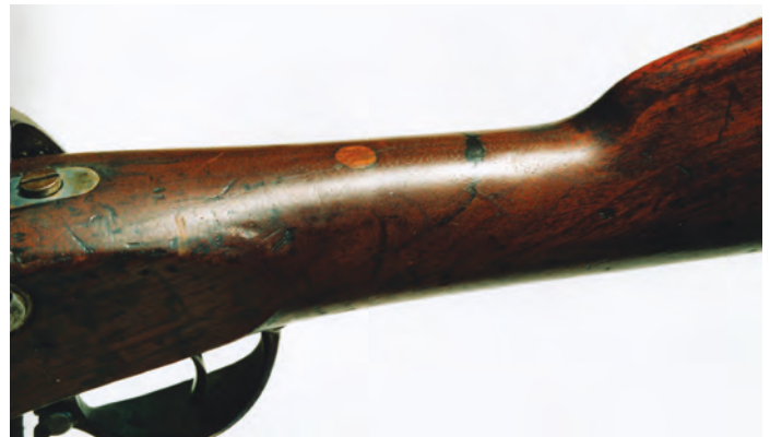
Figure 23. 1862 dated Mason musket showing probable factory repair of wrist crack. (Author's Collection)
