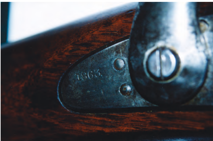
Figure 19. Example of the occasional 1863 lockplate stamped off the centerline. (Author's Collection)
