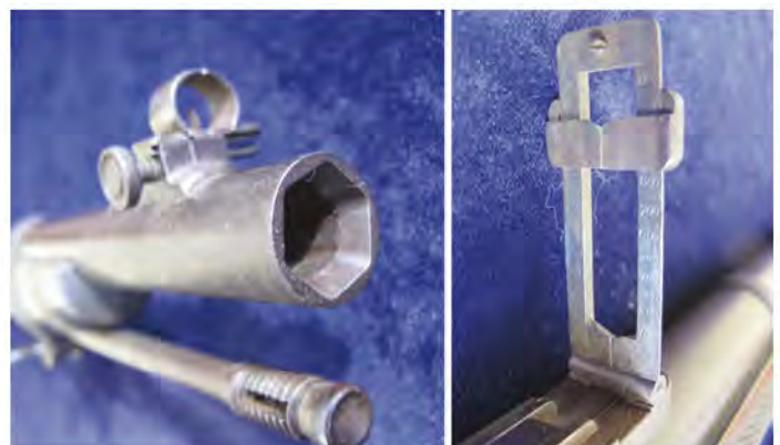
Figure 61. Whitworth countersunk muzzle with hexagonal bore; rear sight graduated to 1,200 yards.
