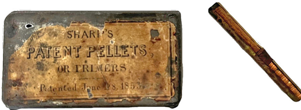
Figure 13. Primer tube for Sharps Automatic Priming System and Tin Box containing Tubes of Primers for the Sharps.
