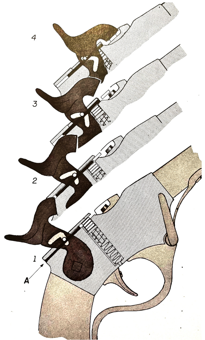
Figure 5. Action of the Sharps Patent Automatic Priming System displaying the linked plunger driving a percussion priming pellet from the magazine to a position over the cone nipple as the hammer falls. (Diagram reprinted from The Gun Collectors Letter No 15, 21 August 1947, p 73).
