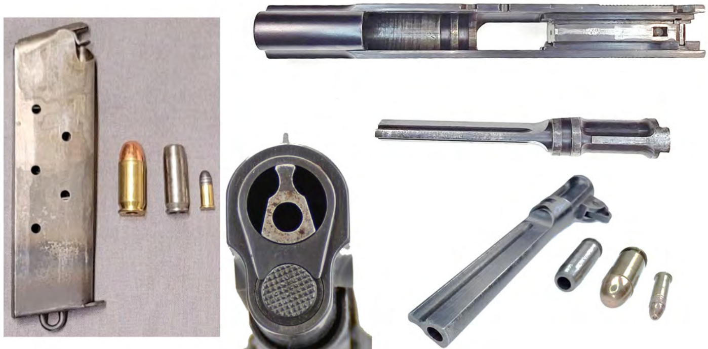
Figure 5. First Type magazine and cartridge adapter; the adapter is the silver object between the standard .45 and .22 cartridge (left); barrel and slide (top right); barrel, adapter and bullets (bottom right) and muzzle configuration (center bottom).
