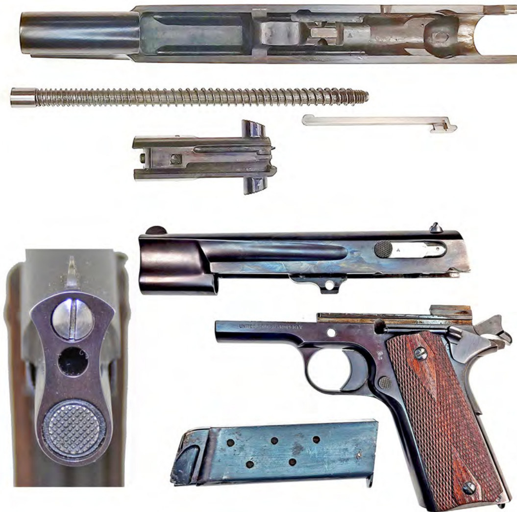
Figure 8. Second Type M1911 reciprocating bolt, recoil spring, ejector and non-reciprocating slide (top), muzzle configuration (bottom left) and receiver, modified magazine, and slide.
