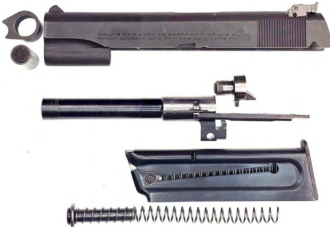
Figure 16. Service Model Ace components also referred to as the ‘Williams Pistol’. Note the floating chamber at barrel breech.
