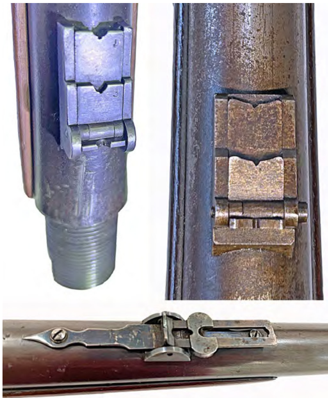
Figure 11. Rear sights on Muzzy made military-configured carbines serial number 60 (top left) and serial number 54 (top right) compared to rear sights on Muzzy made civilian carbine barrels (bottom) such as this one, serial number 86, Ralph Spears collection.
