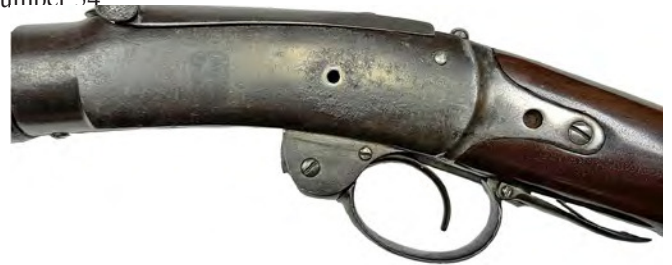
Figure 9. Left side of the receiver for carbine, serial number 60, showing holes where a sling bar would have been originally mounted. Photo by John Dietrich, Courtesy of the Museum and Library of the Confederacy, Greenville, South Carolina.
