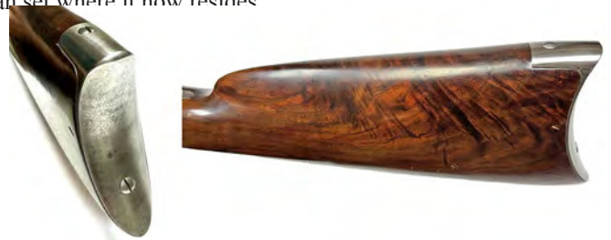
Figure 10. Buttstock and butt plate of military-style carbine, serial number 60, showing atypical characteristics suggesting a later replacement. Photos by John Dietrich, Courtesy of the Museum and Library of the Confederacy, Greenville, South Carolina.
