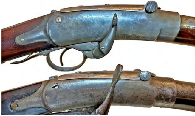
Figure 7. Right side views showing variations in the cocking hammer: serial number 54 (top) has the same size and shape cocking hammer as civilian Morse-Muzzy receivers. Also, like civilian receivers, the end of its hammer and finger buttons are checkered (author's collection); serial number 41 (bottom) has a longer cocking hammer not seen on any other Morse-Muzzy receiver. Its cocking hammer and finger buttons are both without checkering (author's collection, formerly Jim Reid collection).
