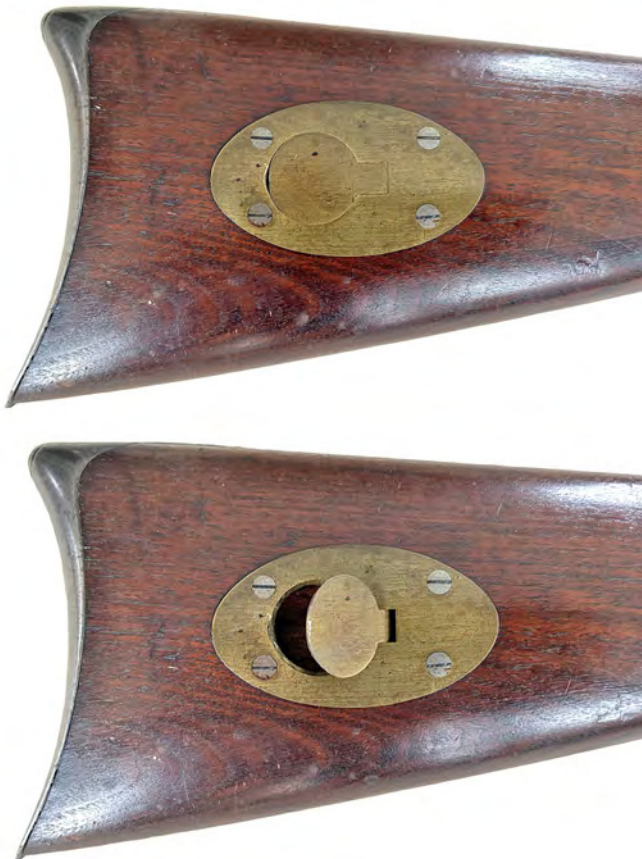
Figure 8. Patch box on Morse-Muzzy military-configured carbine, serial number 54, closed and open.
