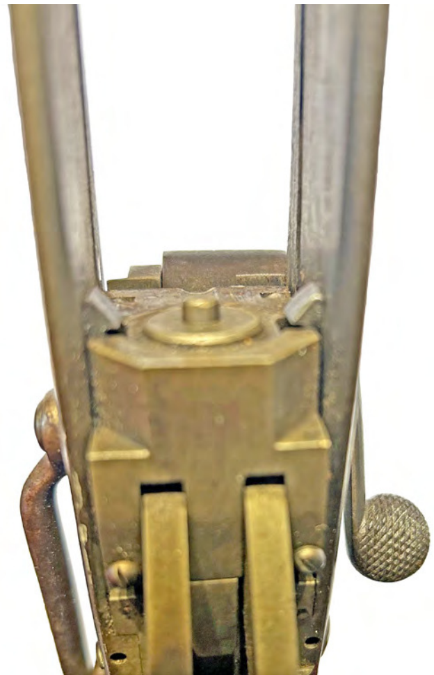
Figure 4. Morse cartridge extractors (author's collection, serial number 54).
