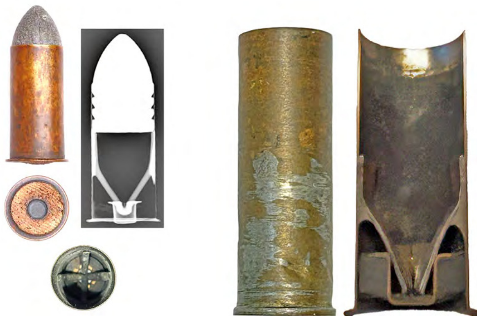
Figure 3. The key components of the Morse cartridges built based on Morse's Patent #20727 illustrated using photographs, X-ray and a side-view cut-out. These illustrations show the details of a Morse patent centerfire cartridge including the three key components (1) a centered primer surrounded by a gutta-percha or similar washer in the base of the cartridge case, (2) a cup-and-anvil to hold the centered primer when it is stuck by the firing pin, and (3) a flange at the base of the cartridge enabling the engagement of "nippers" on the face of the bolt in the automatic extraction.
