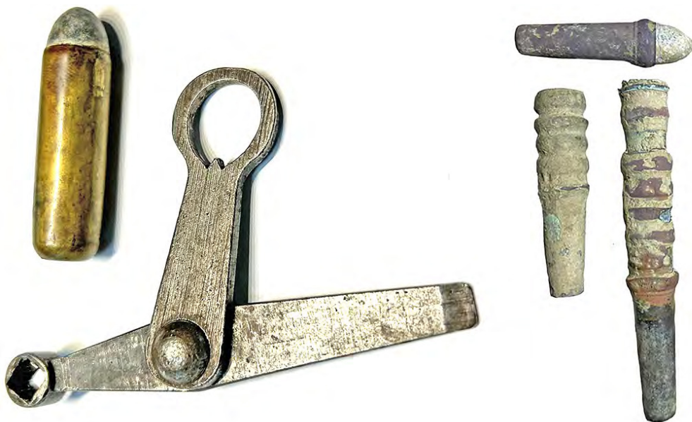
Figure 5. Left - Gallagher carbine extraction “wrench” tool the soldier had to carry with him in his pocket or cartridge box to order to extract a spent cartridge by the hand not holding his carbine (author’s collection). Right - Burnside carbine extraction ad-hoc “tool”: five and ten spent cartridge cases stacked together as an ad-hoc extractors by inventive soldiers (example of ten in author’s collection, formerly in the Dean Thomas collection).
