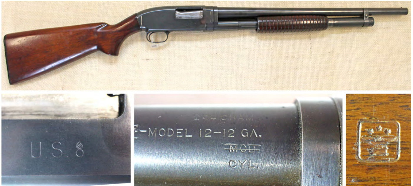
Figure 21. Winchester Model 12 riot gun serial number 976670. Most riot guns were manufactured prior to the trench guns. This early gun has a 41-dated barrel which had “MOD” struck out and “CYL” added when the factory shortened the barrel to 20 inches. As it does not have the usual “W.B.” final acceptance stamp, the stock is most likely an unmarked replacement to which someone added the postwar Defense Acceptance Stamp to make it look more authentic.
