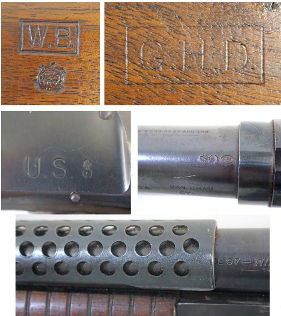
Figure 9. The World War II Winchester Model 97 trench gun has several features that are different from its World War I parent: it is takedown, has a shorter fluted comb and thicker wrist military-inspected buttstock, has factory-applied military markings on the receiver and the 20-inch barrel end extends beyond the bayonet lug. World War II Model 97 trench guns are found in the E921300 to E986300 serial number range. 22 This gun, serial number E927878, is one of the guns delivered on the November 1941 contract. The key identifying features are the serial number, the 42 barrel date, the boxed W.B. inspection stamp, and the six-hole heat shield which was changed early on to the more common Winchester World War II four-hole configuration. The buttstock has a hard rubber buttplate with the Winchester logo and is inspected on the left side with the boxed W.B. over the “crossed cannon” Ordnance Department stamp. Most World War II Winchester trench guns have the later boxed G.H.D. inspection mark. The lower left rear of the receiver is factory-marked with a large “U.S.” followed by the Ordnance Department bomb. The top center of the barrel just forward of the receiver has the Winchester proof mark and the ordnance bomb stamp.
