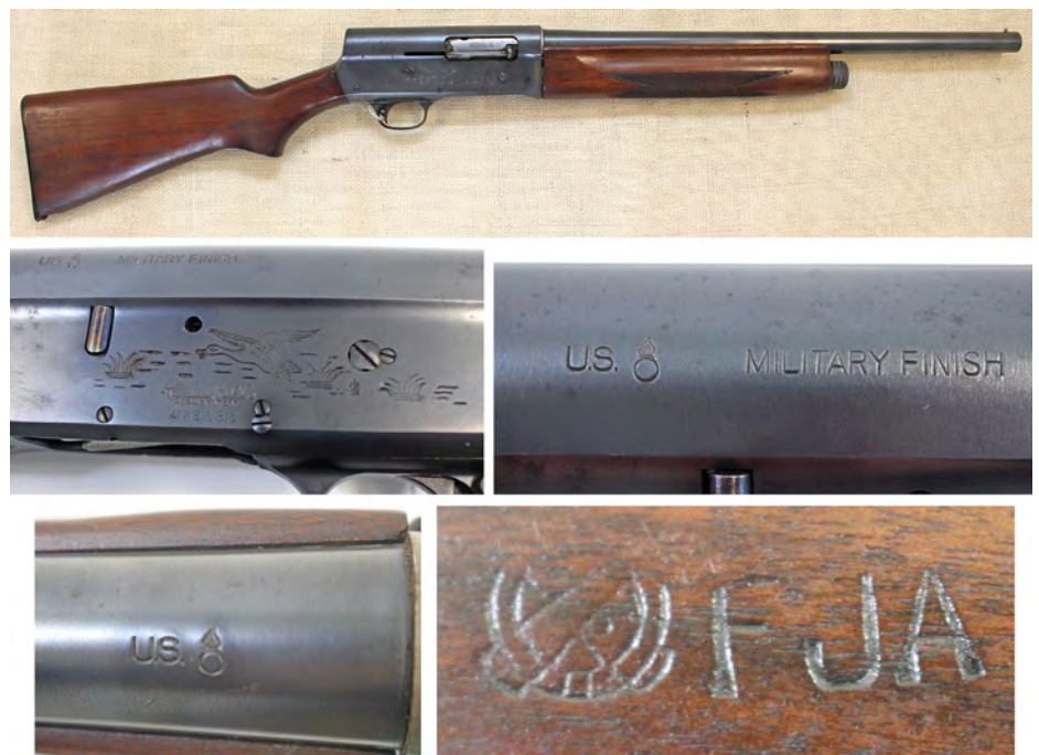
Figure 15. Remington Model 11 riot gun serial number 478386 with early features. It has the commercial checkered forend and game scene on the receiver. The matching barrel is dated May 1943. The bolt is marked “MODEL 11”.
