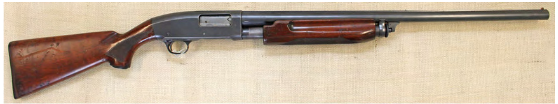
Figure 26. Remington Model 31 skeet shotgun. This is a typical example of an early World War II training shotgun purchase. This Model 31, serial number 39967, is a commercial gun with a solid rib and 26-inch Improved Cylinder choke barrel. It is stamped "RLB" and "flaming bomb" on the receiver.
