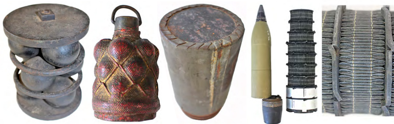
Figure 2. Artillery projectiles. An unfired U.S. stand of “grapeshot” for 12-pounder guns with a 4.62” bore. These were commonly used as naval rounds to destroy ship’s rigging and were mostly obsolete by the Civil War. However, some have been found at Civil War sites. The second is a stand of 1.5” quilted grapeshot. The third is an unfired U.S. 4.62” 12-pounder smoothbore canister widely used as an anti-personnel round. The thin-walled canister contains many lead or iron balls, which are much smaller than grapeshot, packed in sawdust. The canister bursts upon firing and the balls spread. The fourth is a Vietnam War era U.S. 105mm “Beehive” anti-personnel canister round designed and used for direct fire on enemy troops. Several of these rounds were placed with each cannon for quick reaction direct fire. They used 8,000 tiny steel dart-like flechettes, ejected by a mechanical time fuse. Flechette rounds with similar small darts were also used in 12-ga. combat shotguns, 40mm grenade launchers and 90 and 152mm rounds during the Vietnam War.
