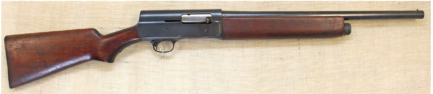
Figure 17. Remington Model 11 riot gun serial number 491019. This can be called the standard World War II configuration as it has no game scene on the receiver and plain stocks. The matching barrel date is July 1943.
