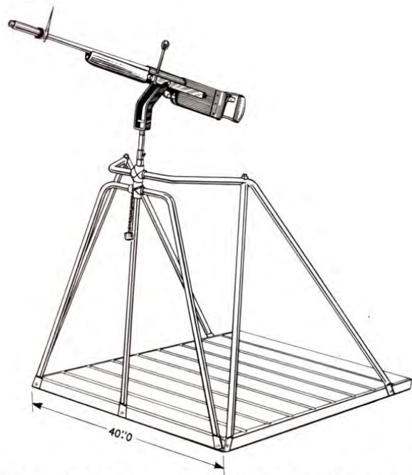
MOUNT, SHOTGUN, FLEXIBLE, COMPLETE WITH MODIFIED REMINGTON SPORTSMAN SHOTGUN
