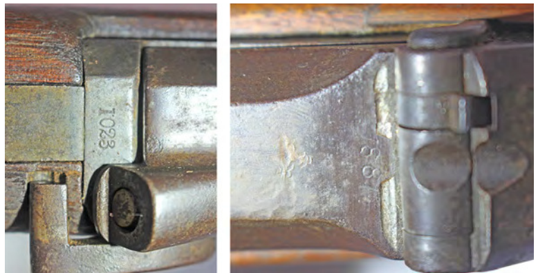
Figure 4. U.S. Springfield Model 1881 20-ga. Forager shotgun. The Springfield Armory built 1,376 Model 1881 26" barrel shotguns between 1881 and 1885. The serial numbers, receiver, 1881-dated breechblock and barrel are unique to this gun. As many earlier condemned parts were used in their assembly, the lock plate may or may not have the "1873" stamping and the hammer can have either coarse or fine knurling. The last use was in Alaska in 1906. The standard cartridge was a brass shotshell manufactured by the Frankford Arsenal. The shells were intended to be reloaded at the unit level in the field. The Model 1881 could be purchased by military personnel for $8.45. 7
