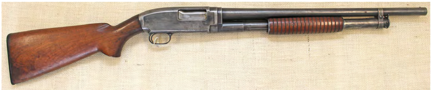
Figure 21. Winchester Model 12 riot gun serial number 976670. Most riot guns were manufactured prior to the trench guns. This early gun has a 41-dated barrel which had “MOD” struck out and “CYL” added when the factory shortened the barrel to 20 inches. As it does not have the usual “W.B.” final acceptance stamp, the stock is most likely an unmarked replacement to which someone added the postwar Defense Acceptance Stamp to make it look more authentic.
