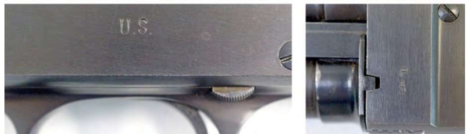
Figure 12. Stevens Model 520-30 Trench Gun, serial number 66756. Markings include "U.S." just above the trigger on the left side, "P" proof mark and "flaming bomb" on the left side of the receiver near the barrel and on the right and left sides of the barrel just forward of the receiver. These markings are smaller than those found on other World War II military shotguns. Note the purplish color of the bayonet adapter (shown next to a Model 12 bayonet adapter), a sure sign of a Stevens handguard/bayonet adapter.
