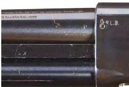
Figure 14. Ithaca Model 37 Trench Gun. The key items to check are the serial number which is found on the right front edge of the receiver, the barrel just forward of the receiver serial number and the stock (disassembly required), the blue finish, the handguard/bayonet adapter, and overall correct configuration. Ithaca made a limited number of Model 37 trench guns during the Vietnam war. These have serial numbers with an “S” prefix or are in the 900000 range. These were followed up by a later police/commercial variant with even higher serial numbers. All these later trench guns are parkerized. (photos courtesy of Rock Island Auction Co.)
