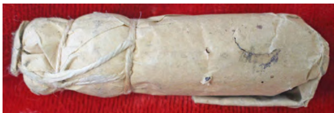
Figure 1. Buck and ball load. Found in .69 caliber with the usual configuration of three buckshot over a .69 caliber round ball. The buck and ball load was used, mostly in .69 caliber smoothbore percussion muskets, through the Civil War. A .58 caliber buck and ball load is shown. Unless otherwise noted, all photographs are by the author and are of items in his collection.
