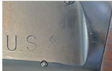
Figure 18. Military-marked Winchester Model 97 riot gun serial number 923463. This gun has a 1940 barrel date and the “U.S.” and ordnance “flaming bomb on the left side of the receiver. The stock is correctly “W.B.” inspected. This gun has a post-military refinish. Most collectors agree that only about one out of three or four Model 97 riot guns received military markings.
