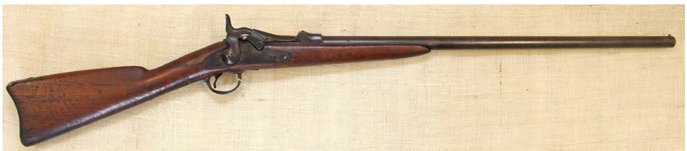
Figure 4. U.S. Springfield Model 1881 20-ga. Forager shotgun. The Springfield Armory built 1,376 Model 1881 26" barrel shotguns between 1881 and 1885. The serial numbers, receiver, 1881-dated breechblock and barrel are unique to this gun. As many earlier condemned parts were used in their assembly, the lock plate may or may not have the "1873" stamping and the hammer can have either coarse or fine knurling. The last use was in Alaska in 1906. The standard cartridge was a brass shotshell manufactured by the Frankford Arsenal. The shells were intended to be reloaded at the unit level in the field. The Model 1881 could be purchased by military personnel for $8.45. 7
