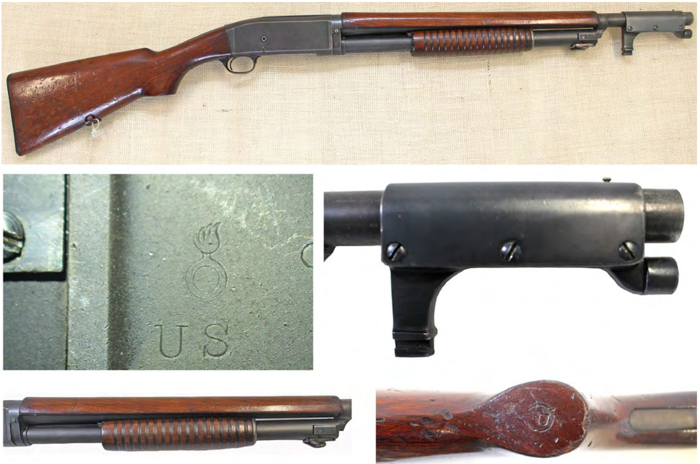
Figure 8. Remington Model 10 trench gun. The Model 10 trench gun is rarely seen today. The key features of this six-shot trench gun are its takedown, hammerless design, sling swivels, 23-inch barrel, wood handguard and separate bayonet adapter. Remington delivered 3,500 Model 10 trench guns during World War I. 15 Some were lost during World War I and post- World War I actions in Central America and the Caribbean islands, and many more were altered to riot gun configuration, but most were just worn out due to their poor mechanical design. Many were scrapped in the inter-war period. The Model 10 serial number range is from U117731 to U165566 with the majority being found between U160000 and U165000. 16 The serial number is found in two places, on the bottom of the receiver and on the left side of the barrel. On issued guns, these numbers are rarely matching. The illustrated gun bears serial number U164493 on the receiver and U159612 on the barrel. The left side of the receiver is stamped with the ordnance “flaming bomb” over “US”. The bottom of the pistol grip on this gun has the circle “P” inspection stamp which is a sign of later depot maintenance. There’s a good chance that this gun saw service in World War II as well as World War I.
