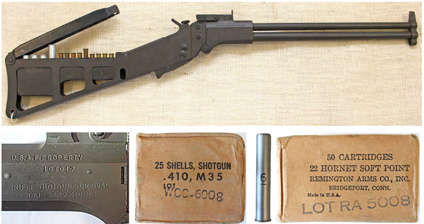
Figure 32. Ithaca M6 Aircrew Survival Weapon. The M6 was adopted by the Air Force in March, 1951. It is an over/under .22 Hornet/.410-ga. combination firearm. It was designated “Cal. .22/.410 Gage Survival Rifle-Shotgun M6”. It folds to fit the survival kit in the seat pack of ejection seats. 47,48 It is a much better firearm than the “piece of junk” .22 Hornet H&R M4 rifle it replaced. 49 Note: because of its 14-inch barrels, the M6 is an NFA item.
