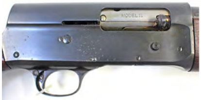
Figure 17. Remington Model 11 riot gun serial number 491019. This can be called the standard World War II configuration as it has no game scene on the receiver and plain stocks. The matching barrel date is July 1943.
