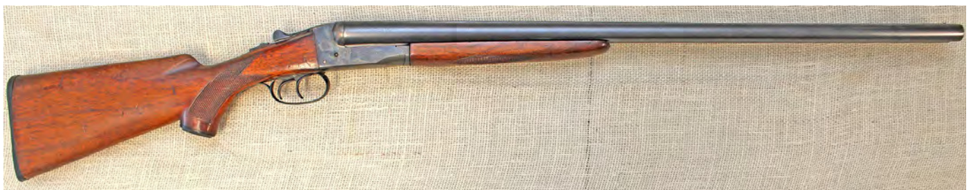
Figure 25. Stevens Model 530 double barrel 12-ga. training shotgun. This is an example of one of many training shotguns that were bought early in World War II. The Model 530 is not serial numbered. This gun has 28-inch barrels. The receiver is marked with the “U.S.” and ordnance “flaming bomb.” Note the commercial finish and game scene.
