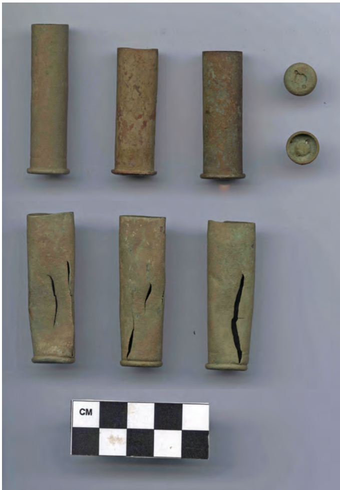
Figure 4. These .45-55-caliber cartridge cases split when fired in a larger caliber firearm. They may represent army cartridges salvaged from dead soldiers and repurposed and fired in warrior used Sharps and Springfield .50-70-caliber firearms (NPS image).
