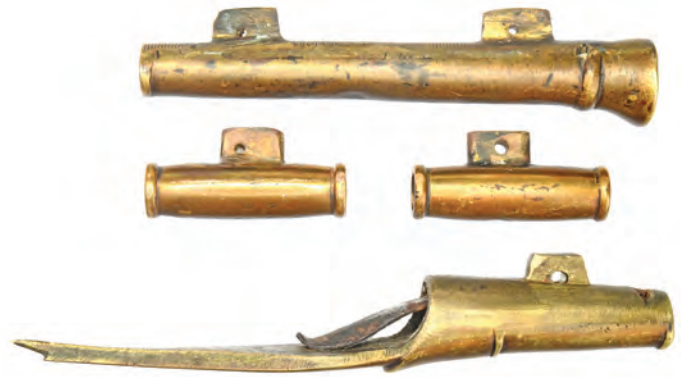
Figure 16. The brass rammer pipes of the subject Dragoon's Carbine. Note the spoon-shaped rammer retention-spring on the tail piece (bottom).
