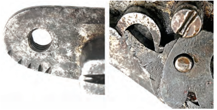
Figure 7. Assembly marks on the front inner edge of the lock-plate (left) and tumbler (right).
