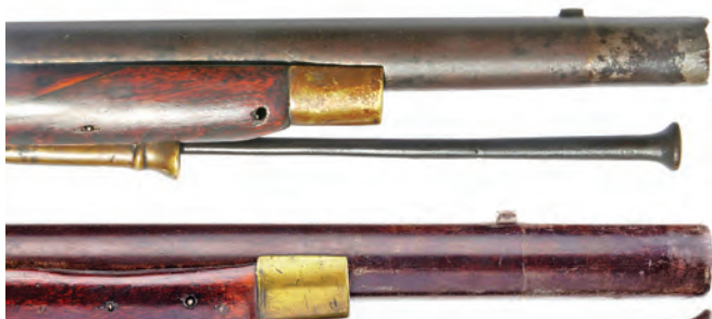
Figure 15. The muzzle end of the Dragoon's Carbine with its iron rammer and cast-brass nose-cap (top), Short Land Pattern Musket with its iron rammer and cast-brass nose-cap (middle, photo courtesy of Morphy Auctions, www.morphyauctions.com ) and 1760 Light Infantry Carbine with its wood rammer and folded-brass nose-cap (bottom; photo courtesy of Morphy Auctions, www.morphyauctions.com ).
