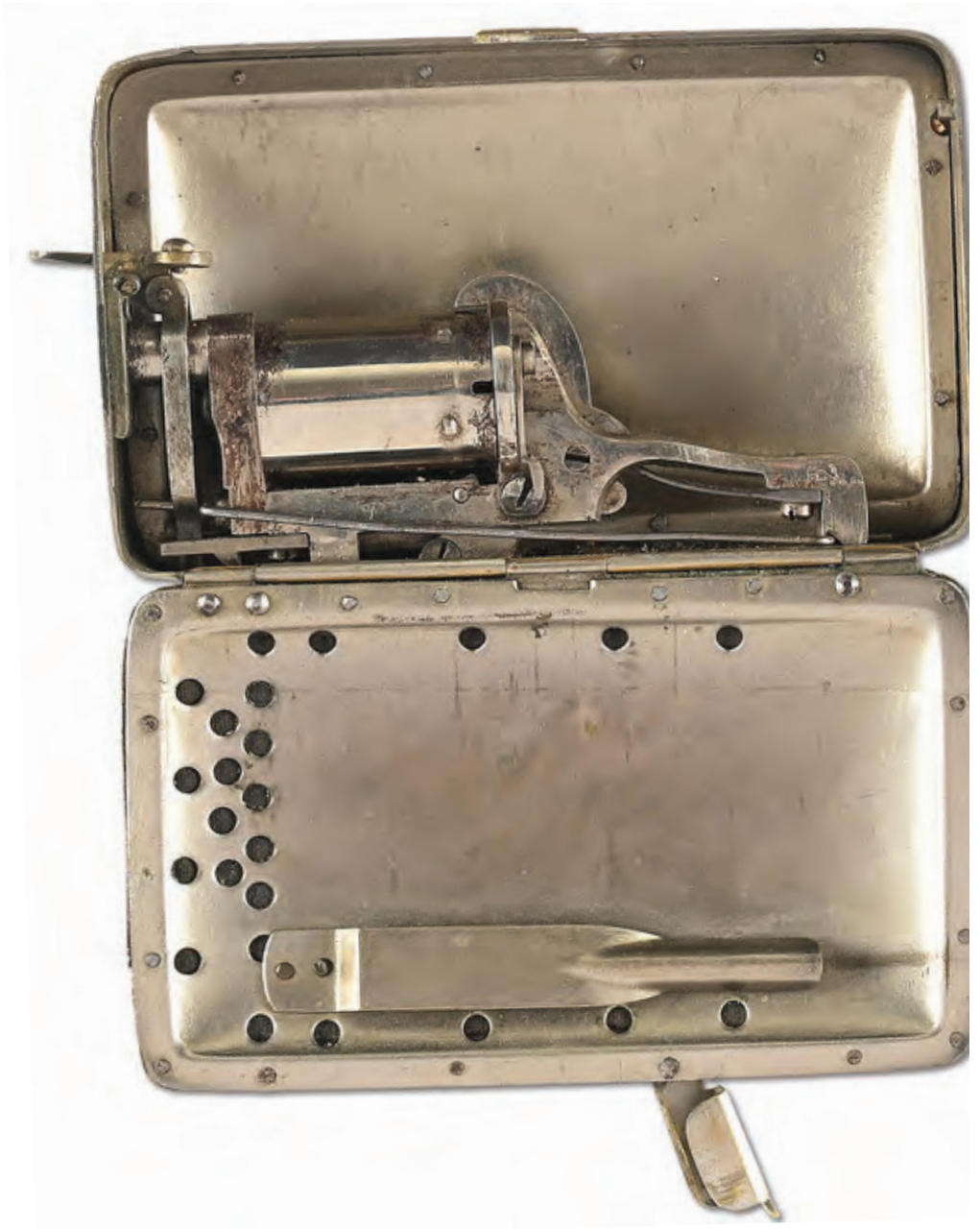
Figure 3. Frankenau Purse Revolver with gun compartment open showing the 5mm pinfire revolver. Note that the hinged firing port over the gun muzzle is open. Note the empty ejector rod holder. Photo courtesy of Morphy Auctions, Denver, PA.
