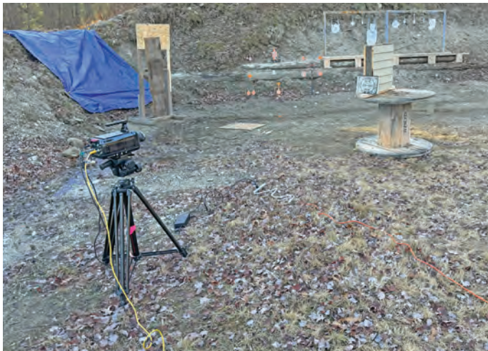
Figure 3. The Fastec high-speed camera being calibrated for a shot at a wall panel.
