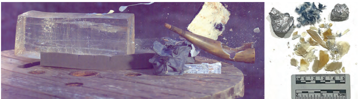
Figure 11. High-speed video of the ball passing through the horn. Right: The split ball, cloth fragments and horn shards removed from the wound track in the ballistic gelatin. The cloth and horn fragments weighed 3.1 grams.
