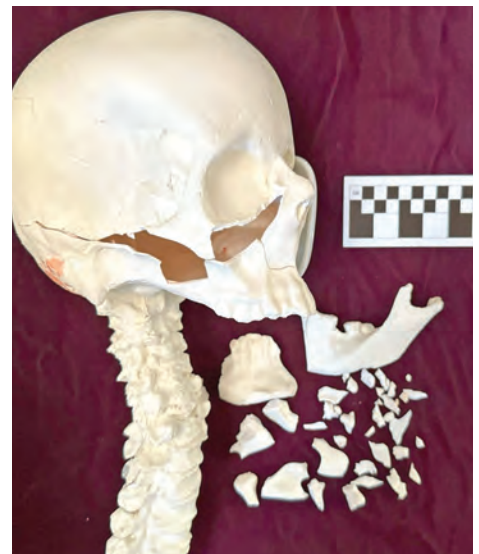
Figure 15. Top left: The ball created a splash effect as it enters the gelatin bust. Center top: the ball exiting the ballistic gelatin bust. Note the massive cavitation effect on the neck and lower jaw area. Top right: the bust after the immediate cavitation ceased. The red areas are synthetic blood oozing from the fractured skull. Bottom: The synthetic skull and bone fragments removed from the gelatin bust.
