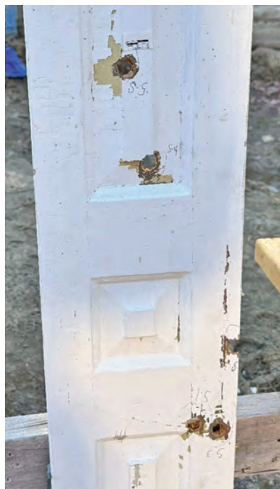
Figure 9. Five bullet strikes in a salvaged indoor window shutter that replicates bullet strikes observed in surviving shutters in the Arlington Historical Society collection. Right: Exit holes showing the wood splintering after the ball passed through the shutter.
