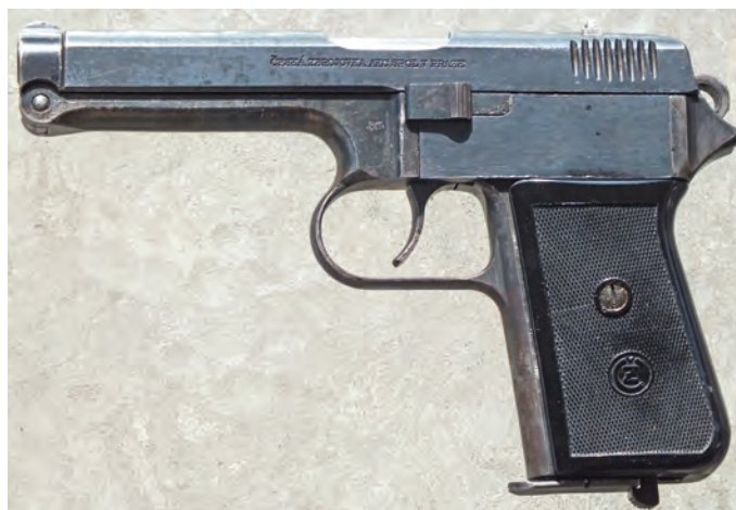
Figure 14. Waffen SS vz-38 with serrated hammers used on the safety-equipped pistols.
