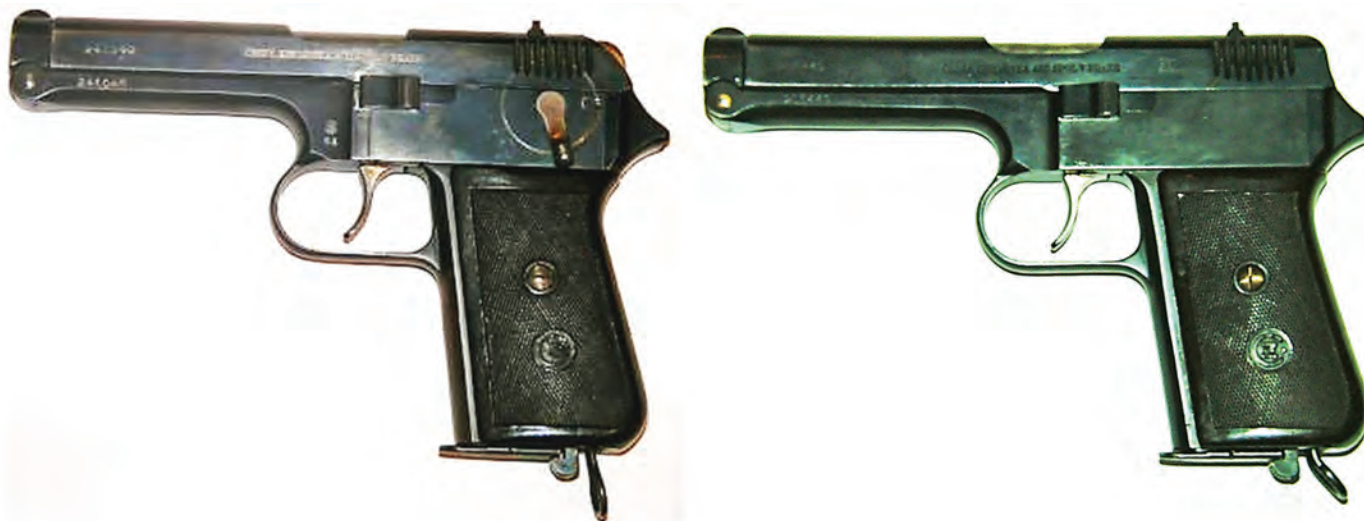
Figure 13. Bulgarian vz38, note safety below the rear sight (left) and vz-38 from Finland with a SA stamp, indicating Finnish Army issue.
