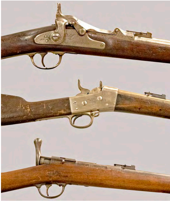
Figure 29. The receivers of the Springfield trapdoor, Remington rolling block, and Ward-Burton bolt action carbines (top to bottom; photo by Amy Cortee-Cox).
