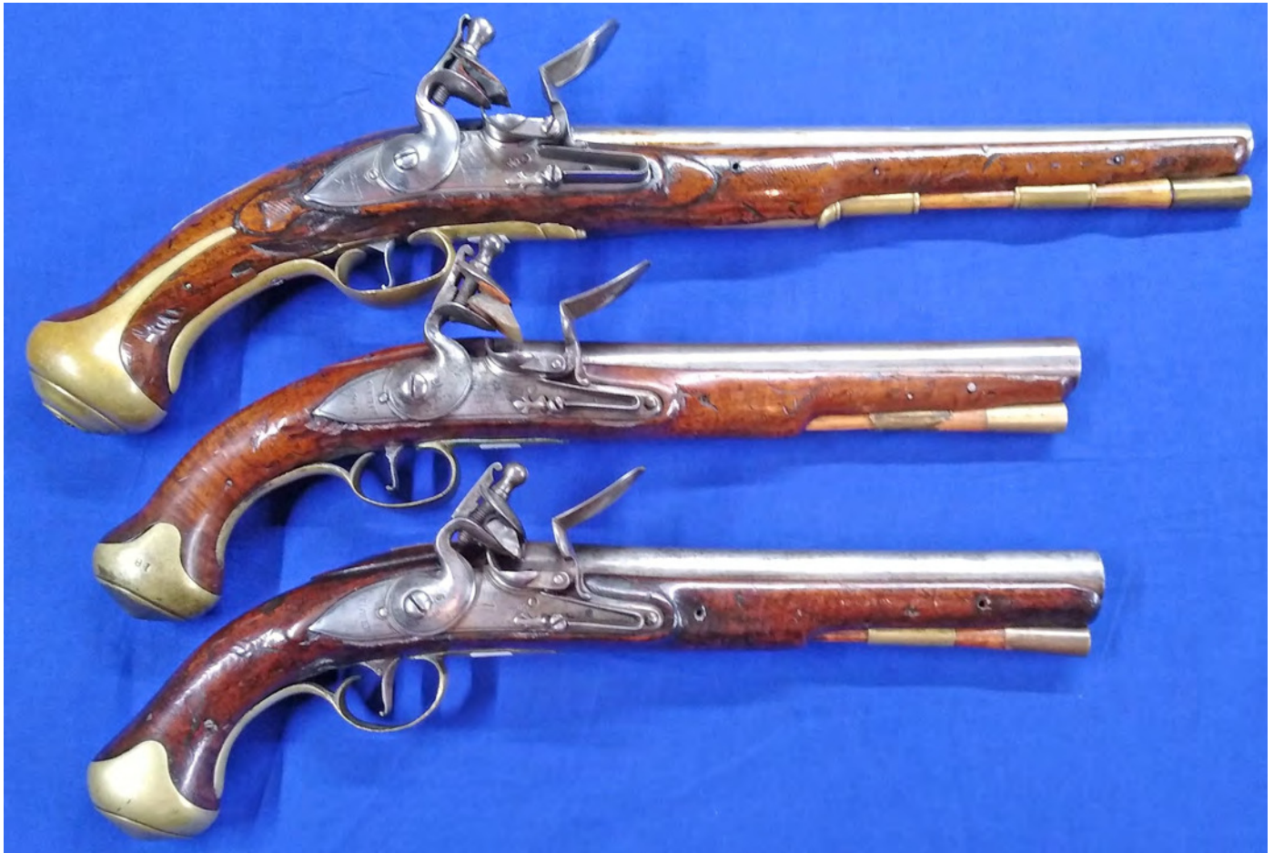
Figure 1. Pattern 1738 Dragoon pistol (top) over a Pattern 1759 (middle) and Pattern 1759/76 (lower).
