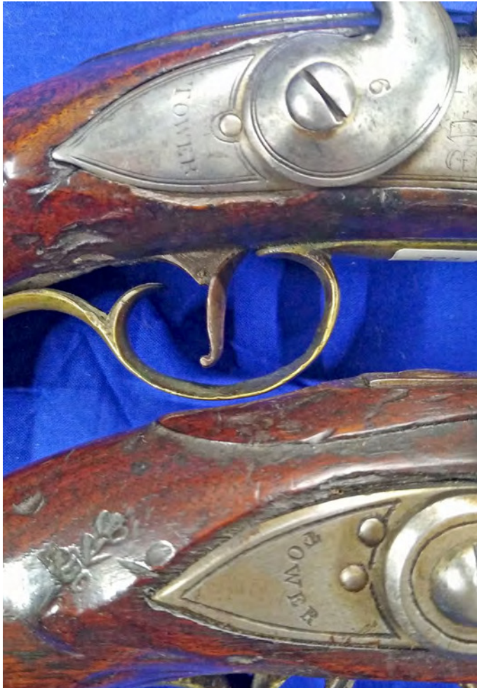
Figure 9. Pattern 1759 Lock compared to Pattern 1777 Locks with two screws visible to the left of the cock.
