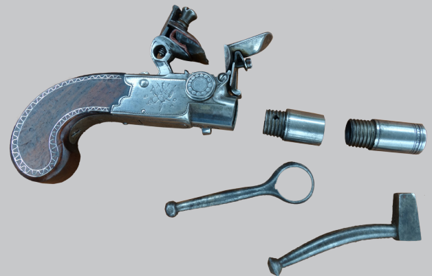
Figure 14 - In a standard turn-off pistol, the threads are part of the breech. Here, they're part of the barrel sections. Note the hole in the rear threads which lines up with the front touch hole.
