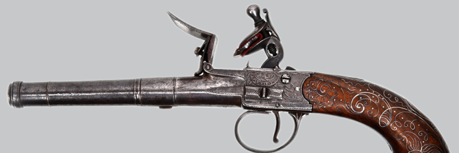
Figure 8 - The Waters pistol. Note the relatively long breech and pan area; the pan selector; and the lug for the barrel turn-off key.
