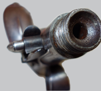
Figure 2 - The breech opening of a conventional turn-off pistol ( also by Louis Barbar). The cavity is filled with powder, and the base of the ball rests on the concave opening. The barrel will screw on tightly over the ball.
