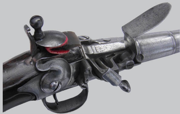
Figure - 6 The pan in the midst of rotating, the next step. The lever is more clearly visible.
