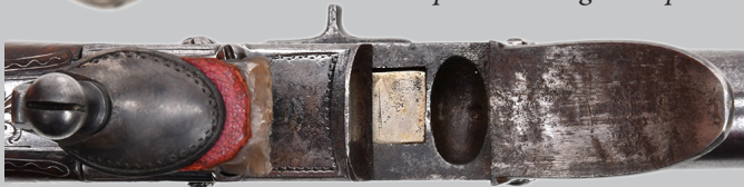
Figure 10 - The Waters' oval front pan for the front ( first) shot is ready. The rear pan is covered. Note that the pan selector has been moved forward.
