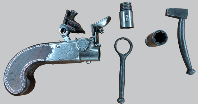
Figure 13 - Both barrel sections off. Note the front section is notched for a muzzle key. Both types of keys are shown
