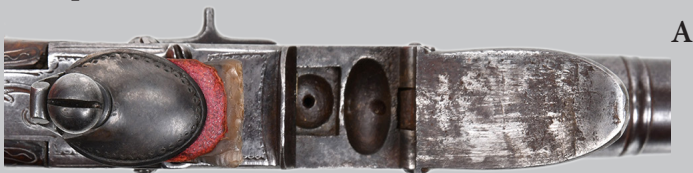
Figure 11 - The Waters' pan selector has been moved rearward. The square-bordered circular rear pan is now revealed, ready for the rear (second) shot.
