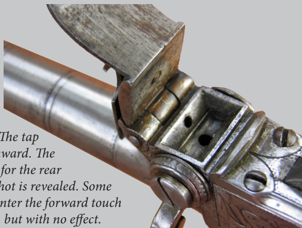
Figure 17 - The tap lever rearward. Only the touch hole for the front ( first) shot is revealed.
