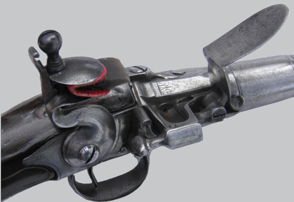
Figure 5 - The pan in position for the second ( rear) shot, with its touch hole in standard position. Priming this pan would be the first step.
