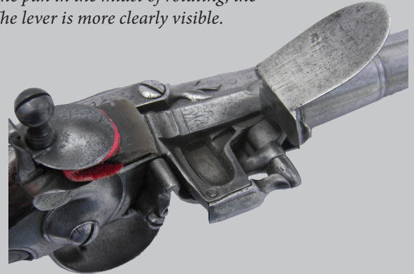
Figure 7 - The pan in position for the first ( front) shot . The small trough leads forward to the front touch hole. Priming this pan would be the next step. One could then fire the first shot
