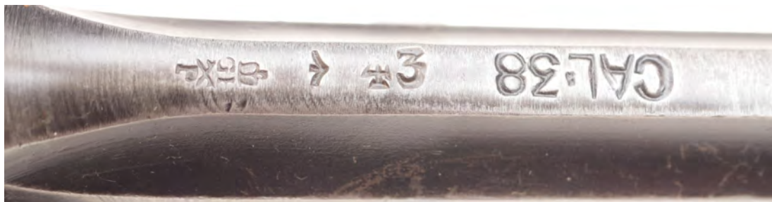
Figure 9. Another example of a military proof on the barrel of an Enfield No.2 .380 revolver.
