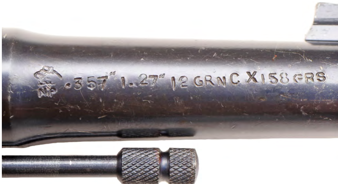
Figure 6. The barrel of a British Purchasing Commission Colt New Service in .357 Magnum bearing London 1954 proof marks. Noteworthy are the lack of a view mark and indications of the nitro cellulose (NC) propellant proving charge and bullet weight.
