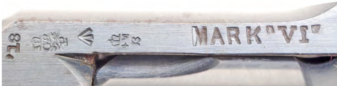
Figure 8. The military barrel proof on the topstrap of a .455" Webley Mk. VI (c. 1918). Since Webley & Scott Ltd. was a civilian arms manufacturer, a RSAF, in this case BSA, was used to provide Government inspection.
