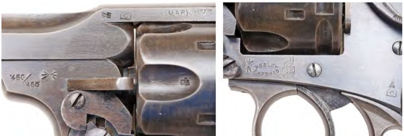
Figure 13. Two views of a WWI Webley & Scott Mk. V bearing both the commercial caliber designation and Birmingham proof and view marks. It was then used as a service weapon, then subsequently sold out of service Sales Permit mark is also in evidence. Note both the [C] and the Government “B” (for the Sparkbrook RSAF) inspector’s mark.
