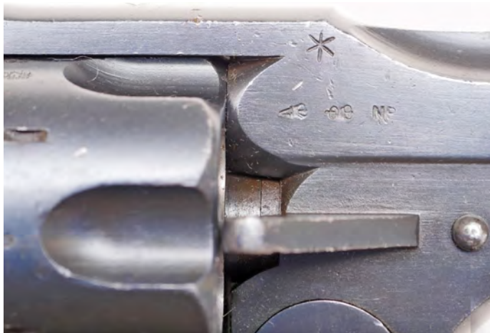
Figure 17. While unlikely, the * might be misconstrued as a small version of the Sale Permit mark. Alternatively, various upgrades or modifications to British military small arms are designated by the addition of a*, referred to as a “star” in the official nomenclature (e.g. SMLE Mk. III* or No. 2 Mk. I,** etc.). However, if the * is over a chamber or forcing cone, on the Nock’s form, or on the barrel, it simply means rust or wear.
