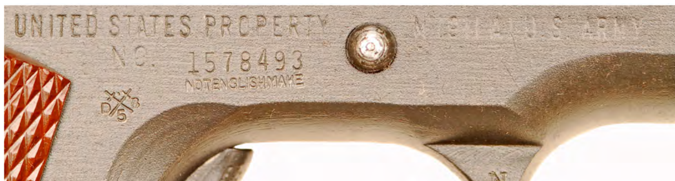
Figure 20. As an example of these “Secret” or “Private” View marks, here on an ex-Lend-Lease Remington Rand M1911A1, just in front of the grip panel, surrounding the crossed scepters are: DB = 1953 year of proof and 5 = Inspector’s designation.
