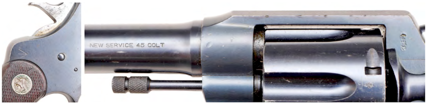
Figure 22. Unlike the Colt Single-Action Army, due to differences in cylinder dimensions, the New Service in .45 Colt could chamber the British .455" Mk. II service cartridge. This BPC revolver displays crudely, but yet officially, the Broad Arrow of military acceptance.
