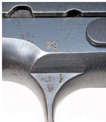
Figure 10. Enfield inspection and proof mark ensemble on a pre-1918 WWI era .455" Colt Government Model [W62020]:
