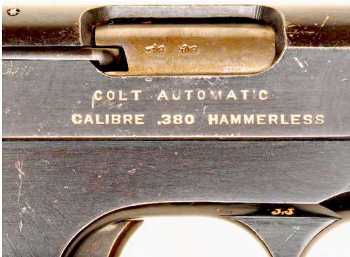
Figure 14. A "JJ" marked London Armoury Co. retailed Colt M1908 Hammerless .380 (27462) manufactured in late 1915. Note also the London proof and view marks on the barrel.
