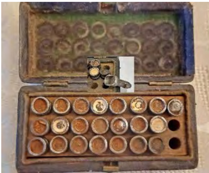
Figure 16. The cased set of hammer noses. Note various residual bits of patch. The small rectangular image that includes the copper cap noses is a superimposition.
