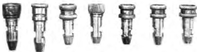
Figure 8. A variety of mature patch lock hammer noses. The mouth is now wider and the end is closed. The indentations near the tail remain, allowing the hammer spring to keep them in place. See Gooding 1 for image source.
