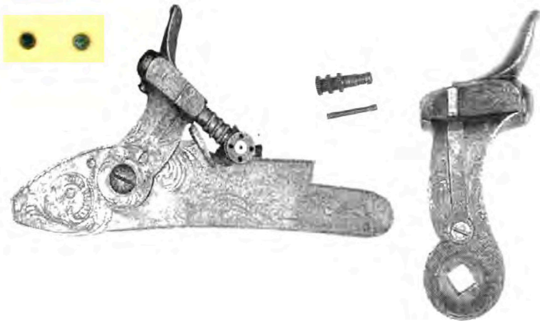
Figure 6. Joseph Manton's patent pellet lock ignition system. From the right, the hammer; the hammer nose; the firing pin; the lockplate showing the nose in place and the anvil; two Manton detonating pellets. See Gooding 1 for image source, arranged by the author.
