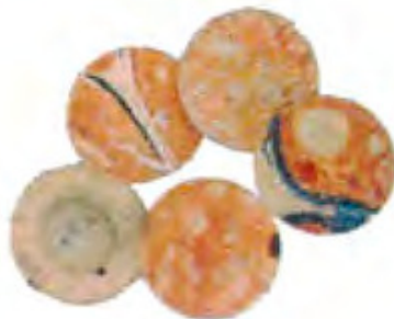
Figure 5. A group of Hall's patches. You can see the central blob of fulminate. See Gooding1 for image source.
