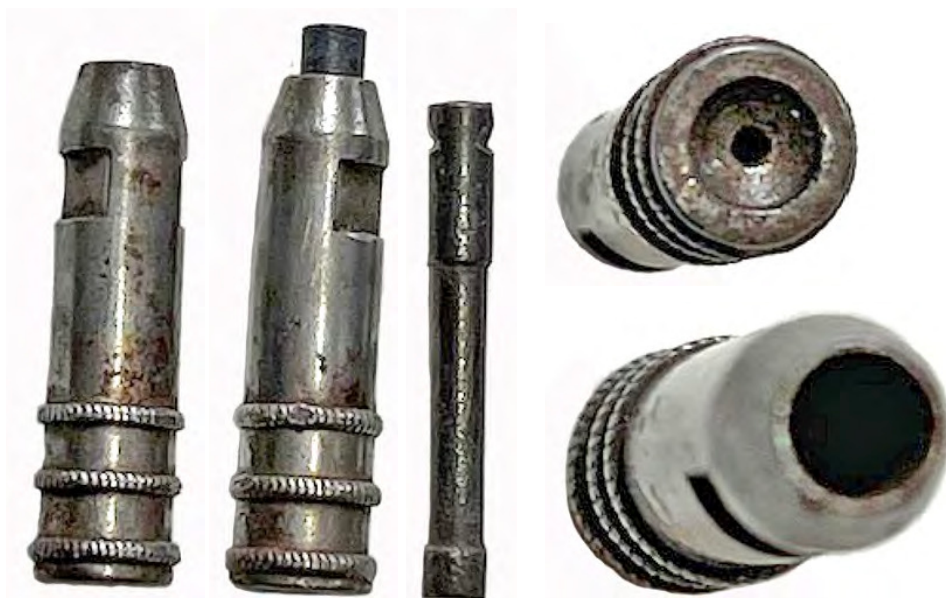
Figure 7. From right, the hammer nose without the firing pin, rear end (note the indentation for the spring); the hammer nose front end, with the ignition flame passage; the firing pin; the hammer nose on its side, with the firing pin inserted; the hammer nose on its side, without the firing pin. Photos by and collection of Will Adye-White.
