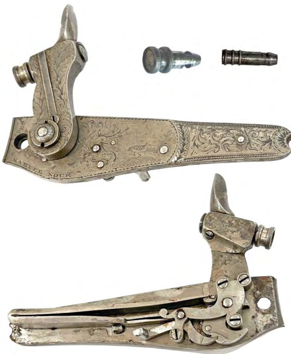
Figure 14. The left-hand lock. I have added a close-up view of the hammer nose showing ribbing for gripping, the indentation to engage the hammer spring, and some residual bits of patch. For comparison, the Manton patent nose. Photos by Jiri Velharticky.
